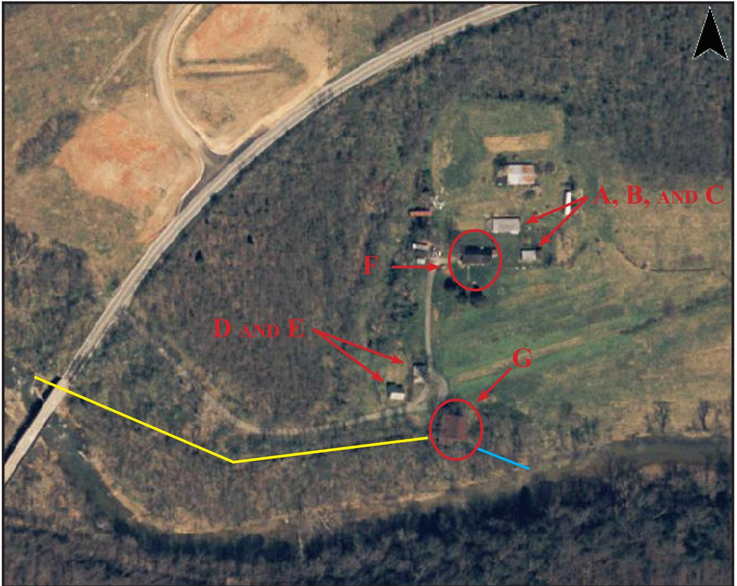
Figure 36: Aerial photograph, 2008. The yellow line in the head race carrying water from Catoctin Creek to the mill (G) circled in red. The blue line is the tail race that conveys the exhausted water from the mill back to the creek. Two outbuildings (D and E) are in proximity to the mill (G) and the dwelling (F) is to the north. Northeast of the dwelling are outbuildings A, B, and C (Map of courtesy of Frederick County GIS).
