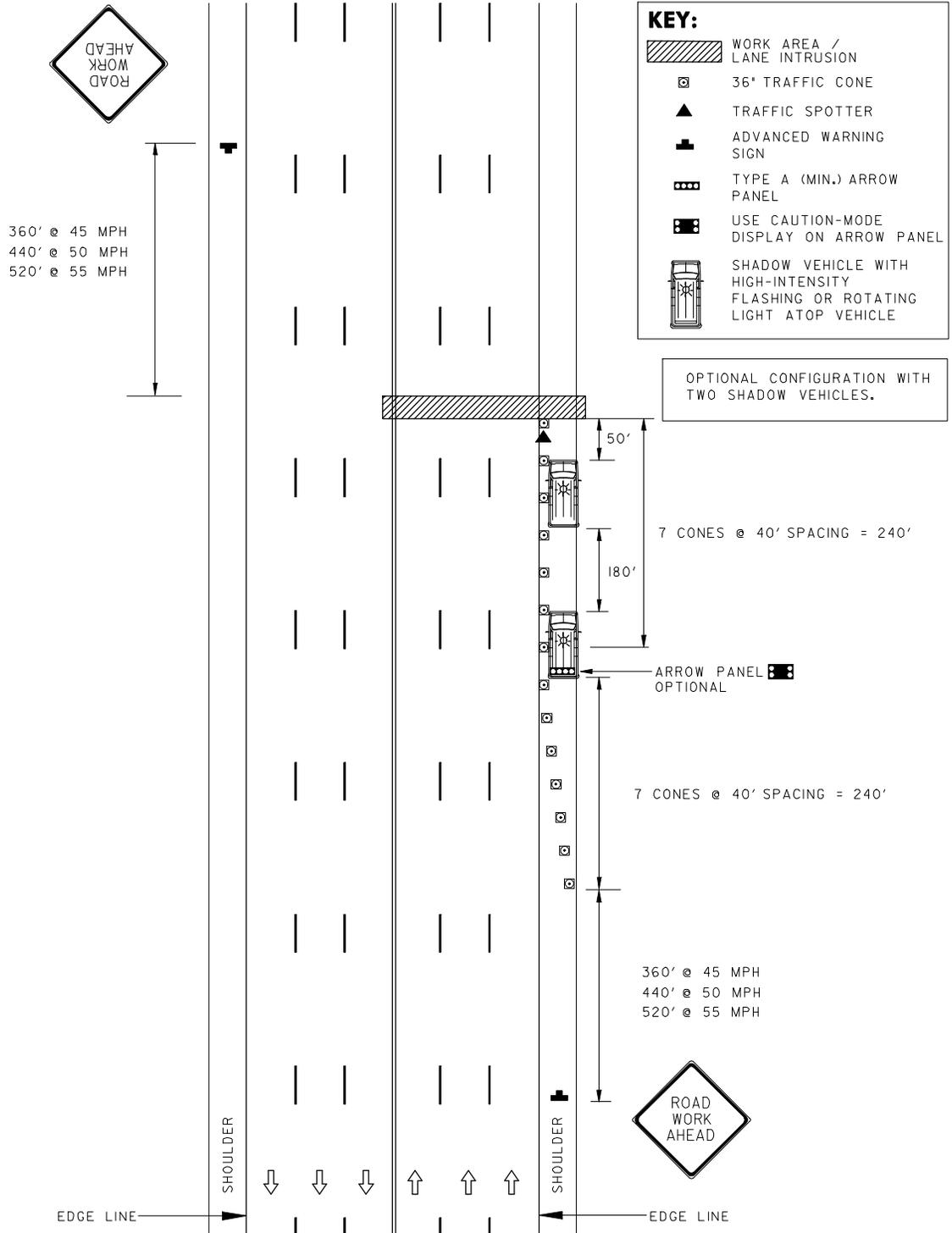
CONES SPACED AT 40' TYP.
