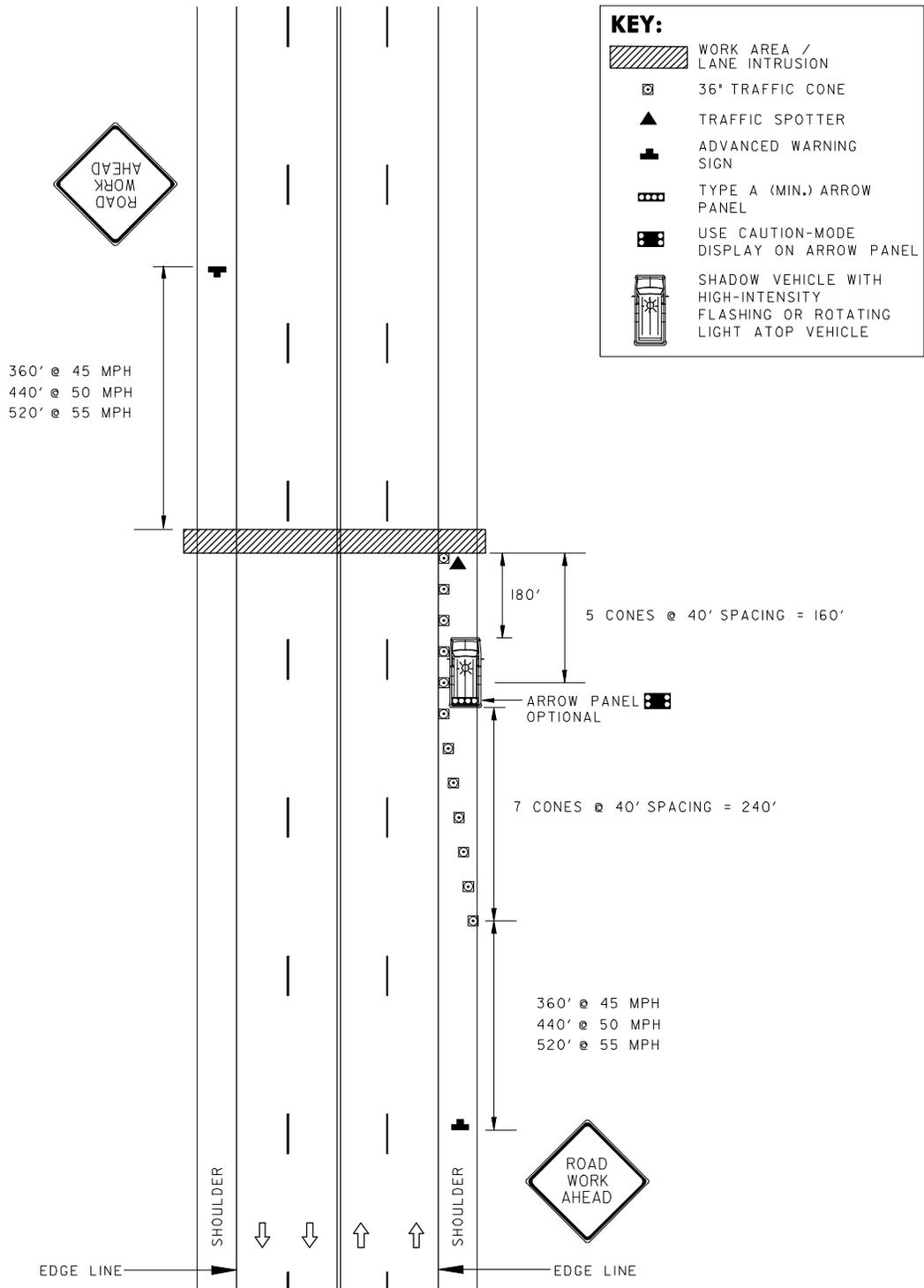
CONES SPACED AT 40' TYP.
