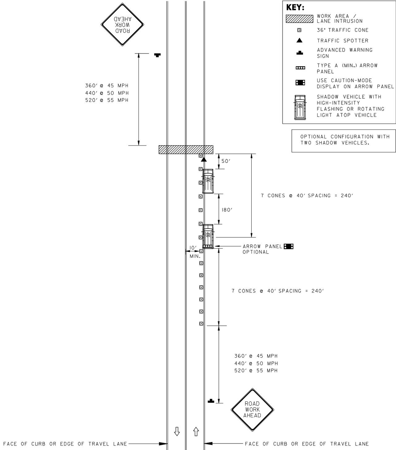
CONES SPACED AT 40' TYP.
