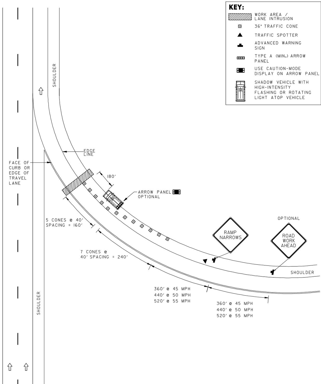
CONES SPACED AT 40' TYP.
