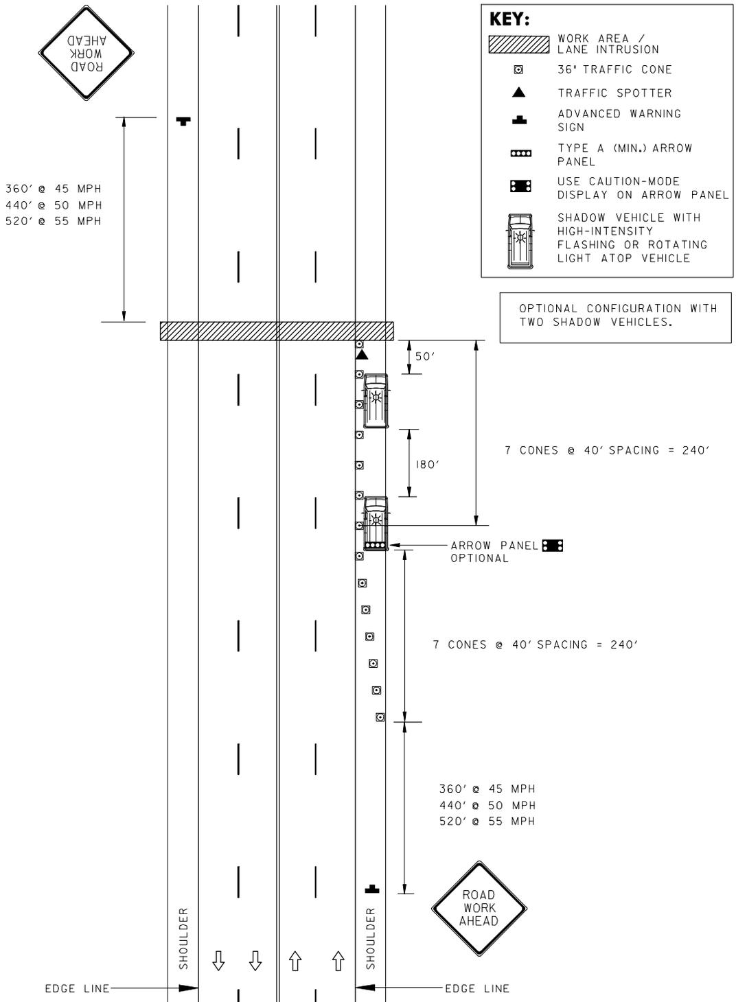
CONES SPACED AT 40' TYP.
