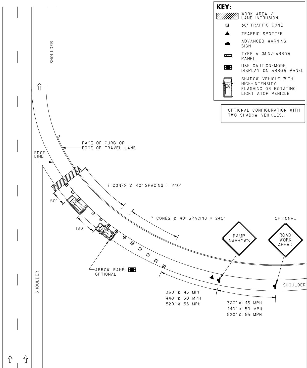
CONES SPACED AT 40' TYP.
