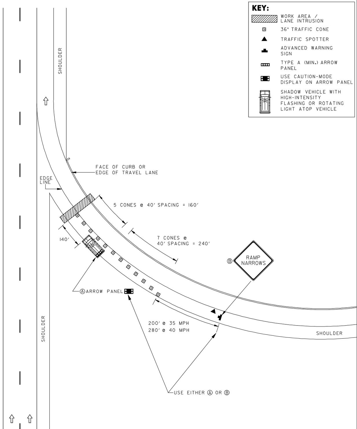
CONES SPACED AT 40' TYP.
