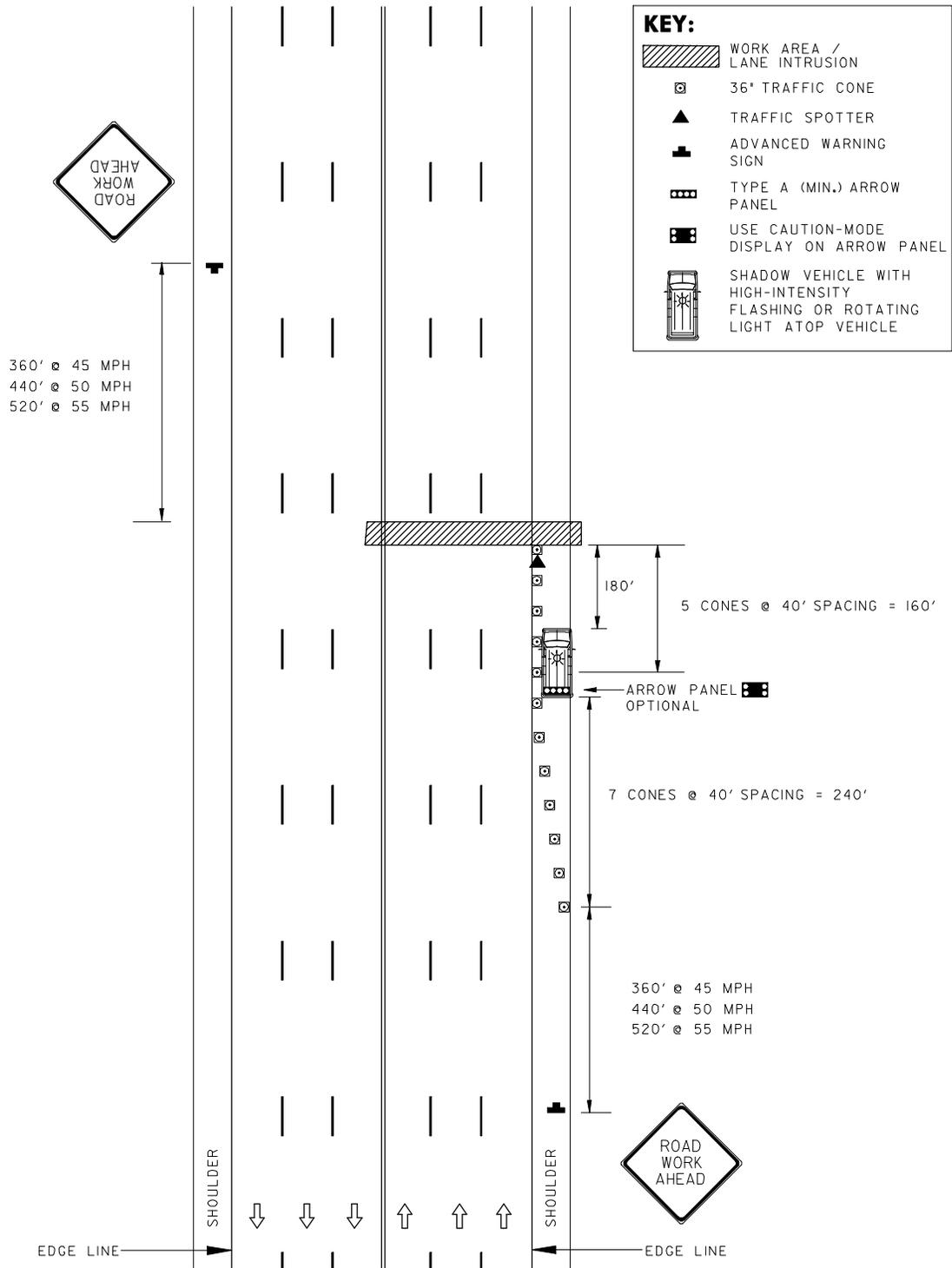
CONES SPACED AT 40' TYP.
