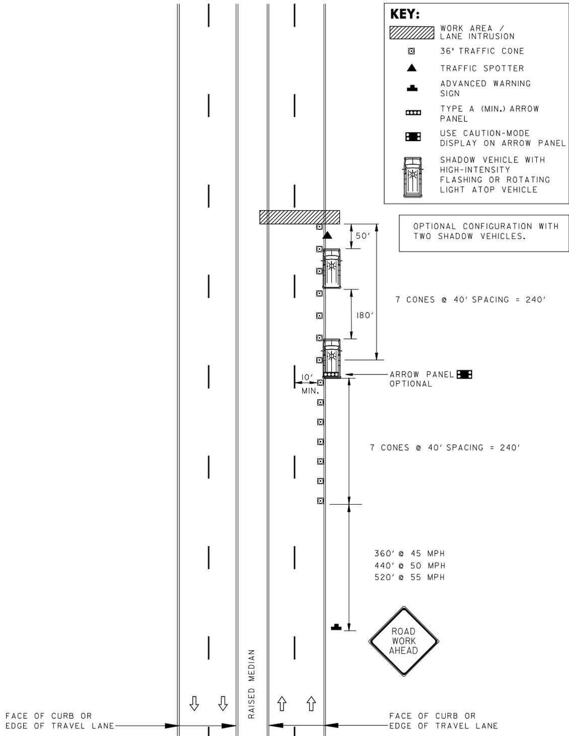
CONES SPACED AT 40' TYP.
