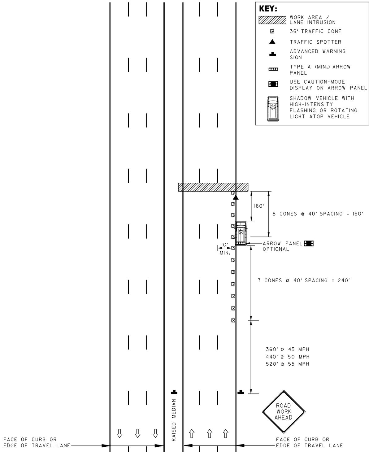
CONES SPACED AT 40' TYP.
