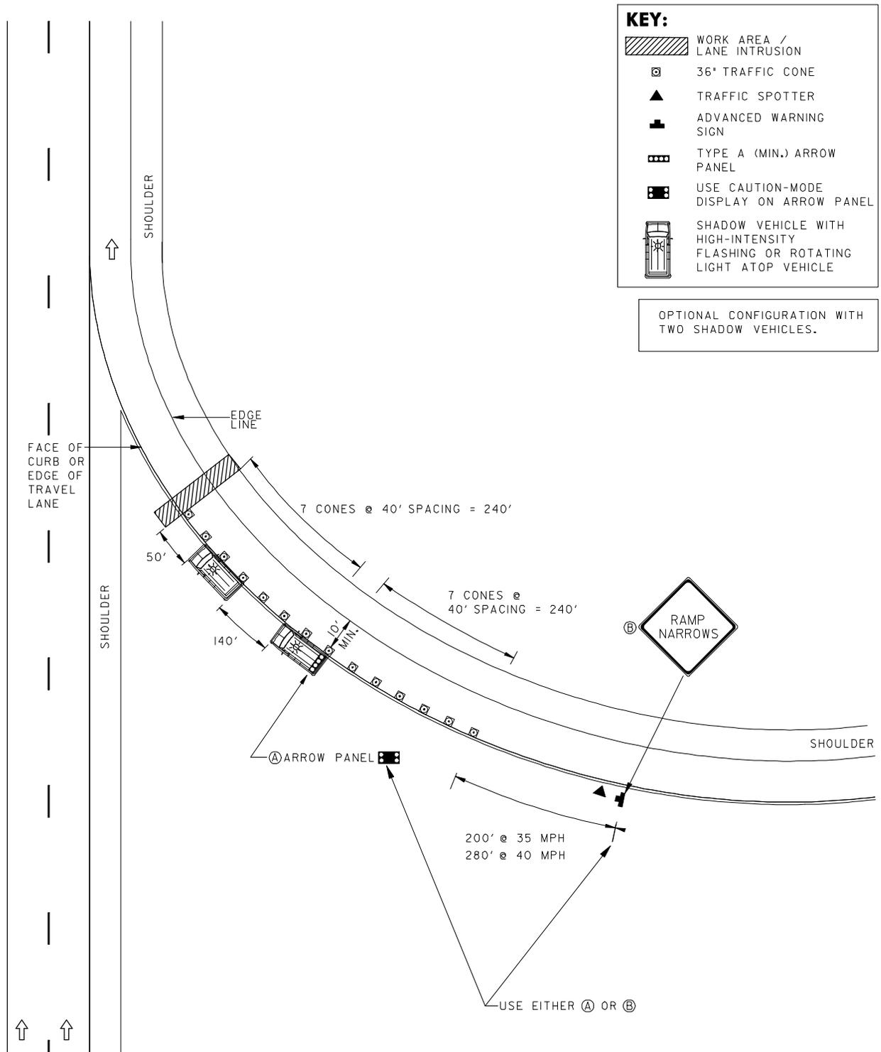
CONES SPACED AT 40' TYP.
