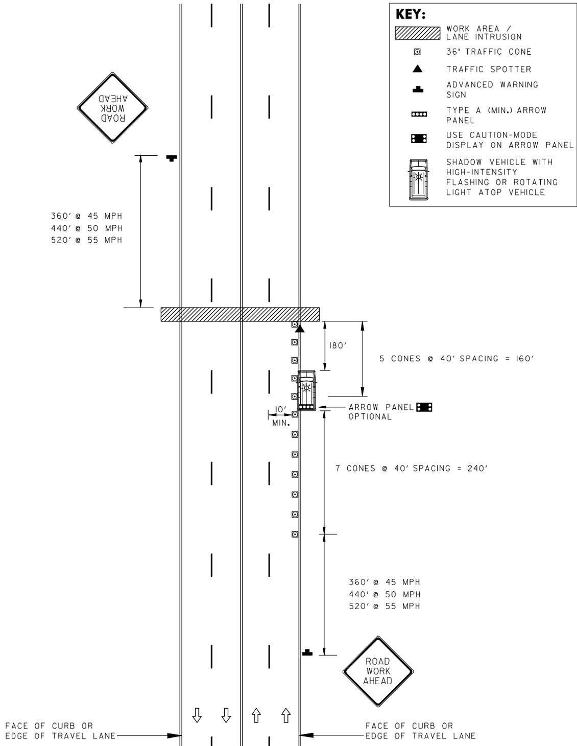
CONES SPACED AT 40' TYP.
