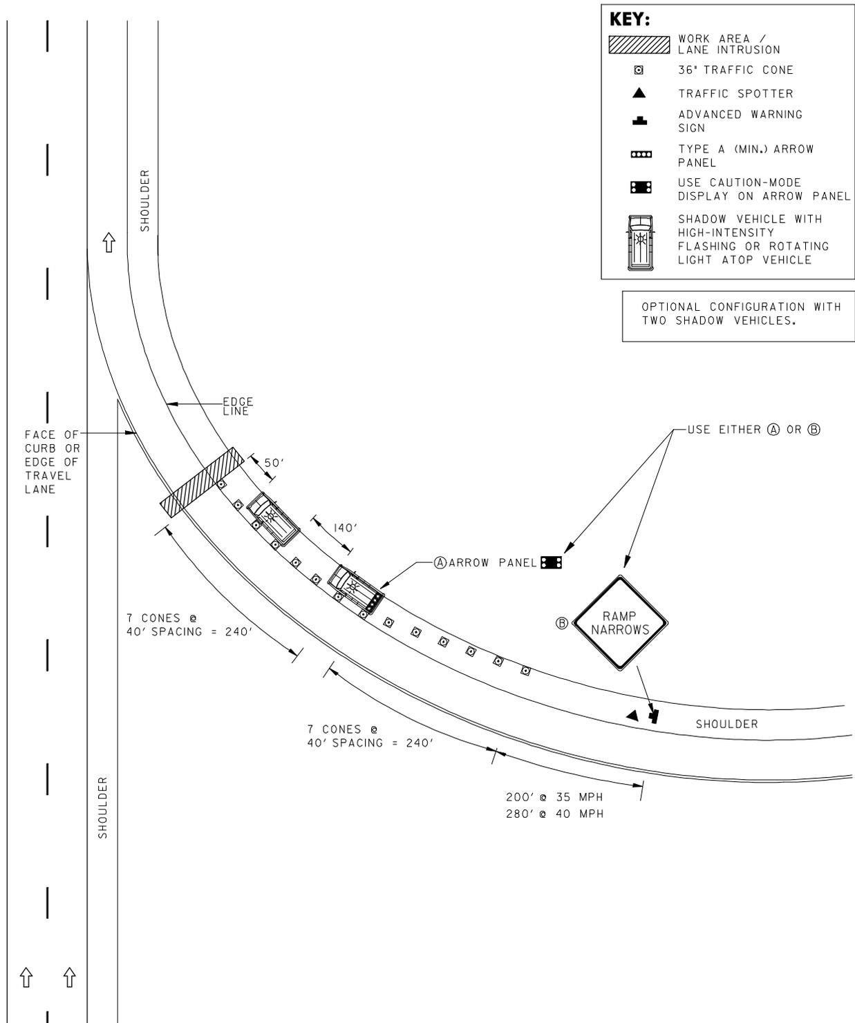
CONES SPACED AT 40' TYP.
