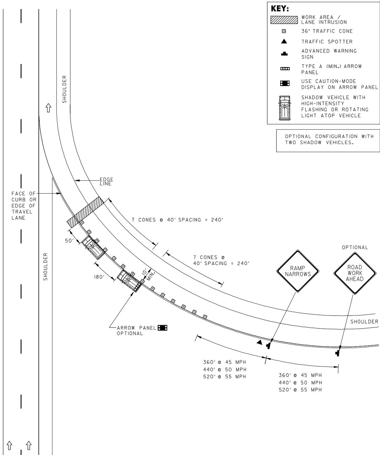
CONES SPACED AT 40' TYP.
