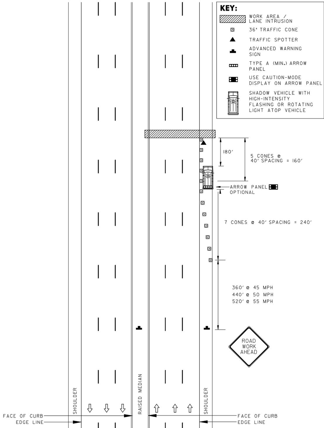
CONES SPACED AT 40' TYP.
