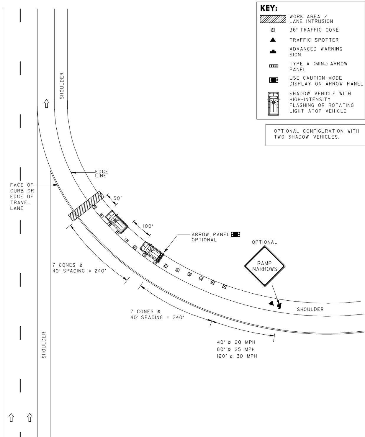
CONES SPACED AT 40' TYP.
