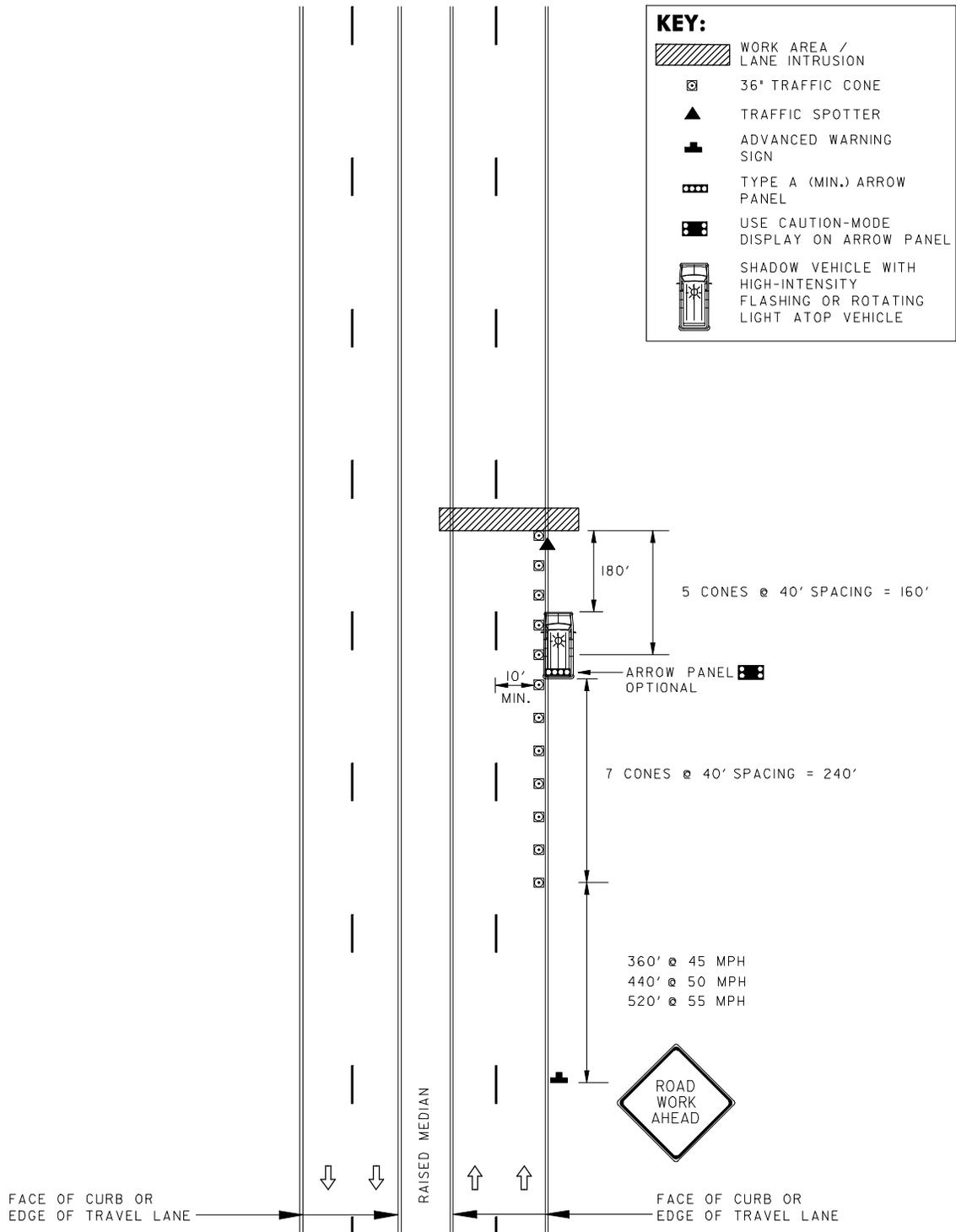
CONES SPACED AT 40' TYP.
