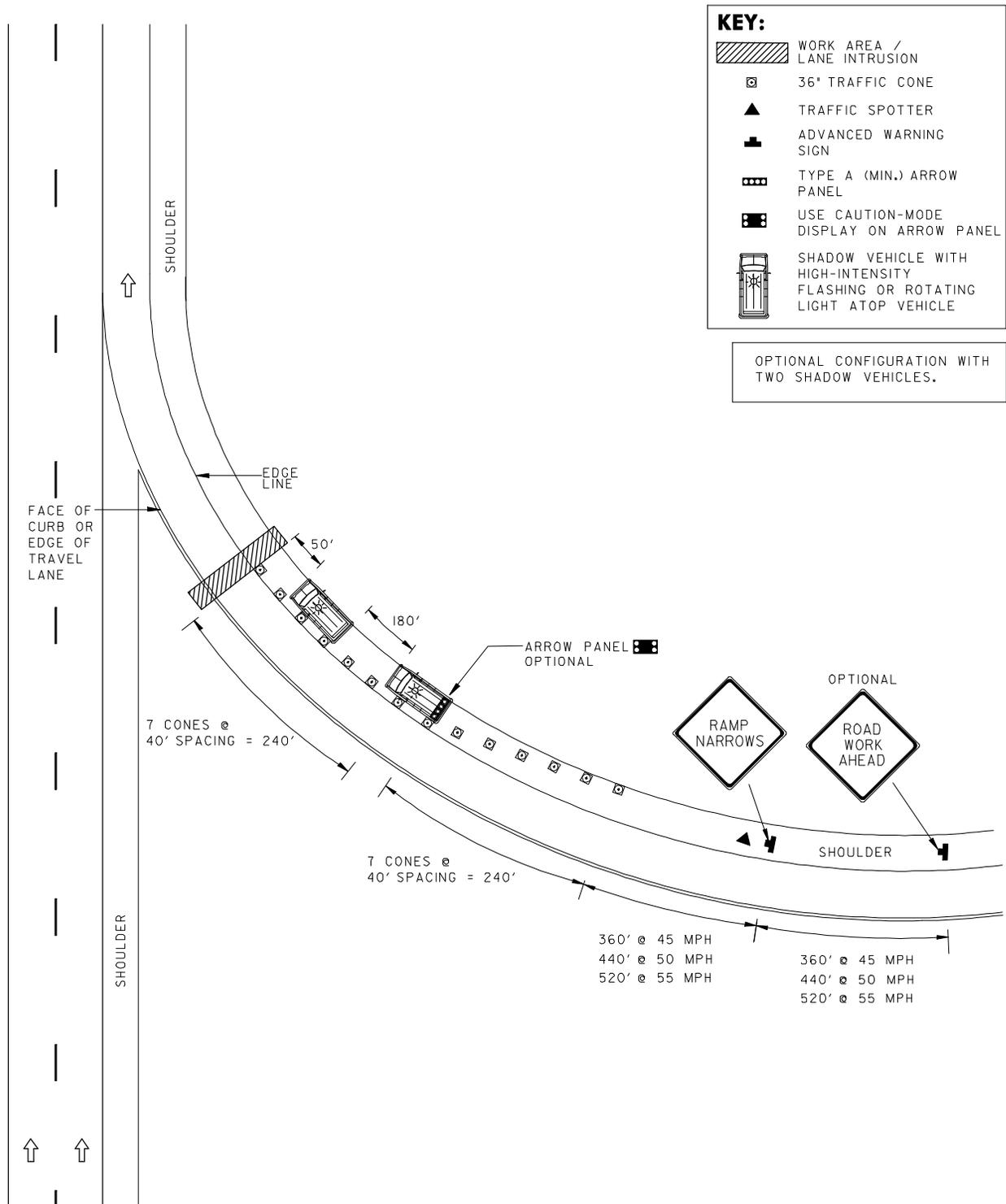
CONES SPACED AT 40' TYP.
