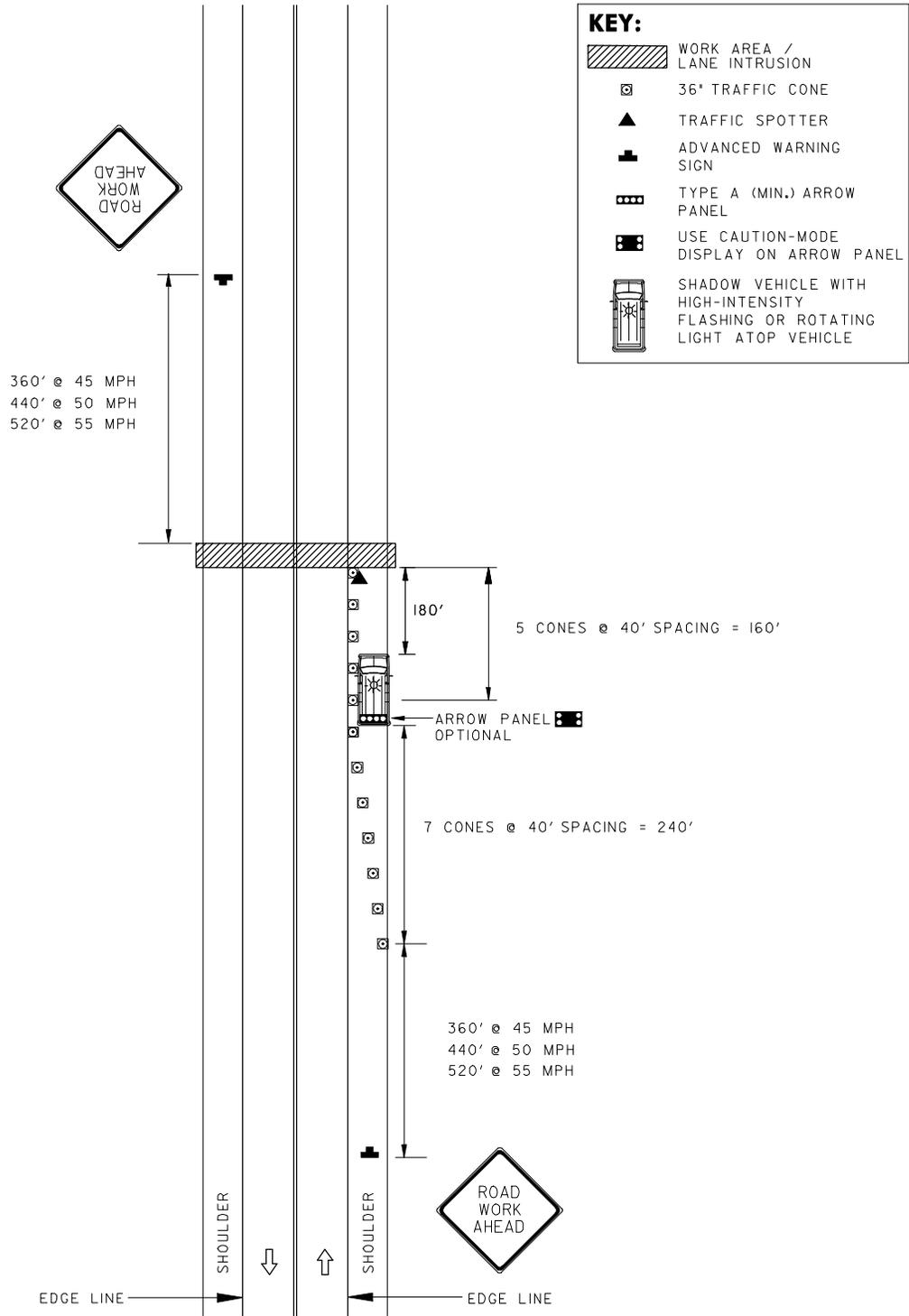
CONES SPACED AT 40' TYP.
