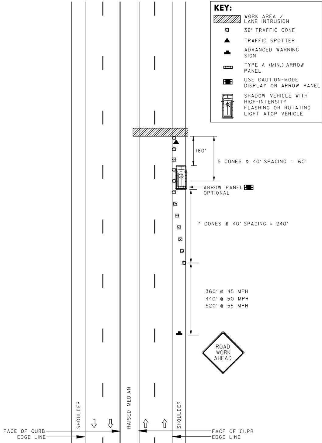
CONES SPACED AT 40' TYP.
