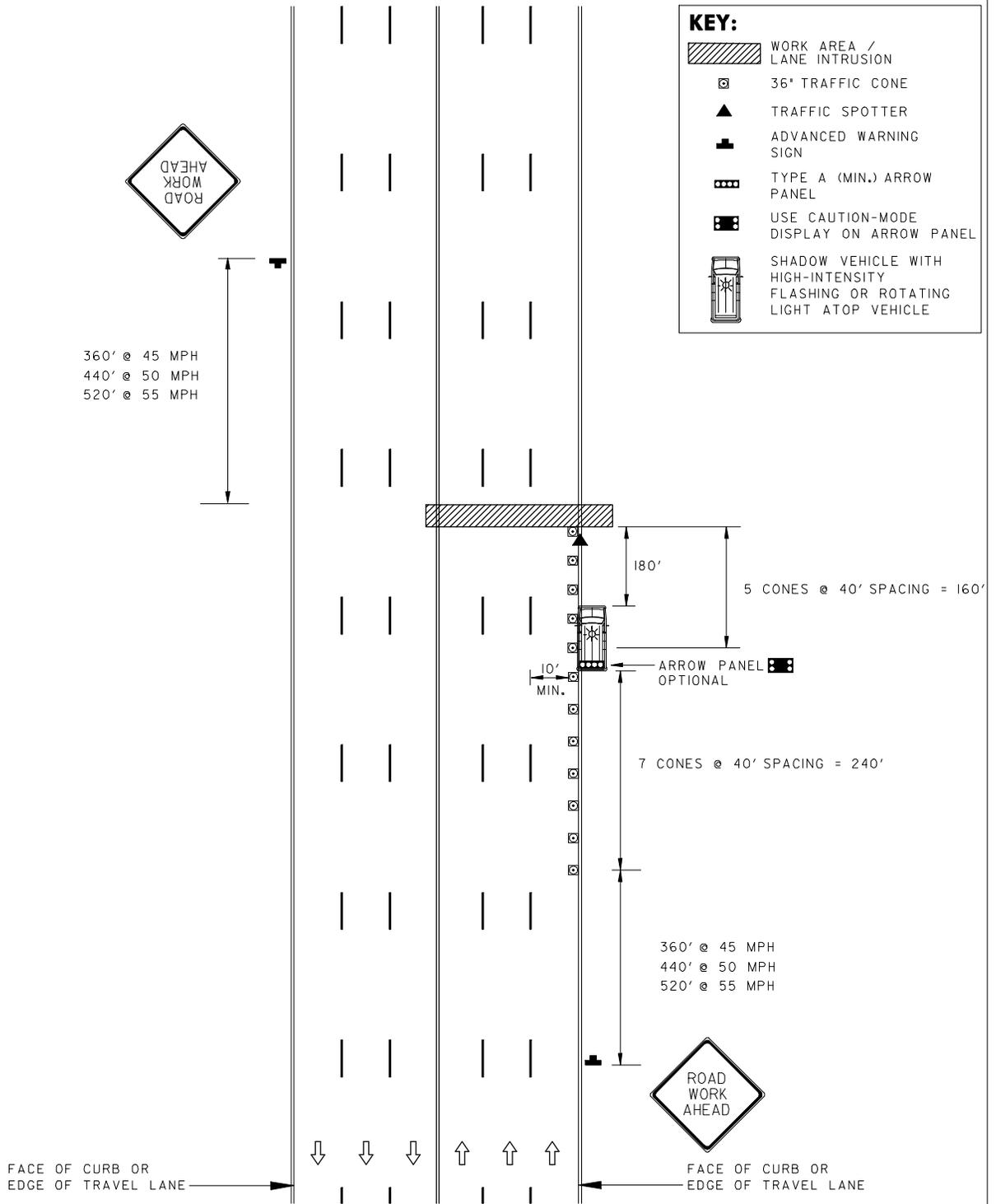
CONES SPACED AT 40' TYP.
