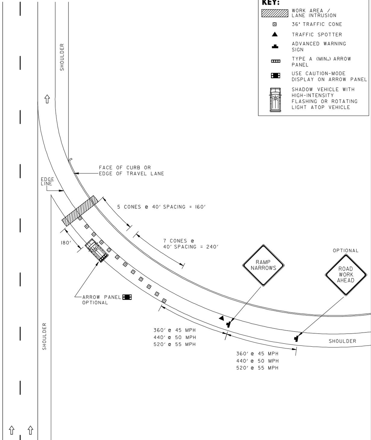
CONES SPACED AT 40' TYP.
