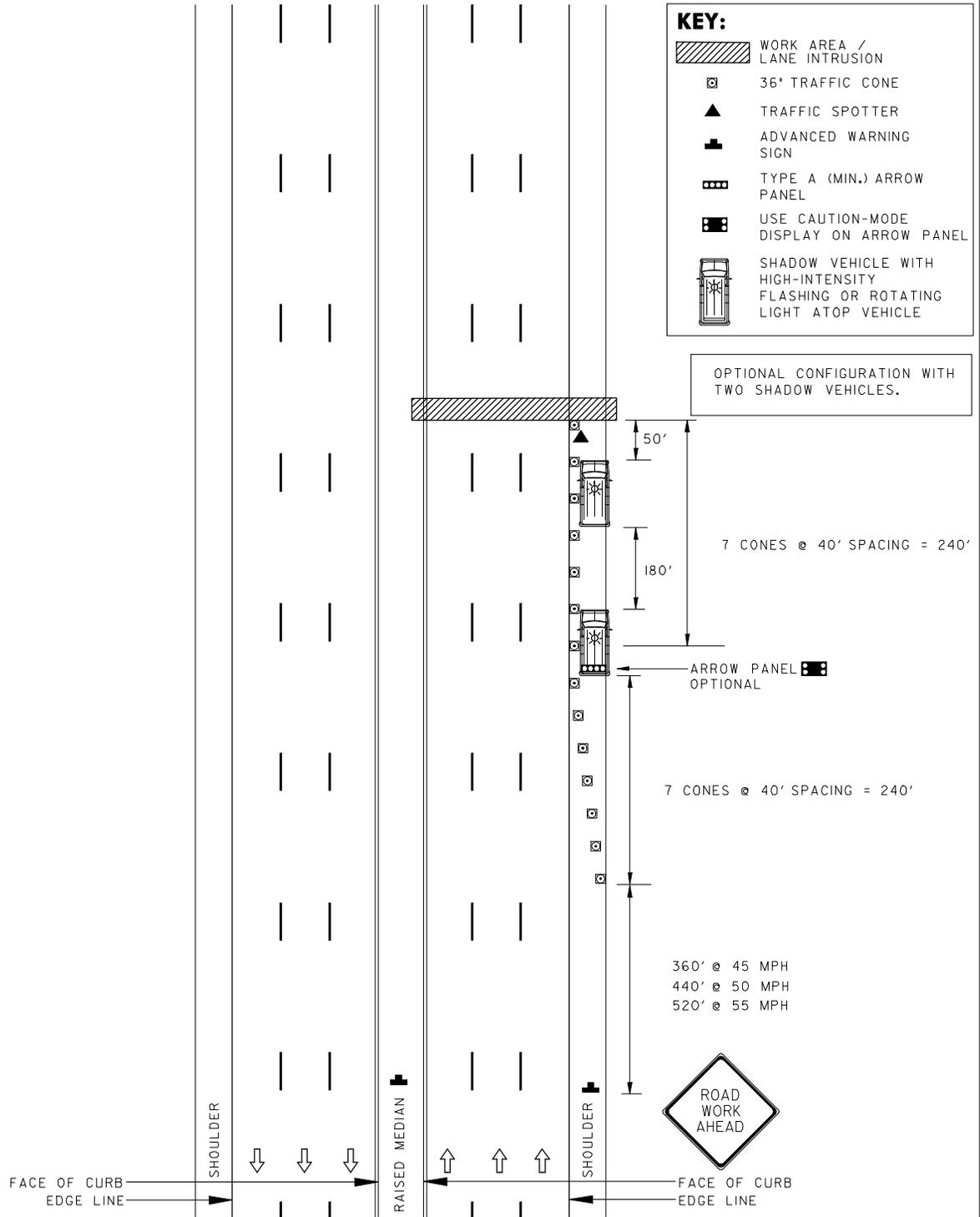
CONES SPACED AT 40' TYP.
