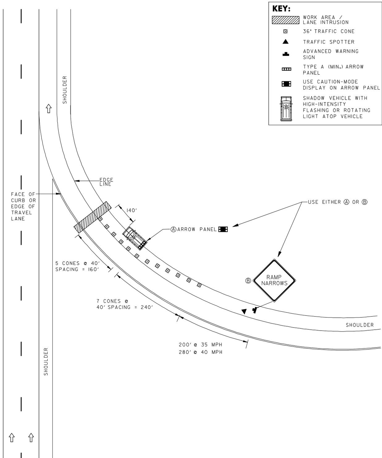
CONES SPACED AT 40' TYP.
