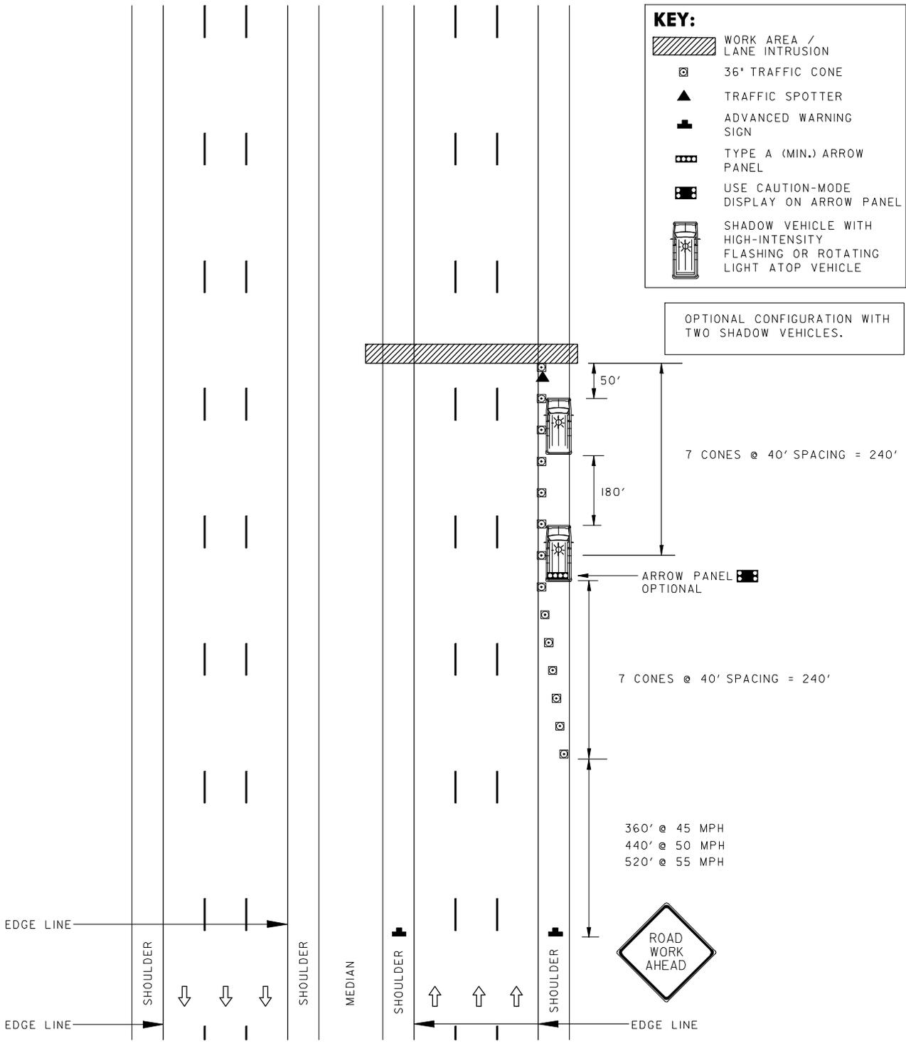
CONES SPACED AT 40' TYP.
