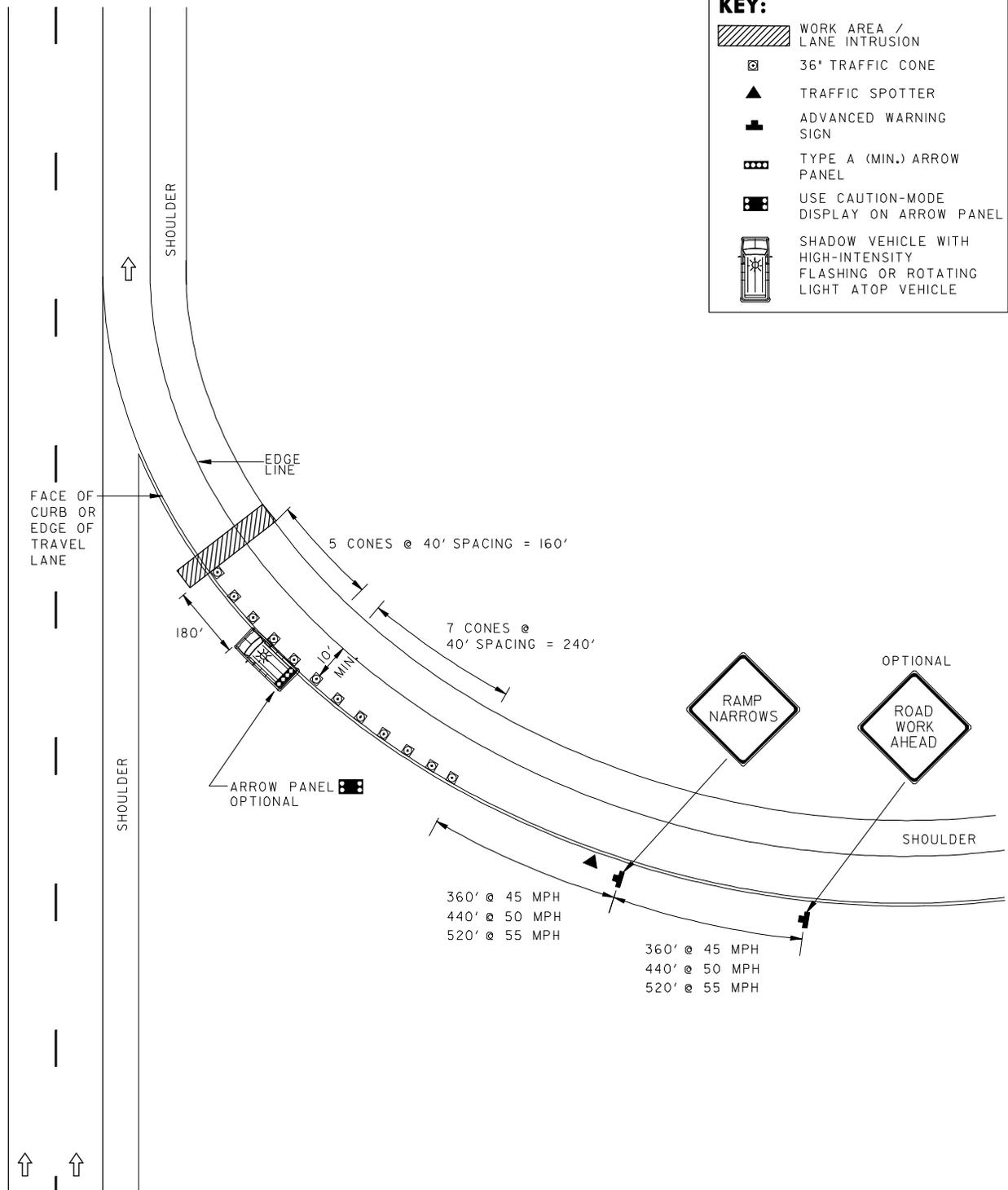
CONES SPACED AT 40' TYP.
