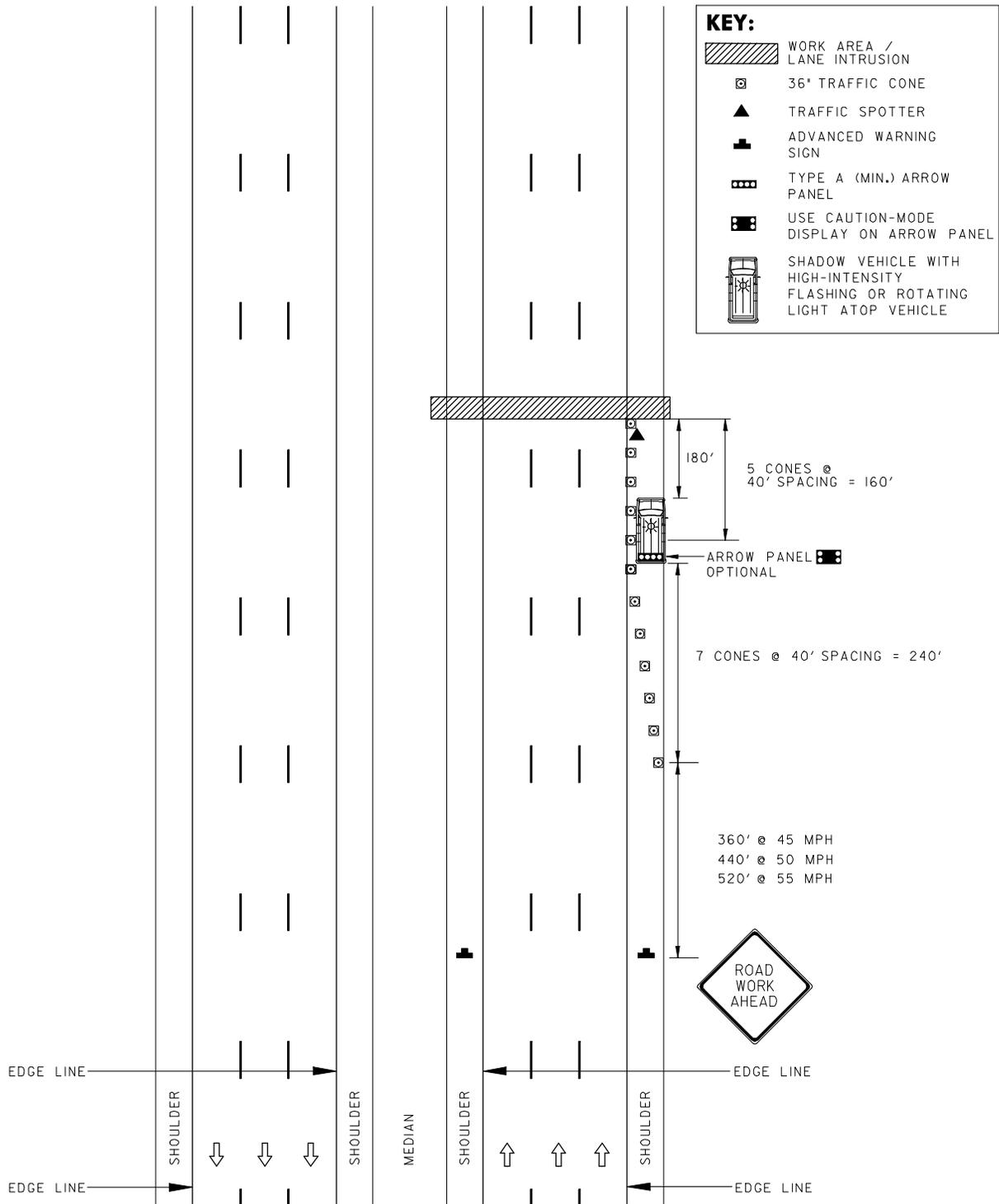
CONES SPACED AT 40' TYP.
