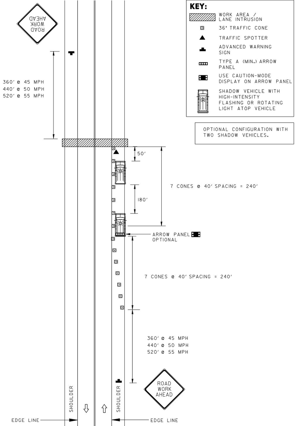
CONES SPACED AT 40' TYP.
