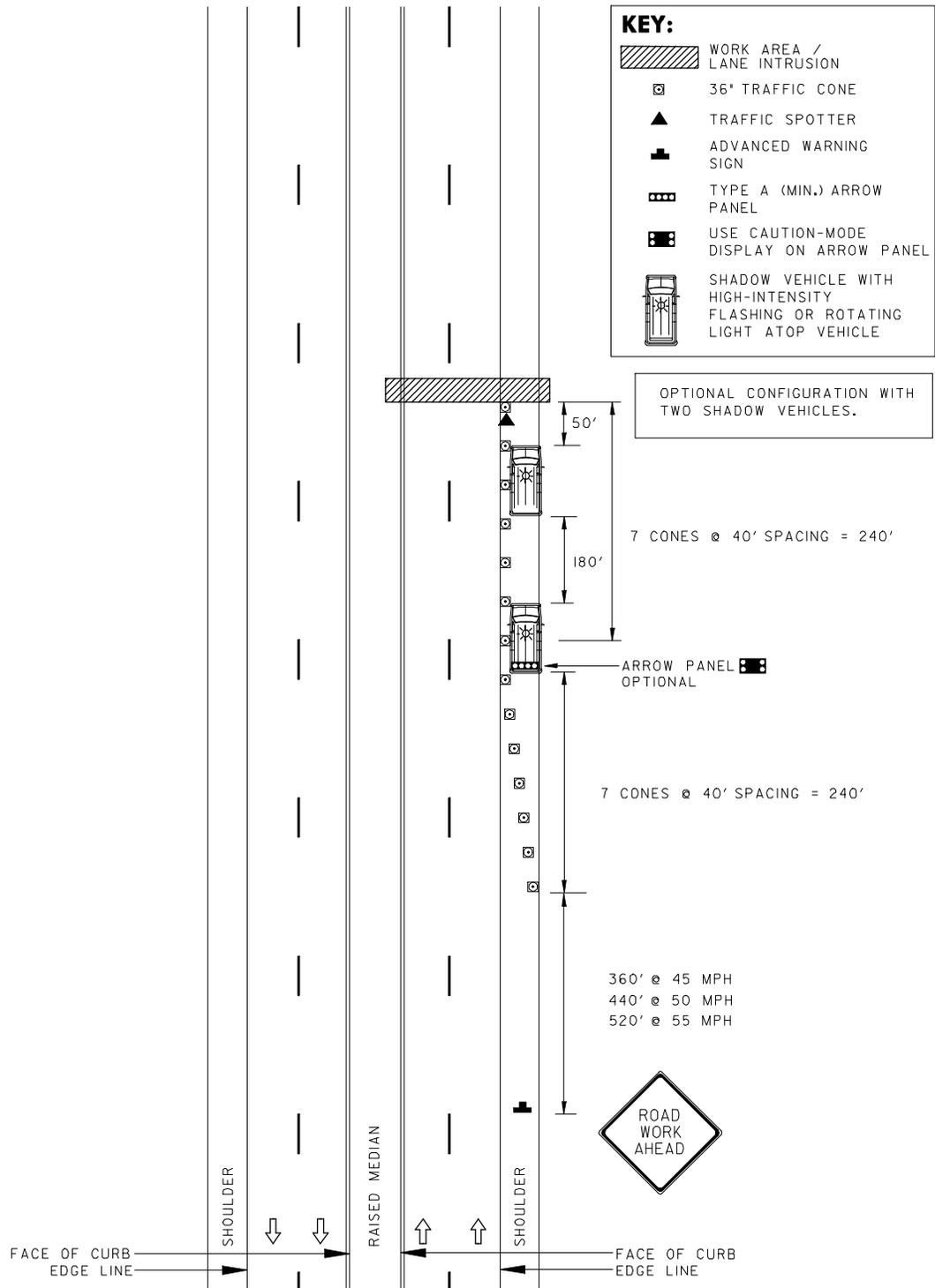
CONES SPACED AT 40' TYP.
