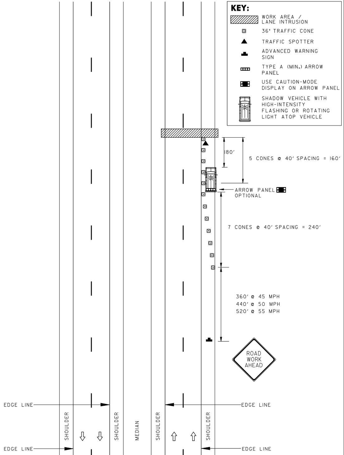
CONES SPACED AT 40' TYP.
