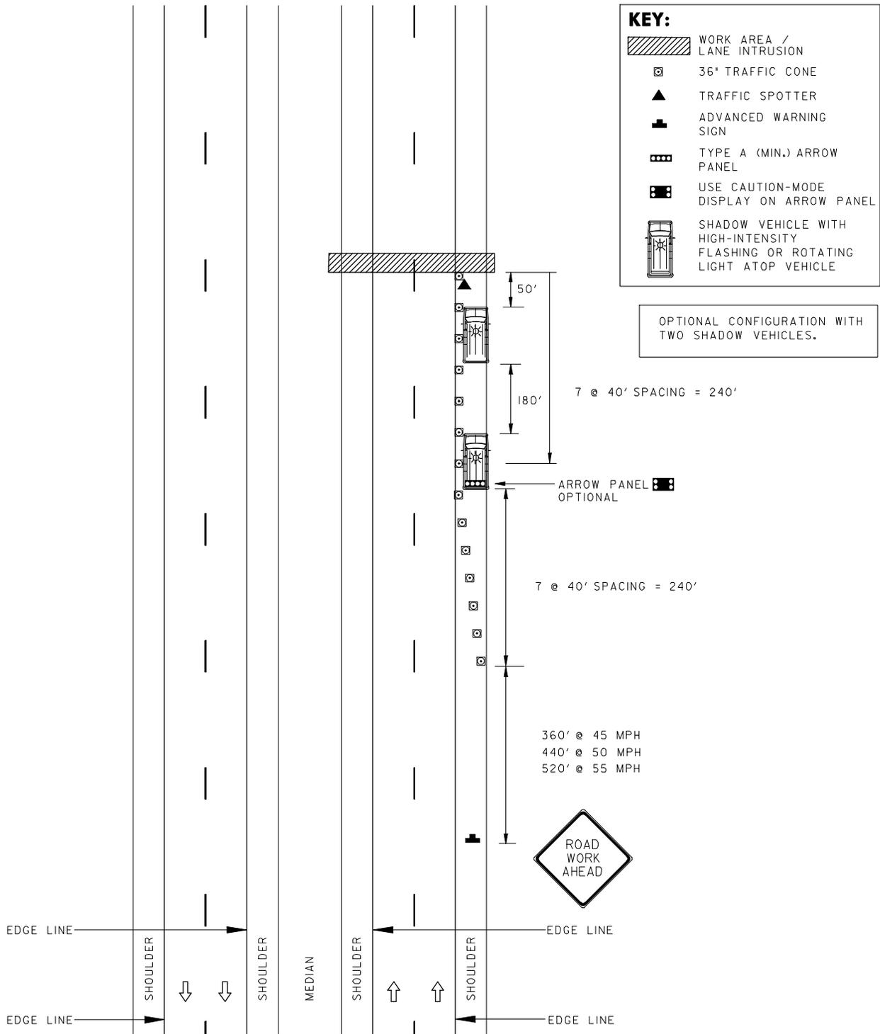
CONES SPACED AT 40' TYP.
