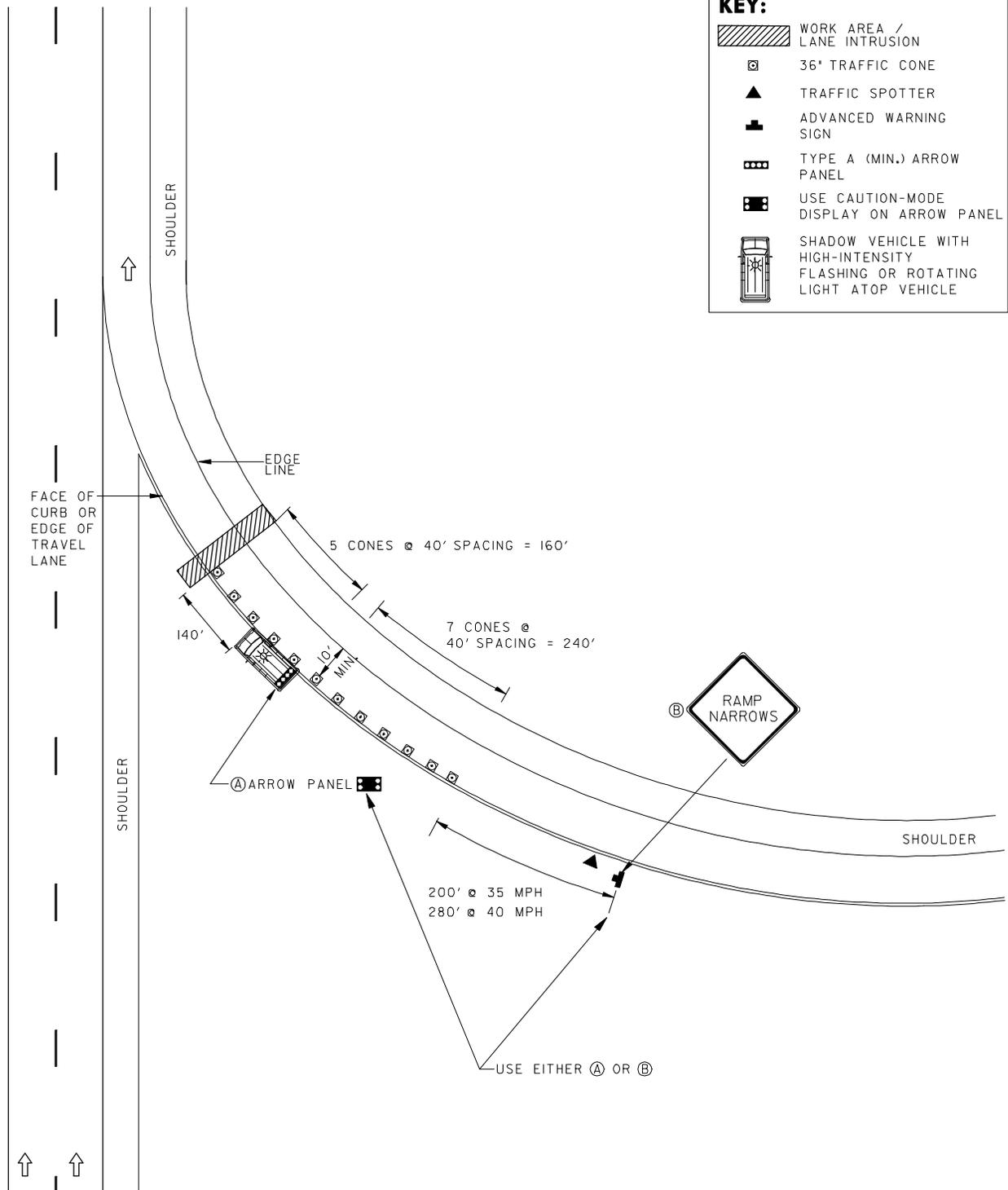
CONES SPACED AT 40' TYP.
