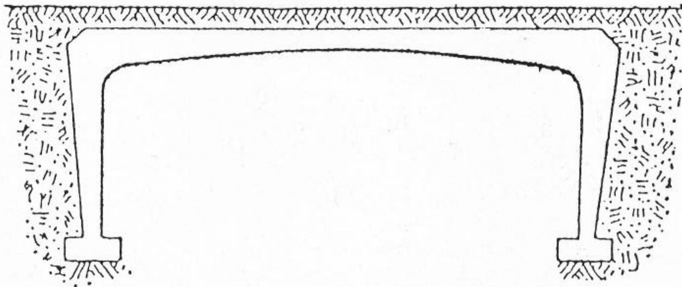
FIGURE 20: Concrete Rigid Frame Bridge Schematic
