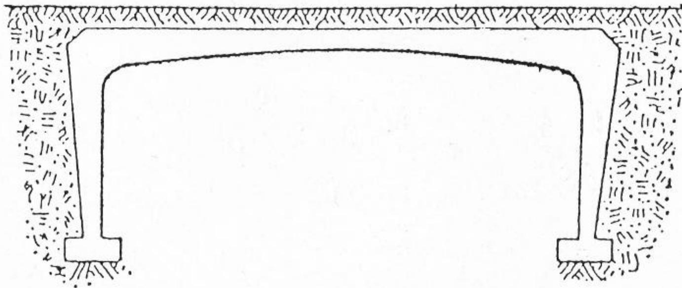
FIGURE 20: Concrete Rigid Frame Bridge Schematic
