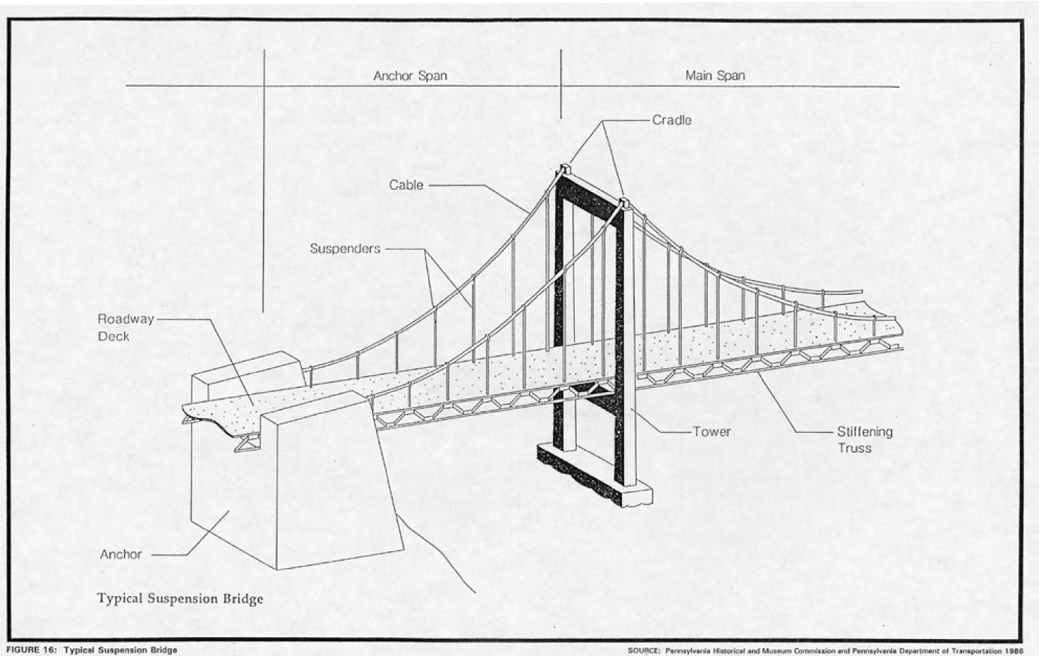
FIGURE 16: Typical Suspension Bridge
