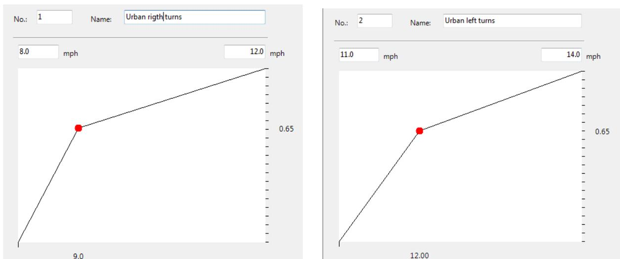
Speed reduction zones should be placed at the sharpest point on the curve of the link or connector. The speed reduction zones for turning movements should be short, usually within 5-15 feet depending on the curve length. Excessively long reduced speed zones will reduce the turning movement volume capacity and should only be used if the turning movement excessively reduces vehicle throughput.
