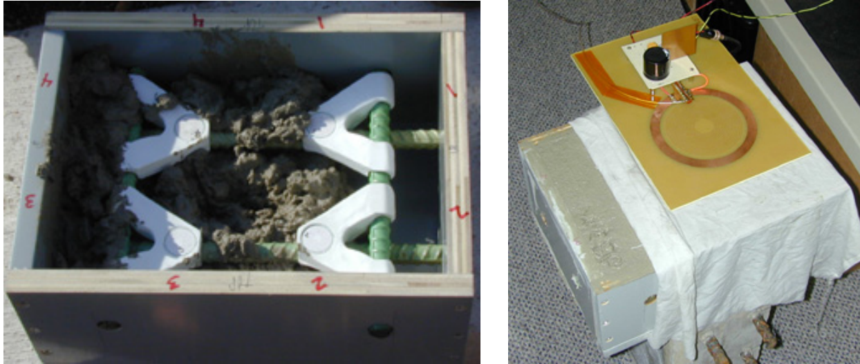
Figure 13 - Pouring Test Block and Measuring Test Block with Reader Head
