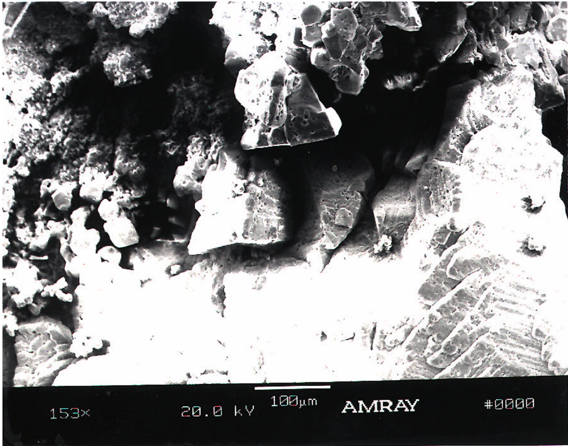
FIGURE 5.20- Calcium Carbonate Exudates
