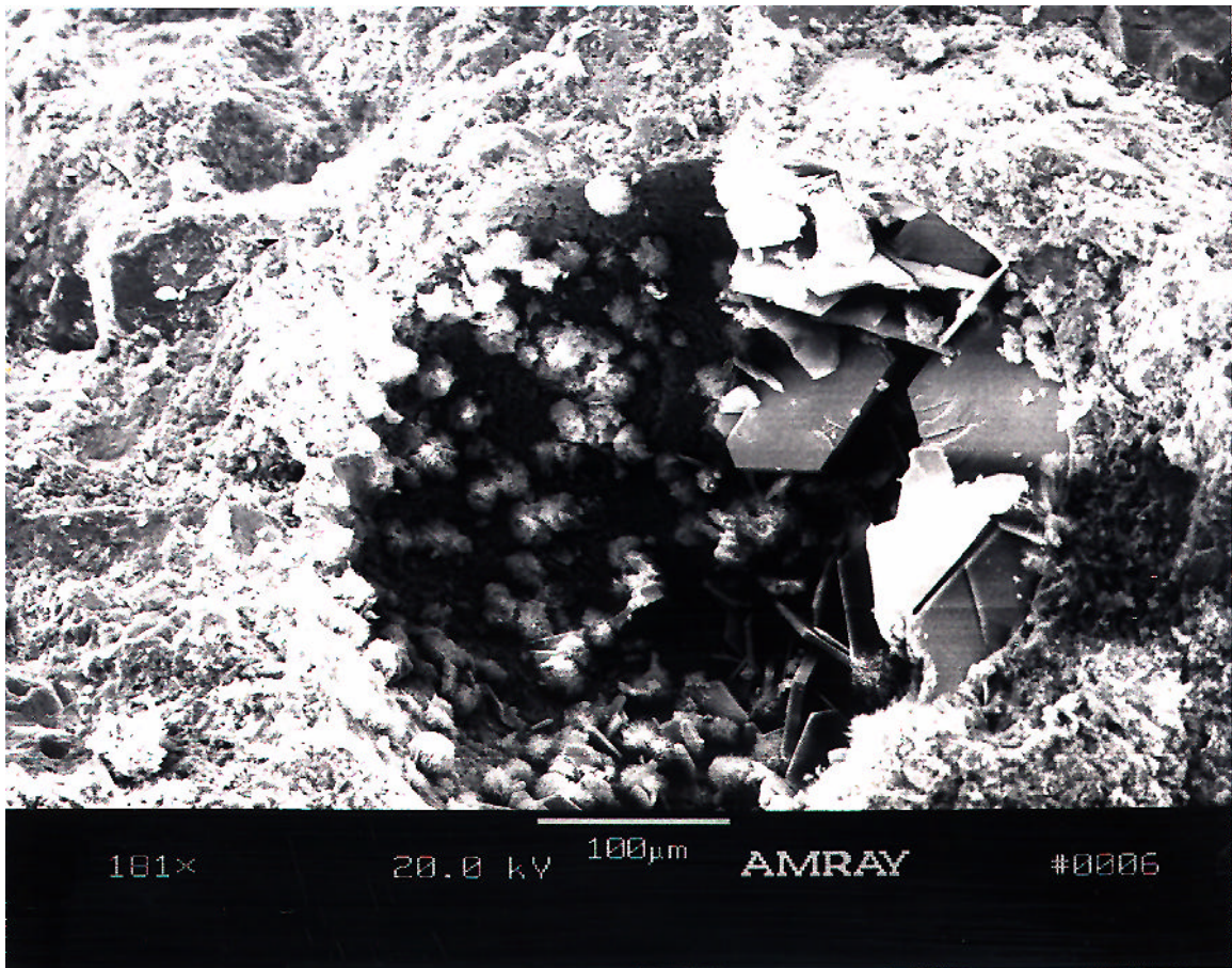
FIGURE 5.23- Ettringite and Calcium Hydroxide
