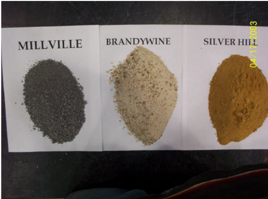
FIGURE 2.2 – Fine Aggregate Selection
