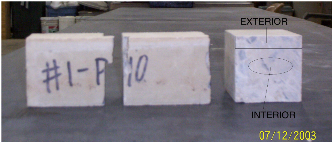
FIGURE 4.4 - Sampling SEM Specimens
