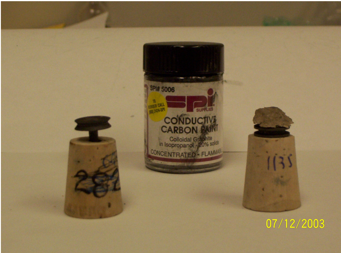
FIGURE 4.5 – Mounting of Fractured Surfaces
