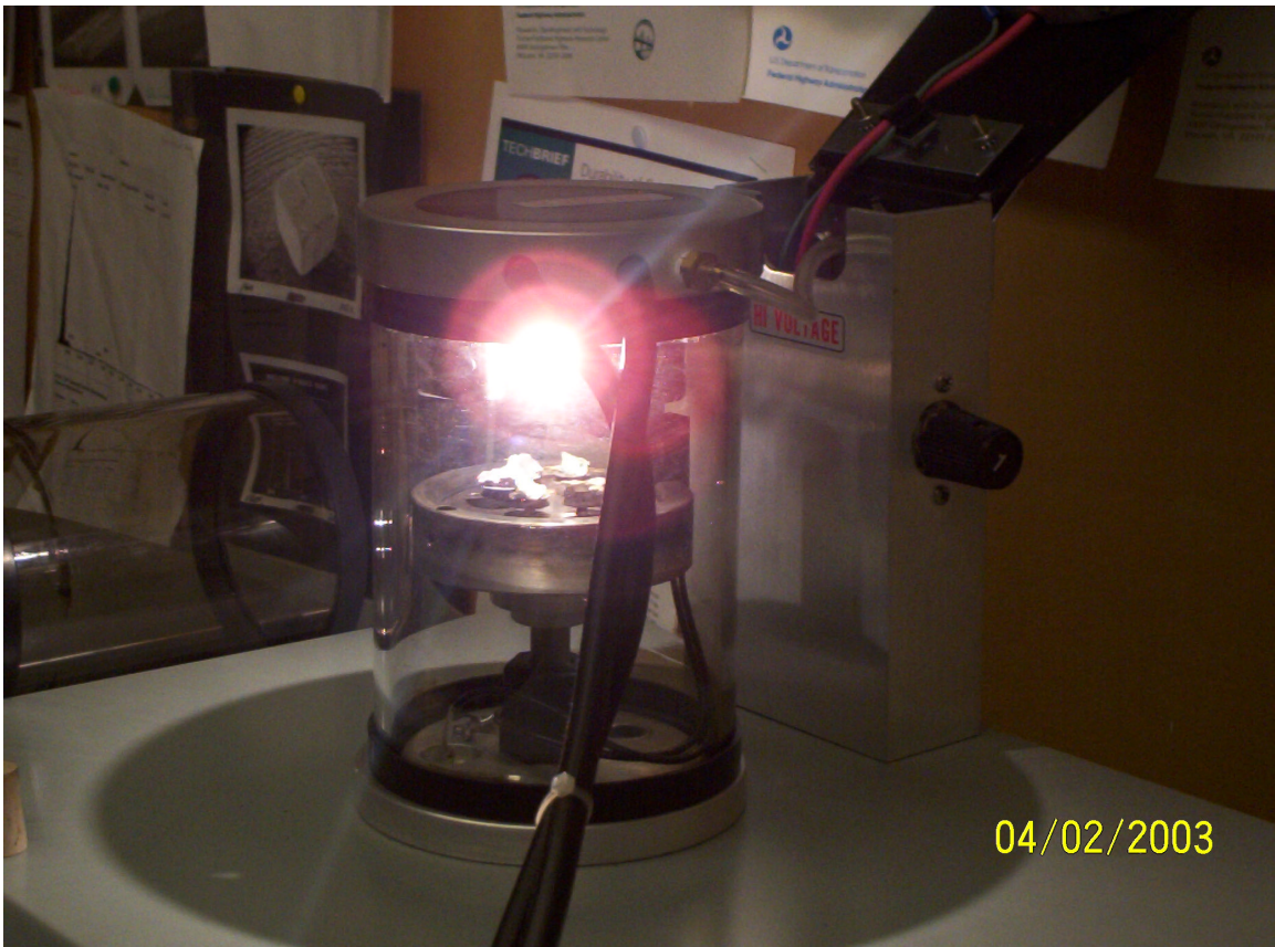
FIGURE 4.6 – Carbon Coating of Fractured Surfaces
