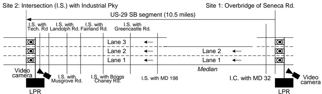
Figure 0-3: Deployment of LPR system on U.S. 29 SB segment
