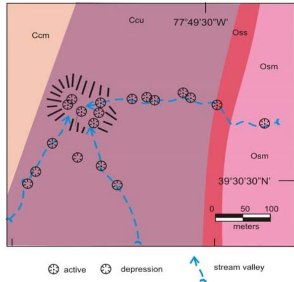
**Figure 15. GPS sketch map of an area within the Williamsport Quadrangle demonstrating the relationship between sinkholes and drainage.**
