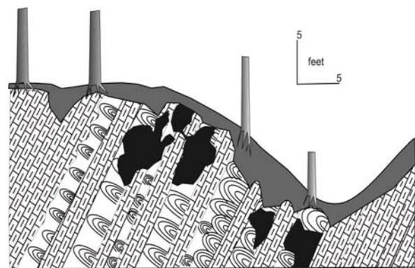
**Figure 9. A, Sketch of solution cavity preferentially forming along purer carbonate intervals bearing algal thrombolites of the middle part of the Conococheague Formation**
