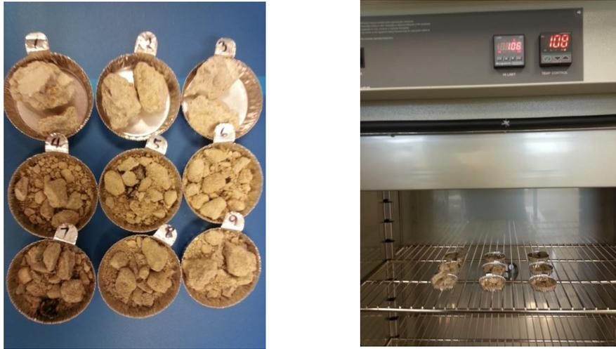
**Figure 3 Moisture content measurement of RCA**
