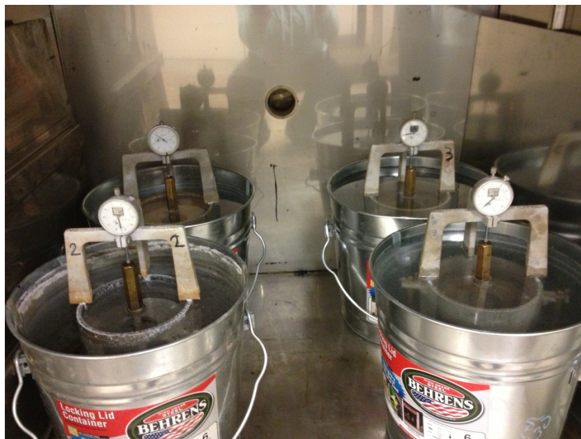
Figure 2.2. ASTM D4792 Accelerated swell test set-up
