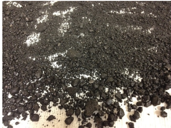
(a) (b) Figure 2.1 (a) Bitumen coating procedure and (b) bitumen coated samples
