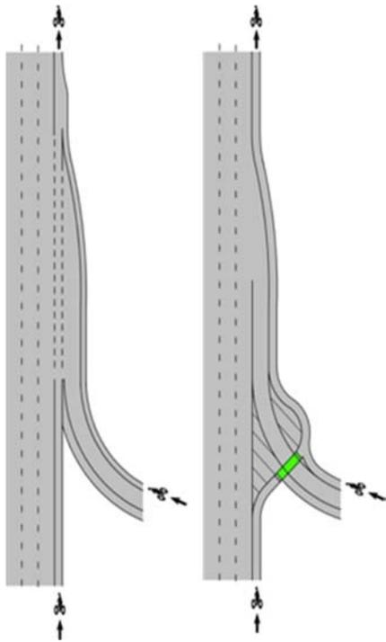
**Figure 1a Two treatments for merging ramps
