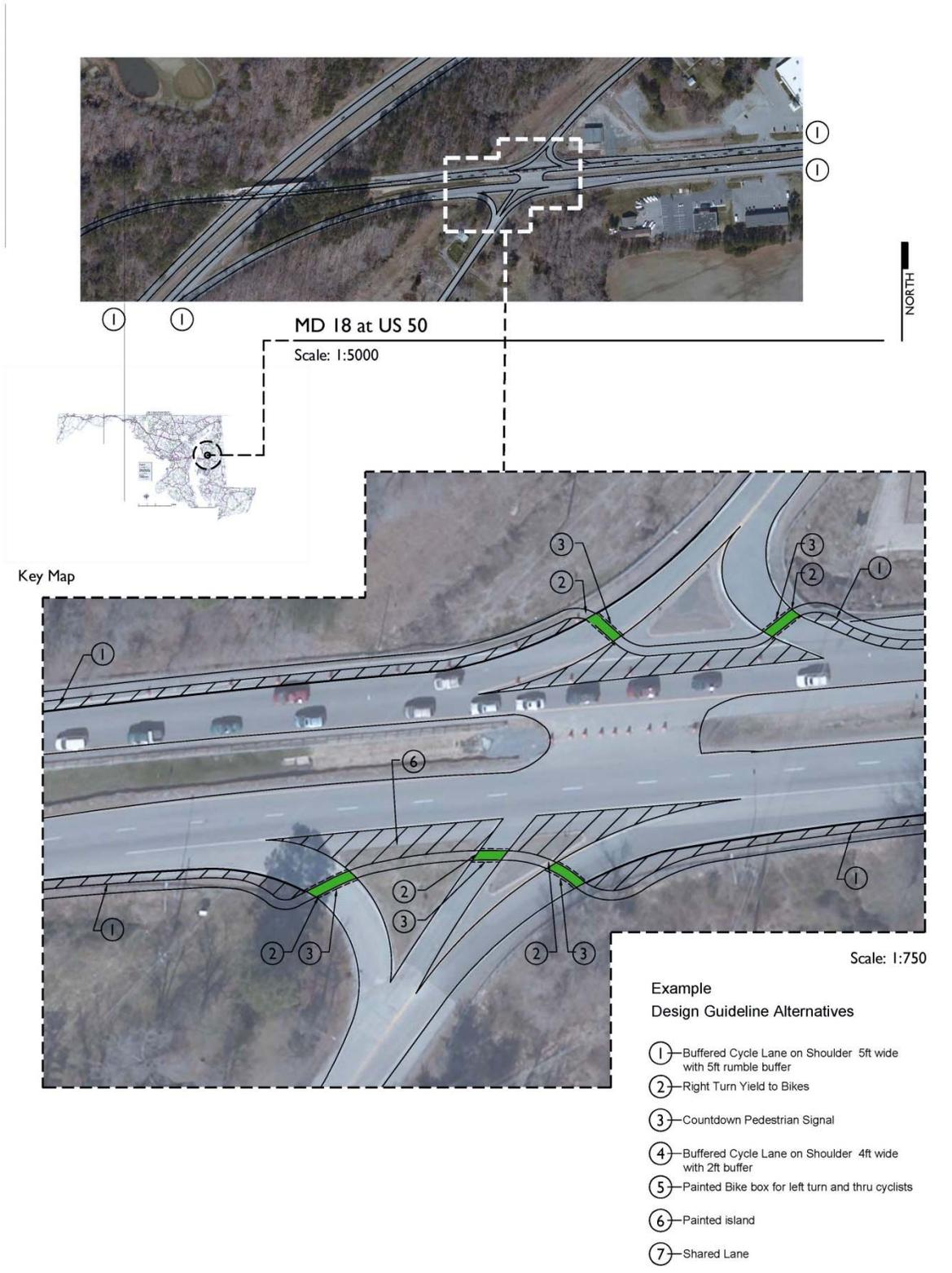
**Figure 7b Implementation Study of the At-Grade Intersection of US 50 at MD 18**
