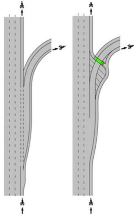
**Figure 1b Two treatments for diverging ramps
