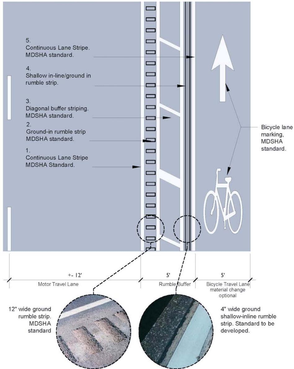
**Figure 3 Rumble-buffered bike lane design**
