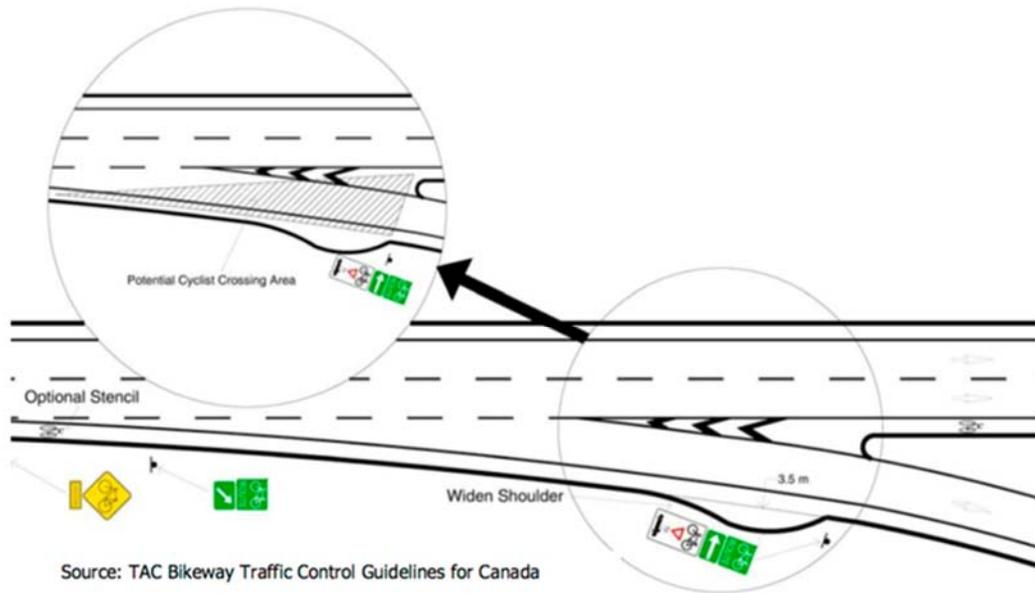
**Figure 4-4 Canadian design 2 for diverging ramps**
