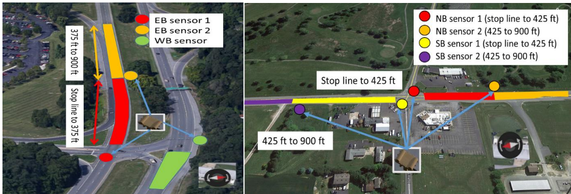
Figure A14 Design of the DZPS at the intersection of US 40 and Western Maryland Parkway
