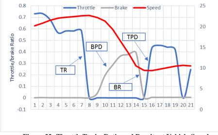
Figure 32: Throttle/Brake Ratio and Resultant Vehicle Speed
