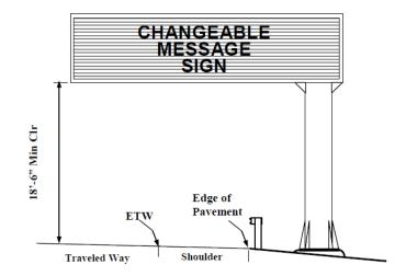
Figure 8. Simple overhead hybrid signs
