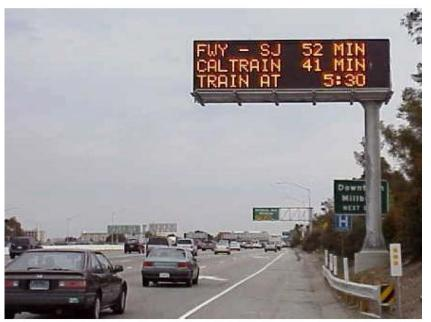
Figure 9. Example of a Permanent DMS in California
