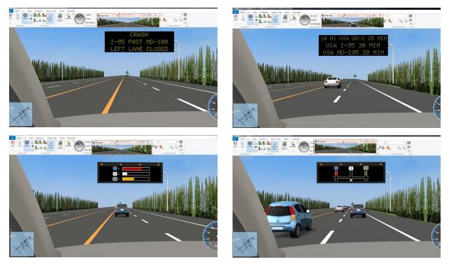
Figure 22. A Screenshot of the Simulated Driving Environment and Some DMS signs
