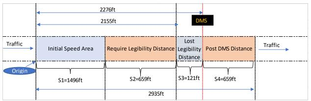
Figure 33. Description of the Segments utilized for DMS Speed Analysis
