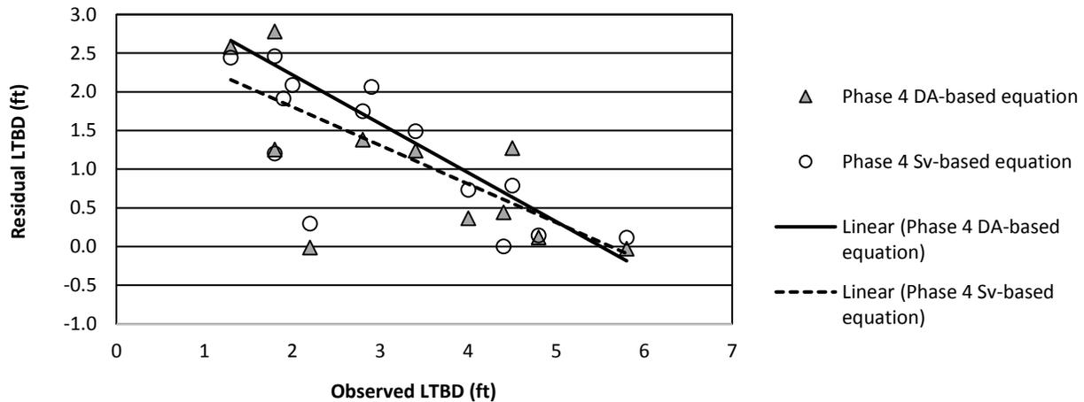
**Figure 4.8.** Comparison of residual LTBD values and observed LTBD for DA-based and  $S_v$ -based equations. Note that these residuals are for sample sites in streams without recent channelization.
