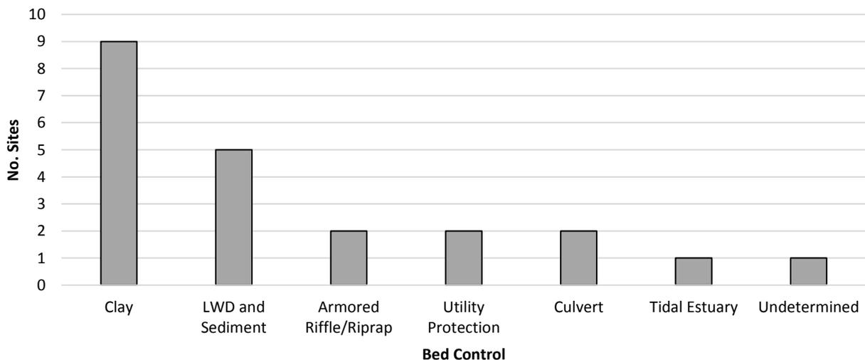
**Figure 4.7.** Frequency of bed control types downstream of LTBD measurement sites.
