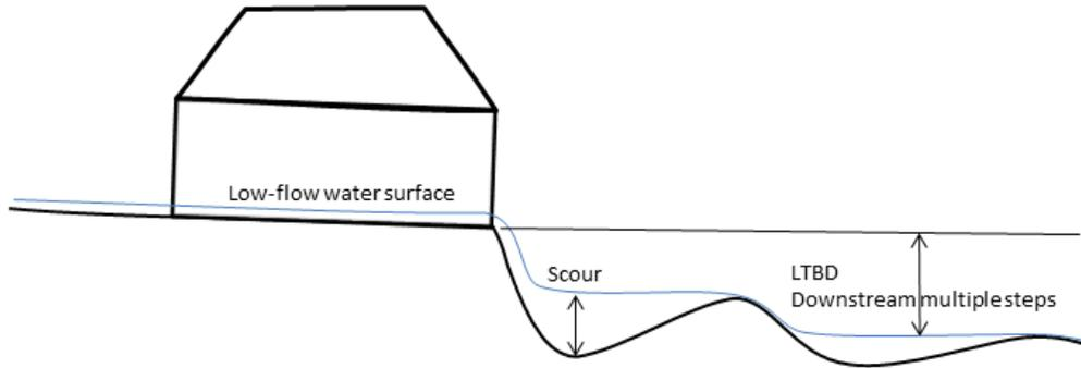
**Figure 3.2.** Typical bed profile of a culvert with downstream bed degradation and a scour pool.
