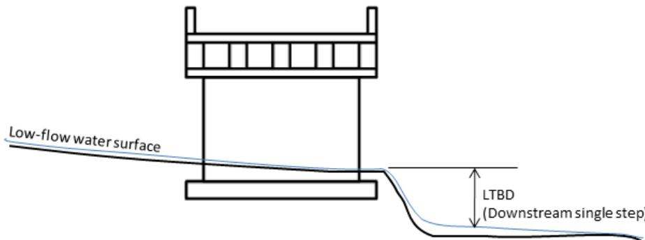
**Figure 3.3.** LTBD: uniform degradation and single step downstream.
