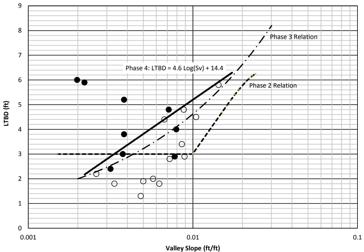
**Figure 4.3.** LTBD as a function of valley slope. A minimum value of 3 ft should be used for all sites with slopes less than 0.0034 ft/ft. Marker-filled data points represent LTBD values from sites where extensive recent channelization was identified.
