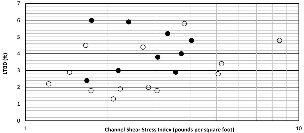
**Figure 4.4.** LTBD as a function of shear stress index. Markers filled data points represent LTBD values from sites where extensive recent channelization was identified.
