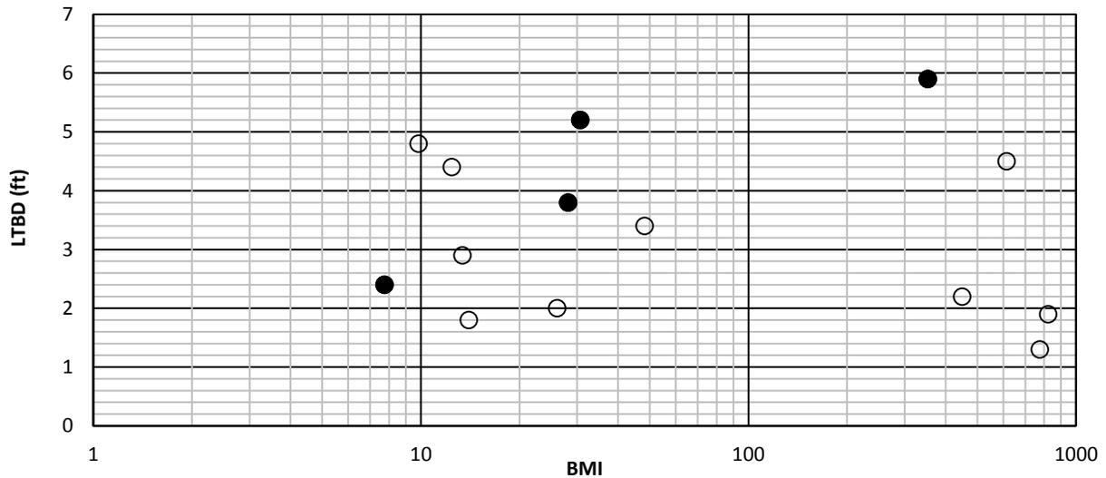
**Figure 4.5.** LTBD as a function of bed mobility index. Marker-filled data points represent LTBD values from sites where extensive recent channelization was identified.
