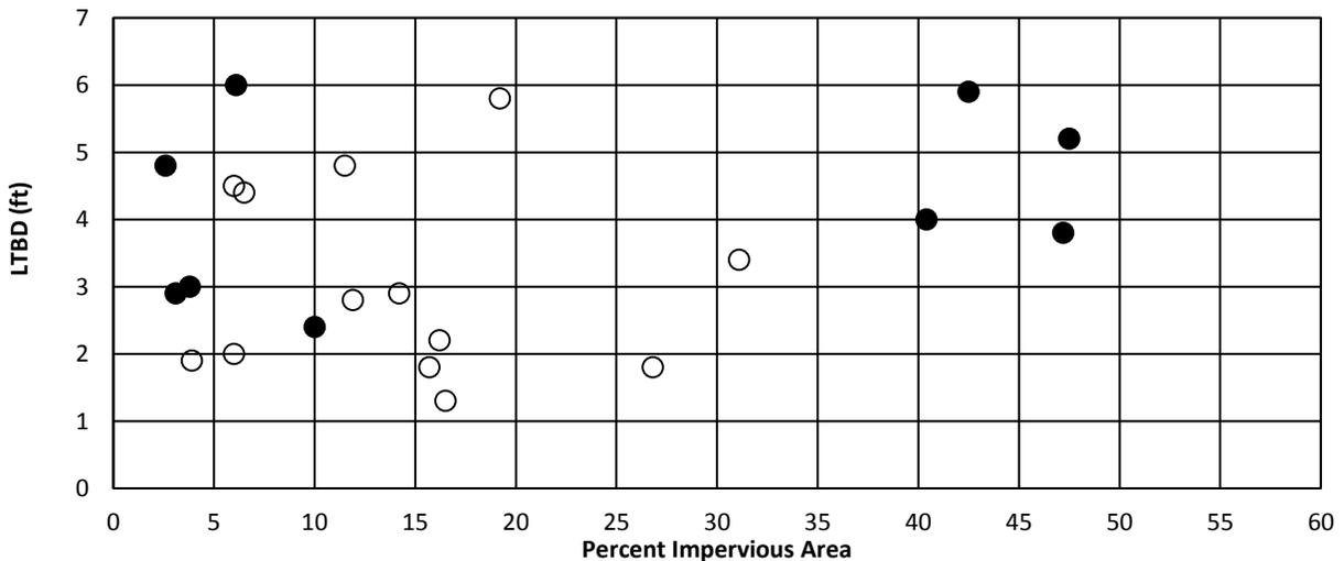
**Figure 4.2.** Variation of LTBD with percent impervious area. Marker-filled data points represent LTBD from sites where extensive recent channelization was identified.
