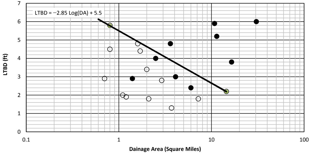
**Figure 4.1.** Variation of LTBD with drainage area for streams of the Western Shore of the coastal plain. Marker-filled data points represent LTBD values from sites where extensive recent channelization was identified.
