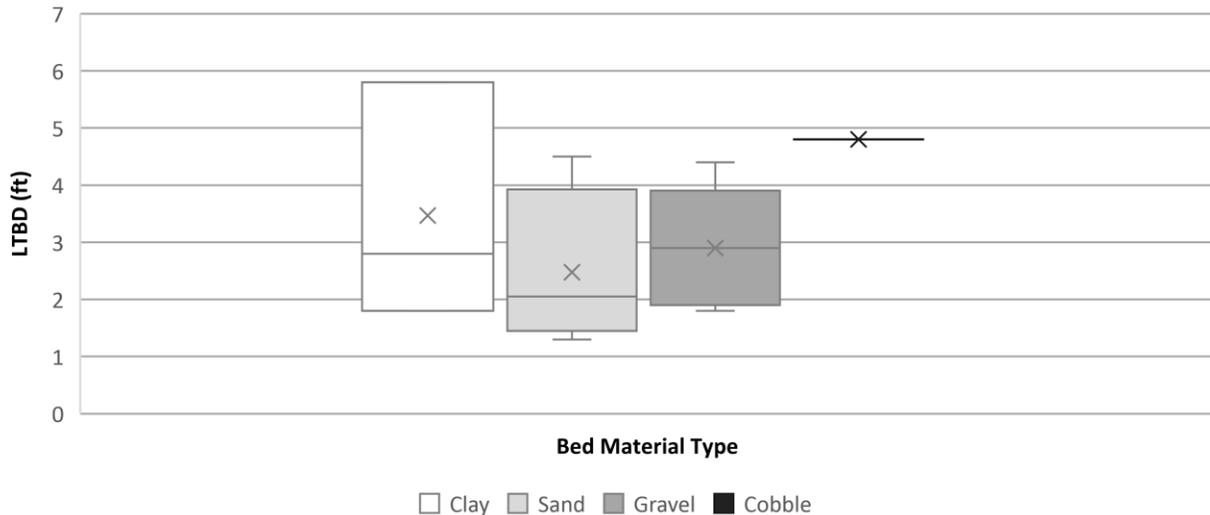
**Figure 4.6.** Box plot of LTBD as a function of bed material type. This plot excludes data from sites where extensive recent channelization was identified.
