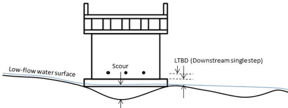
**Figure 3.5.** LTBD with scour and uniform degradation.
