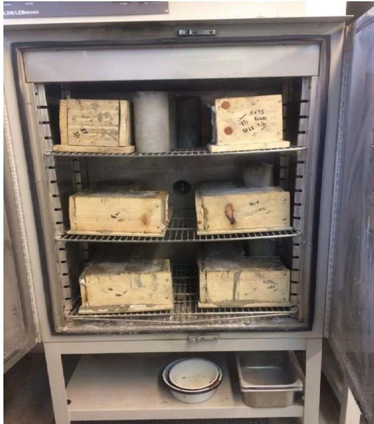
*Figure 18: Underlay specimens placed in oven for steam-curing*
