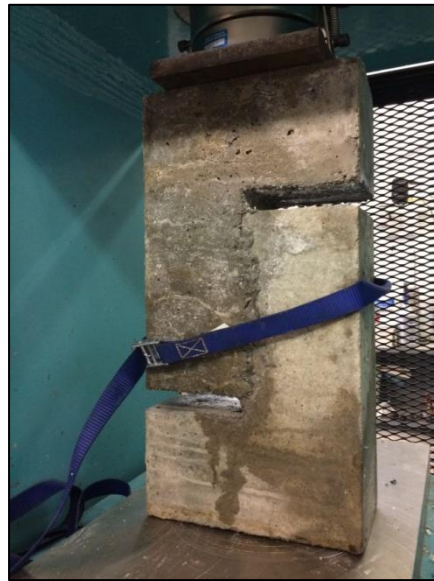
Figure 19: Testing of composite specimen for the Double-L test (Shear Bond Strength)
