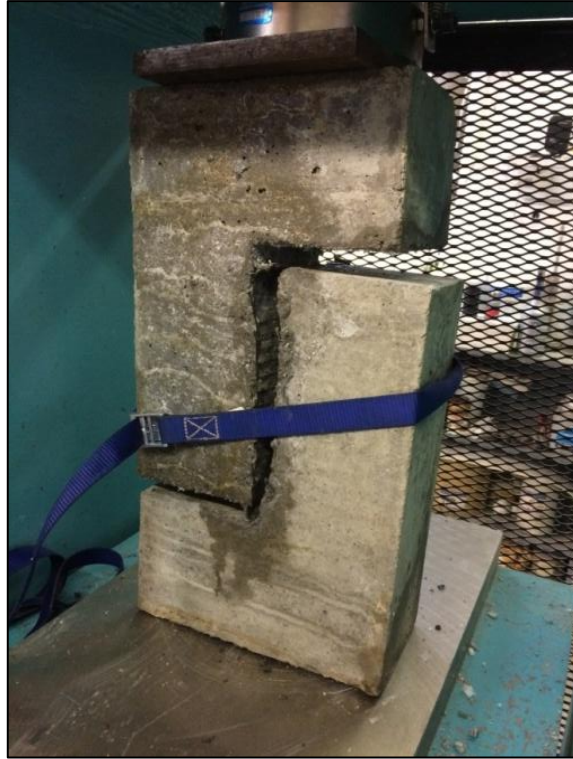
Figure 22: Composite specimen after shear bond failure in the Double-L test
