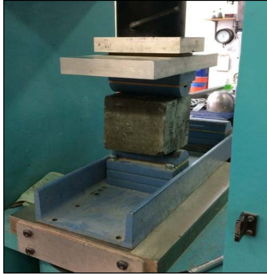
Figure 20: Testing of composite specimen for the Split-Prism test (Tensile Bond Strength)
