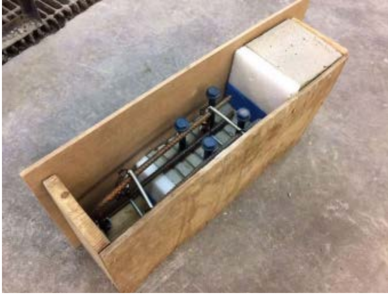
Figure 13: Underlay half with anchors protruding from the bond surface prior to pouring of overlay concrete
