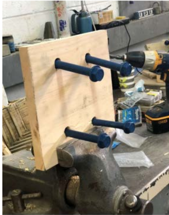
Figure 12: Tapcon anchors inserted in the bond panel
