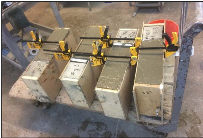
Figure 14: Composite specimen with freshly poured overlay concrete
