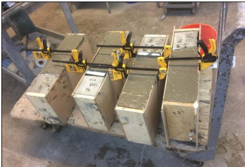
*Figure 14: Composite specimen with freshly poured overlay concrete*
