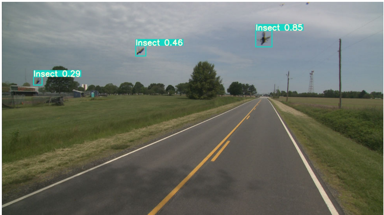
Figure 37. Sample output image with 3 insect objects identified by YOLO v3 model
