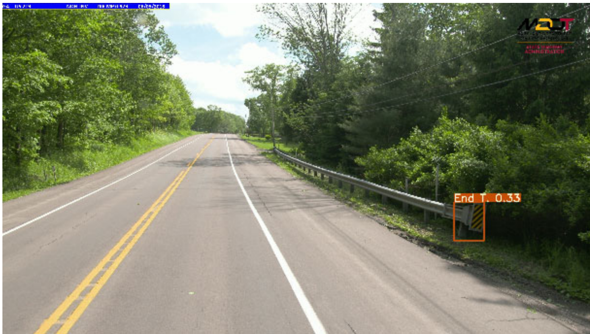
Figure 31. Sample output image with traffic barrier end treatment object identified by YOLO v3 model with inclined traffic barrier end treatment and shrubs in the background
