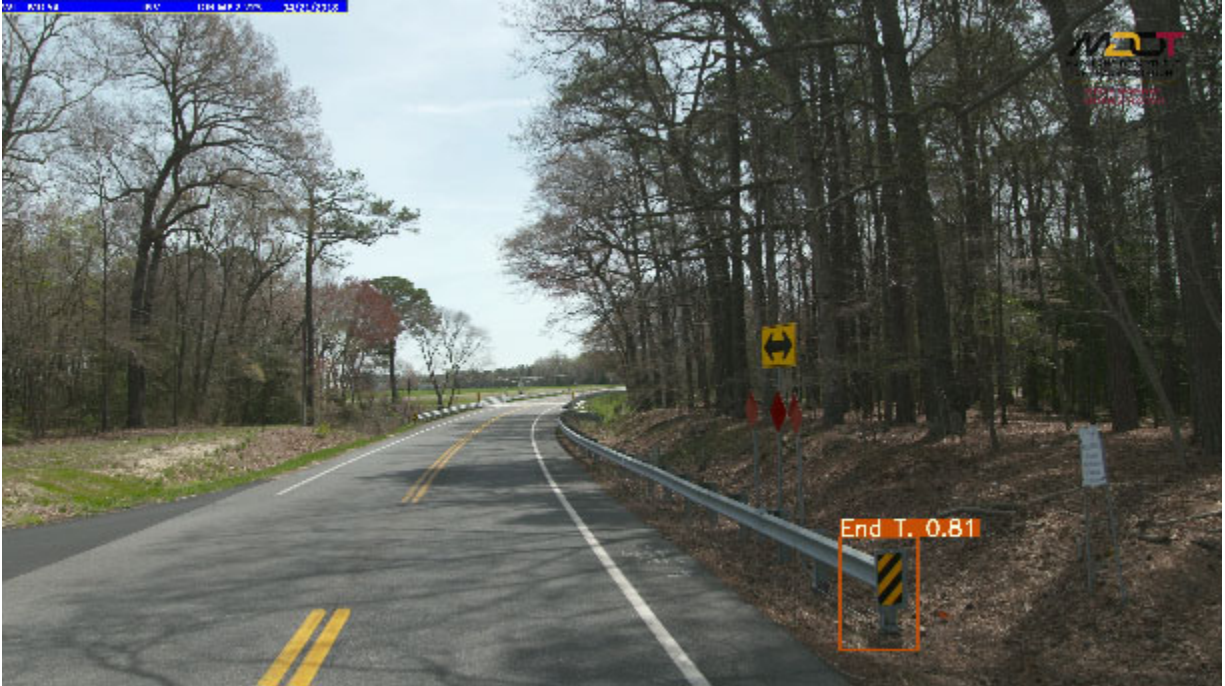
Figure 26. Sample output image with traffic barrier end treatment object identified by YOLO v3 model with woods background and with close-up view of traffic barrier end treatment
