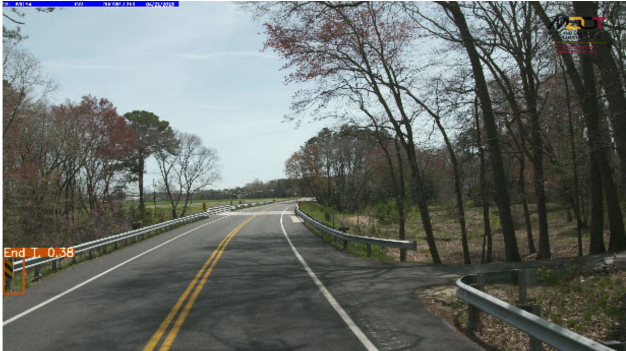
Figure 30. Sample output image with traffic barrier end treatment object identified by YOLO v3 model with partial view of traffic barrier end treatment on the left
