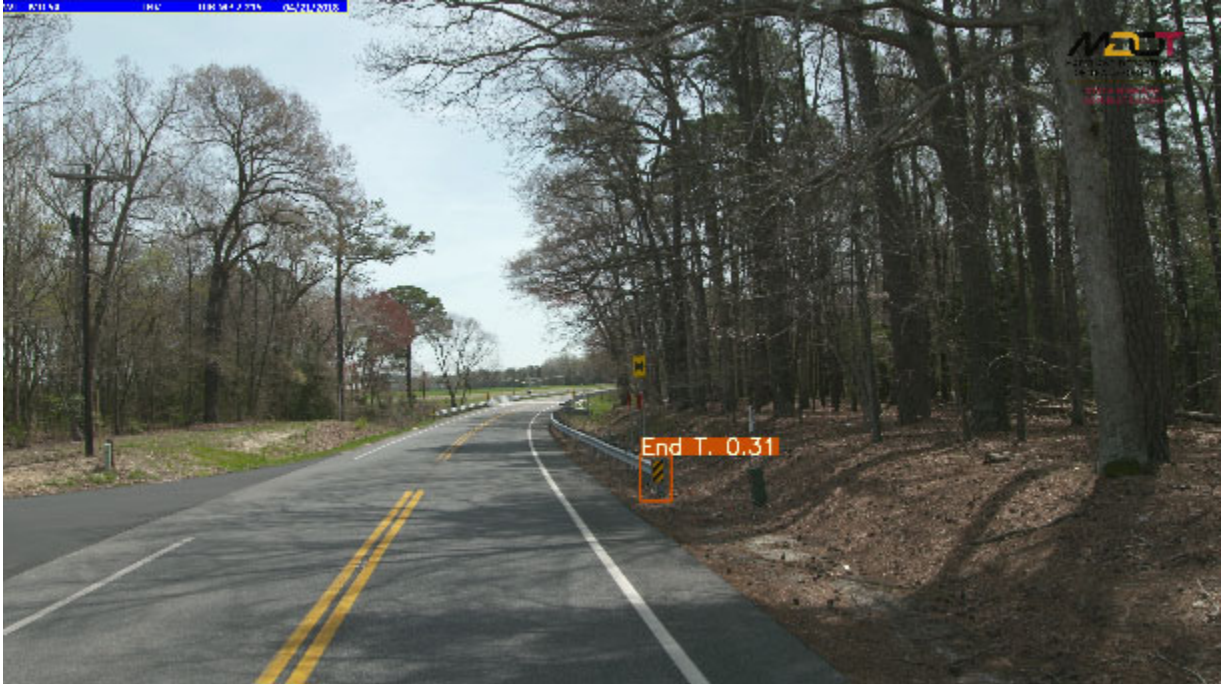
Figure 28. Sample output image with traffic barrier end treatment object identified by YOLO v3 model with small-scaled traffic barrier end treatment in the picture
