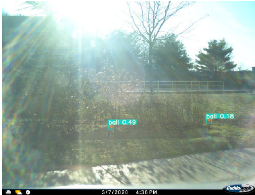
Figure 18. Sample output image with ball objects identified by YOLO v3 model in an overexposed photo from remote cameras
