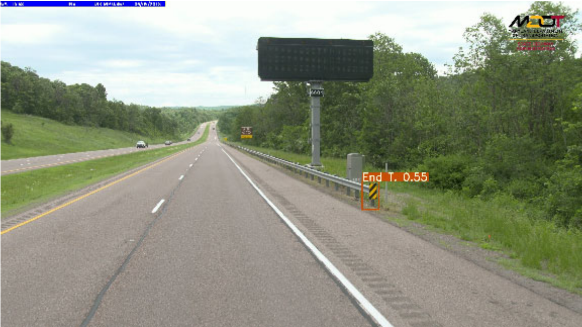
Figure 22. Sample output image with traffic barrier end treatment identified by YOLO v3 model
