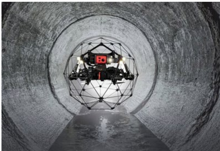
Figure 1. Flyability Elios 2 UAS conducting culvert inspection.
