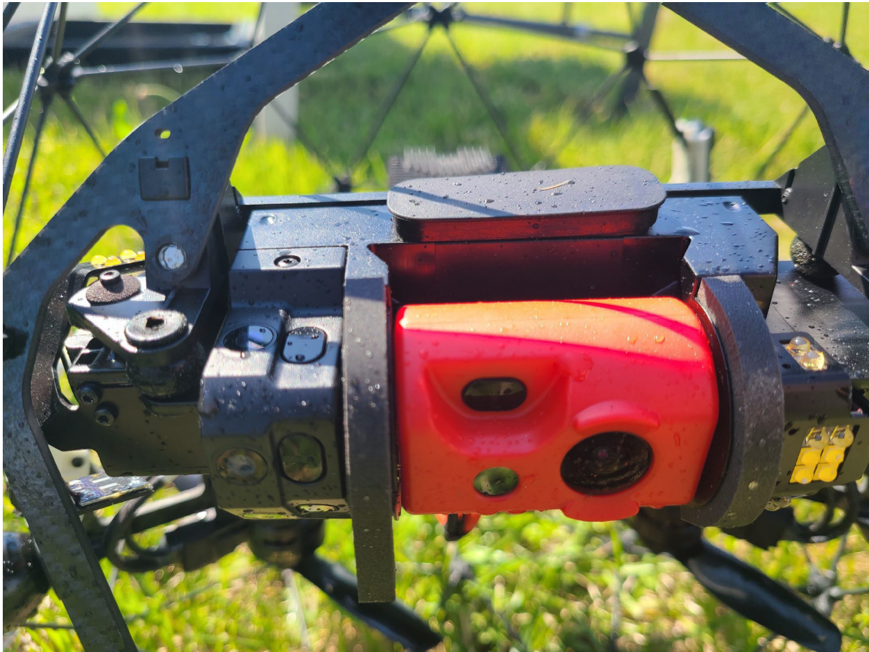
Figure 7. Elios 2 after confined space water testing.
