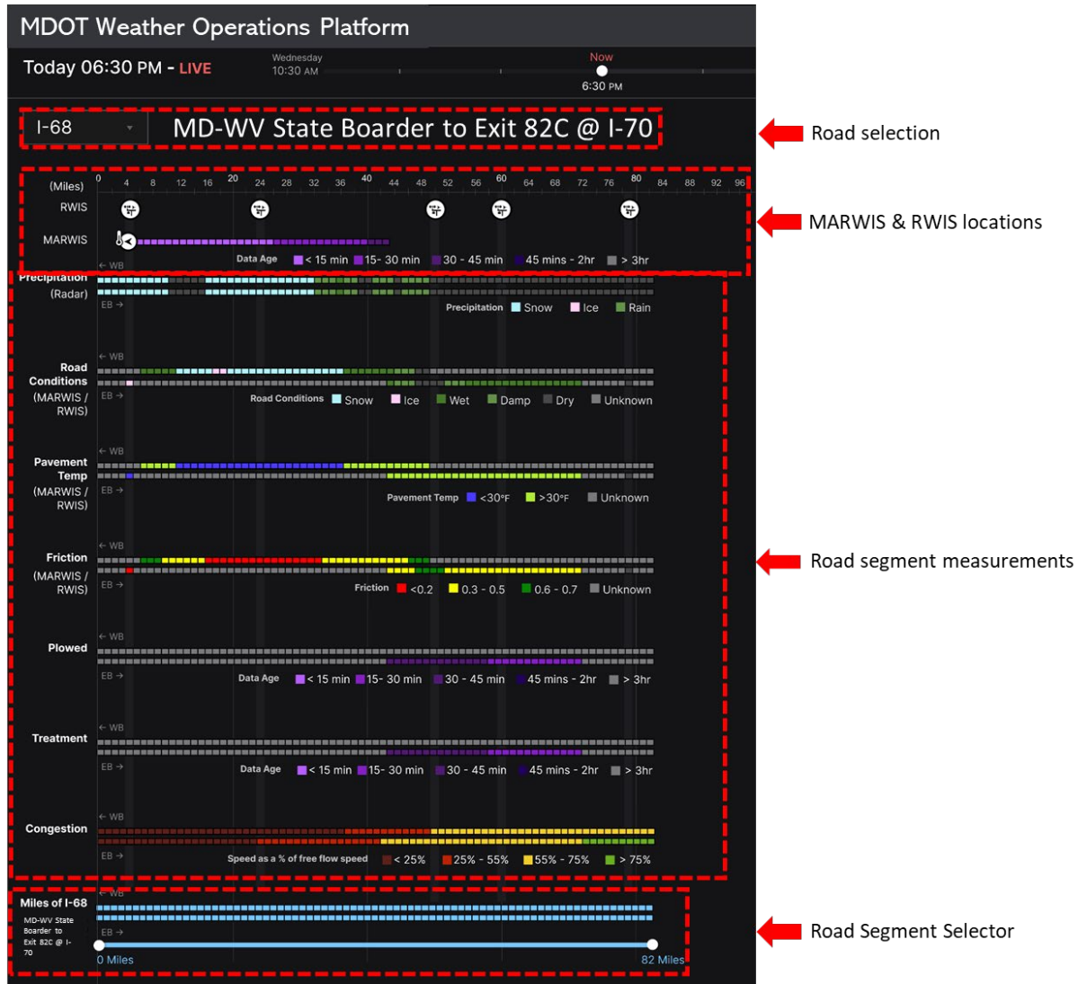
Figure 27: Road View – Road Condition Summary
