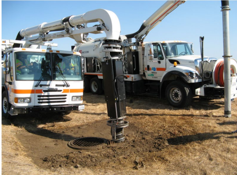
Figure 7. ARDVAC and A Standard Vacuum Truck for Drain Inlet Cleaning
