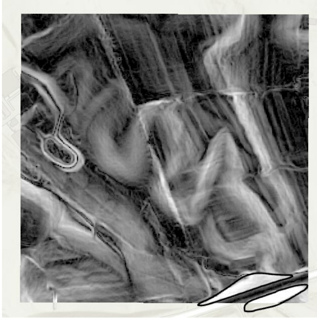
Figure 9. Sample training chip with a 256x256 cell size for embankment detection model
