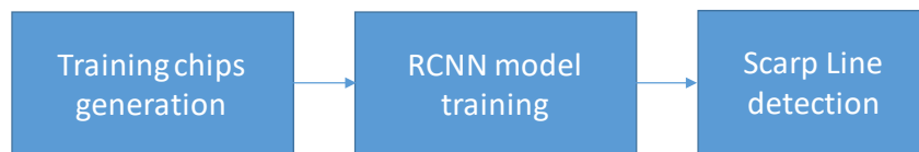
Figure 24. Flowchart of machine learning-enabled automated scarp polylines generation
