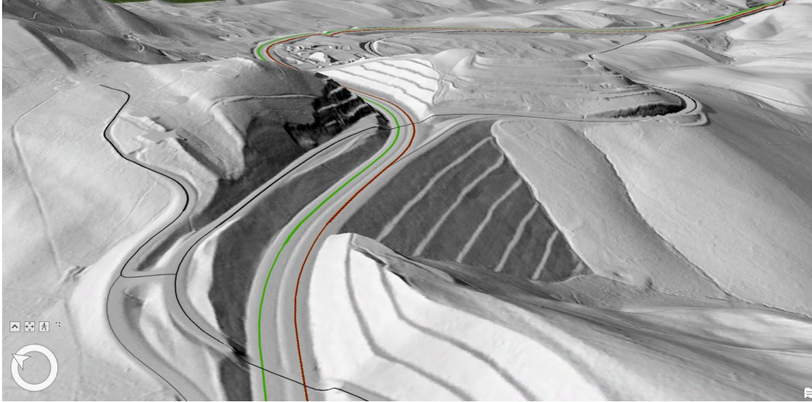
Figure 5: Lidar Hillshade, Courtesy of Maryland iMAP, illustrating the digital elevation model used to identify zones of elevation change adjacent to highways
