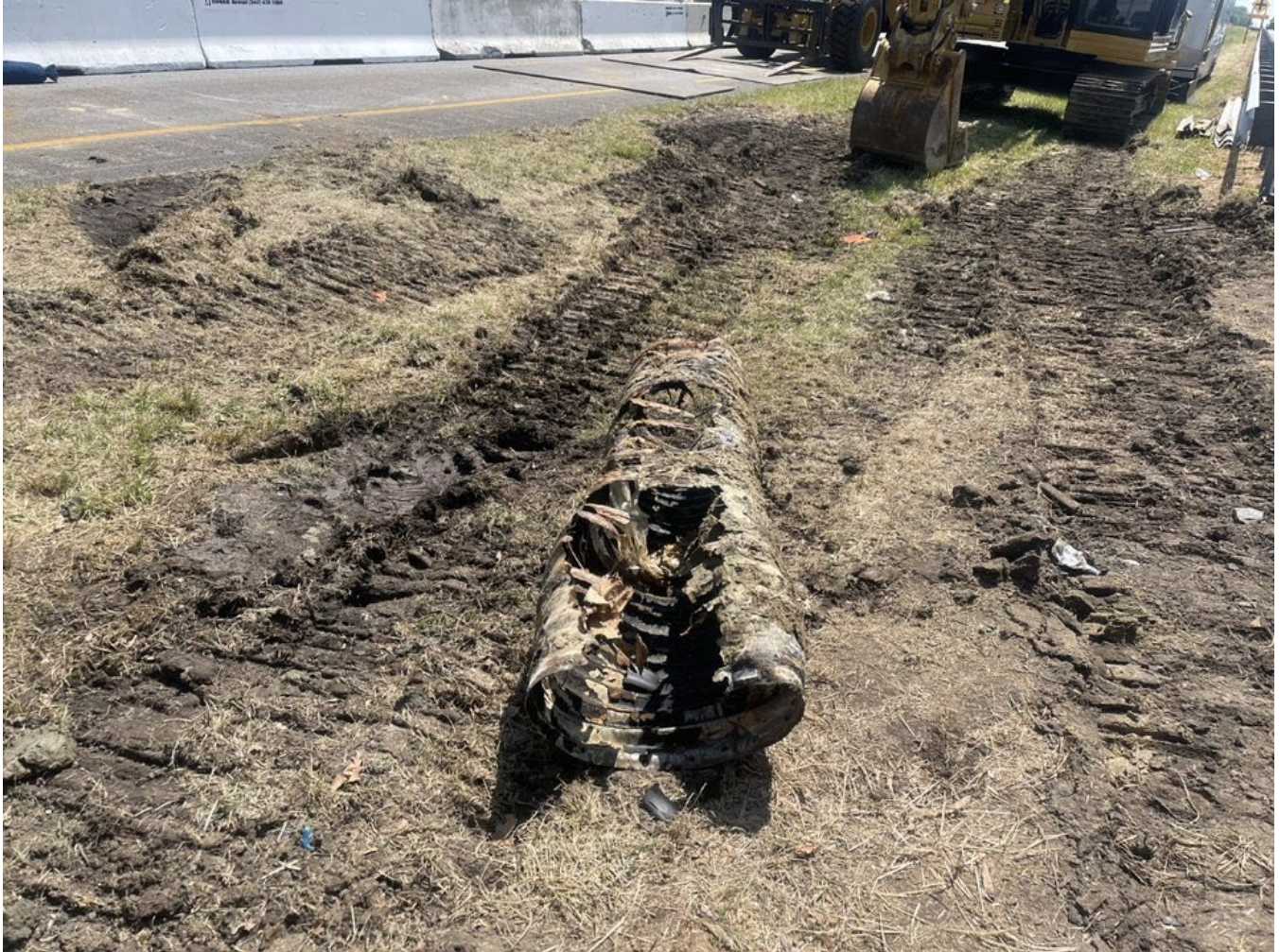
Figure 13: Damaged Corrugated Metal Pipe after Extraction. This pipe was the cause of the subsurface void.
