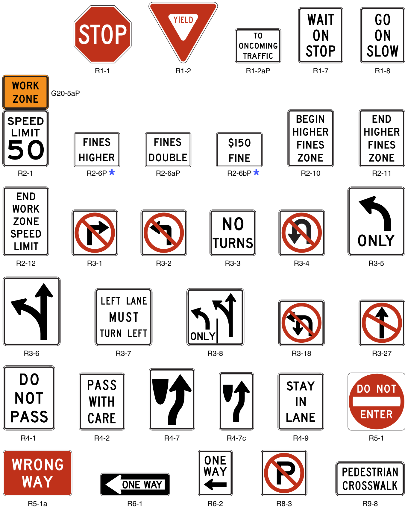
Figure 6F-3. Regulatory Signs and Plaques in Temporary Traffic Control Zones (Sheet 1 of 2)
