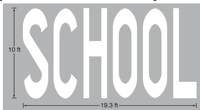
Figure 7C-1. Two-Lane Pavement Marking of “SCHOOL”
