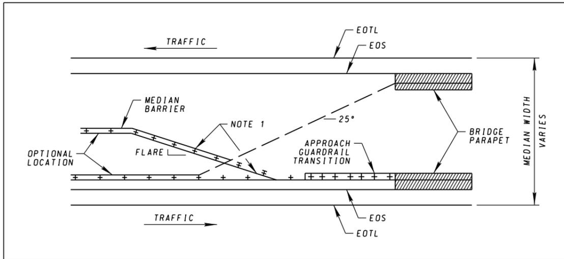
*Note 1: For W-Beam barrier, barrier should not be placed in areas that are not recommended in Std. MD-605.31 unless the slopes are modified as described in Section V of these Guidelines.*
