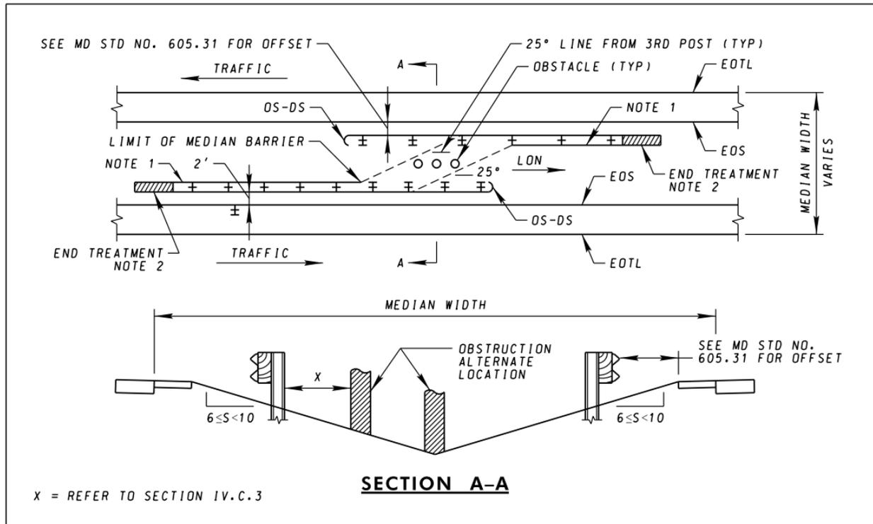
*Note 1: If the back of the barrier is within the “Barrier Optional” or “Evaluate Need for Barrier” regions of Figure 6-1 of the RDG, a TBWB-MB is required*
