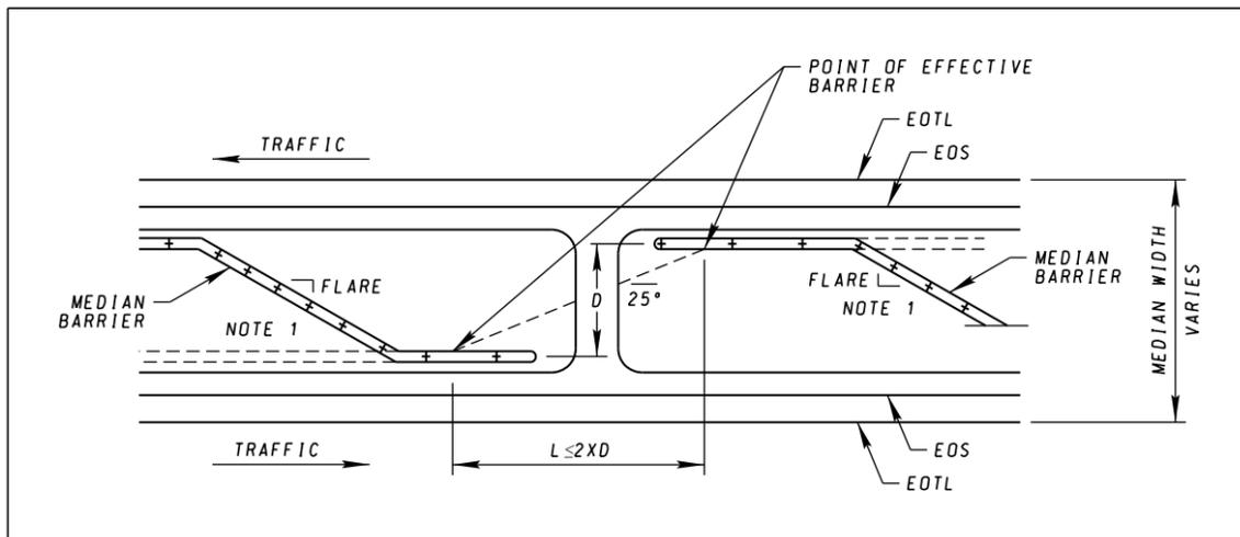
*Note 1: For W-Beam barrier, barrier should not be placed in areas that are not recommend in Std. MD-605.31 unless the slopes are modified as described in Section V of these Guidelines.*
