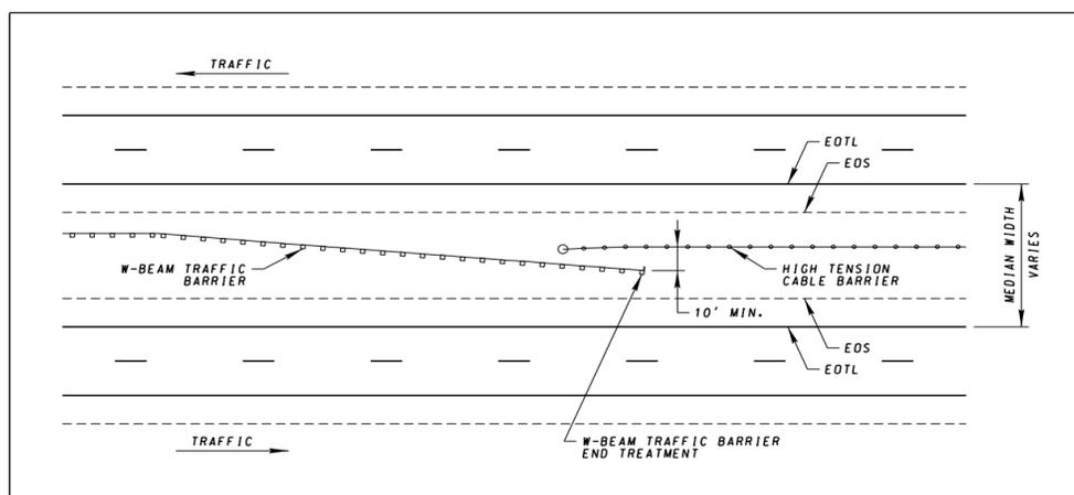
**Figure 6: High-Tension Cable Barrier/W-Beam Traffic Barrier Transition Layout**
