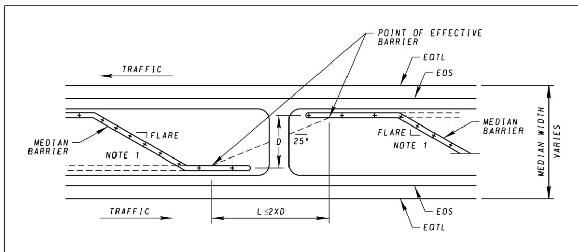
*Note 1: For W-Beam barrier, barrier should not be placed in areas that are not recommended in Std. MD-605.31 unless the slopes are modified as described in Section V of these Guidelines.*
