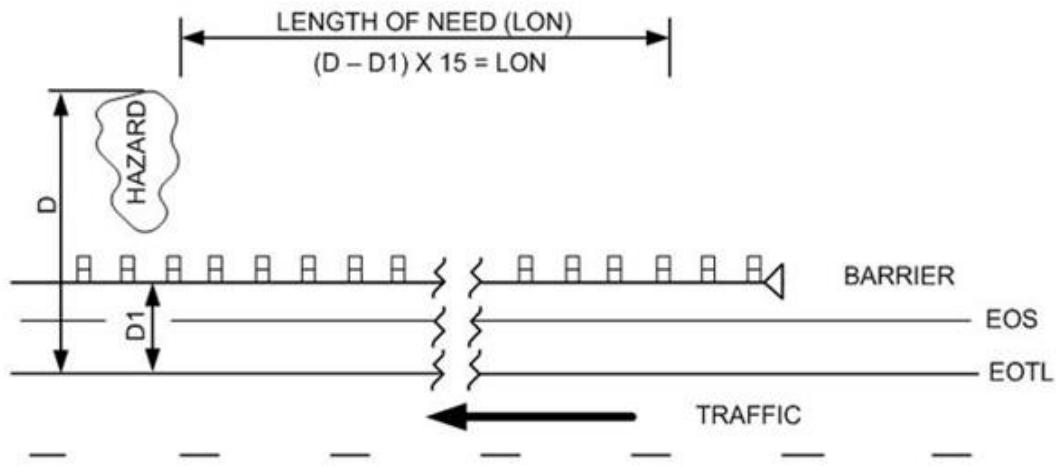
$D$  = Distance from the back of the hazard to the EOTL
