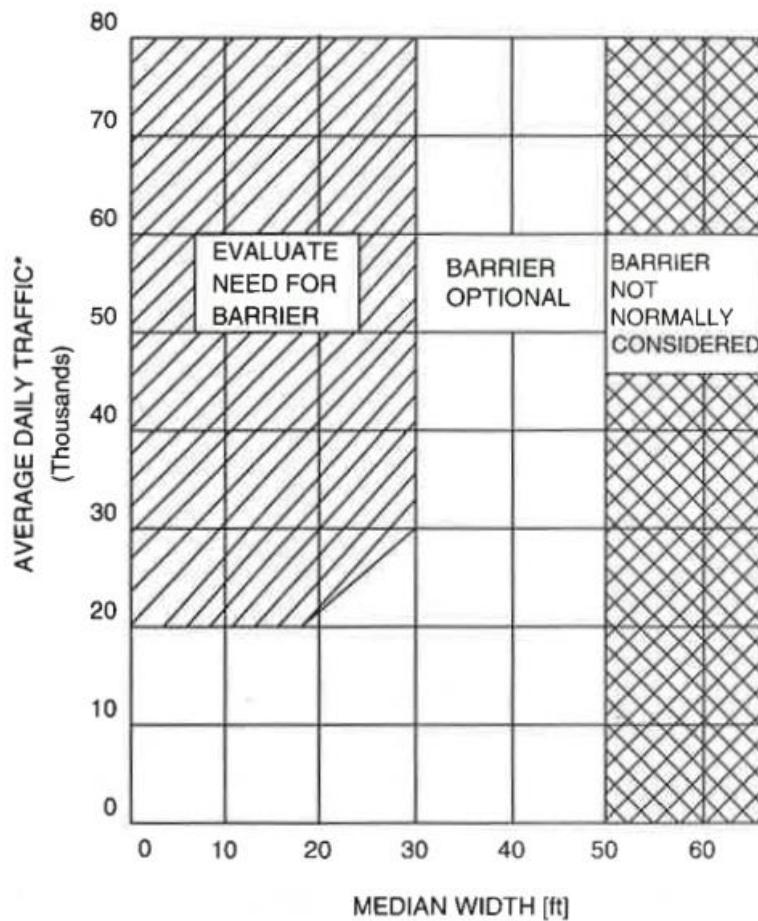
**Figure 4: Guidelines for Median Barrier on High Speed, Fully Controlled-Access Roadways
