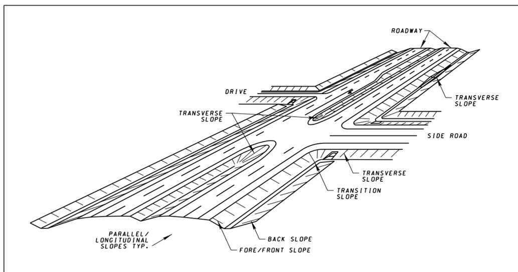
**Figure 1: Roadside Slopes (Adapted from Figure 3-1 of the RDG)**
