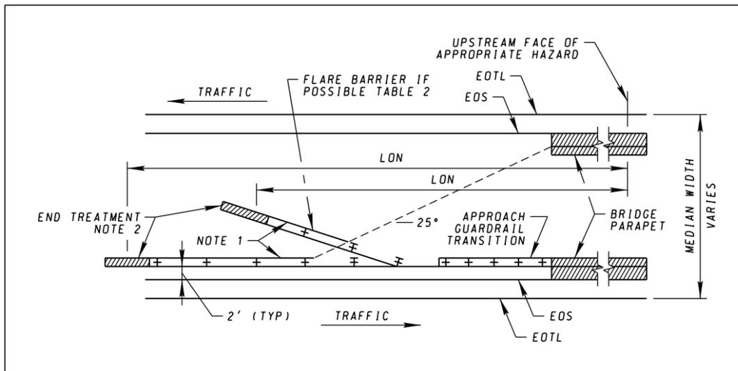
*Note 1: If the back of the barrier is within the “Barrier Optional” or “Evaluate Need for Barrier” regions of Figure 6-1 of the RDG, a TBWB-MB is required.*
