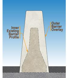
CONSTANT SLOPE MEDIAN BARRIER OVERLAY DETAIL EXISTING JERSEY OR F-SHAPE
