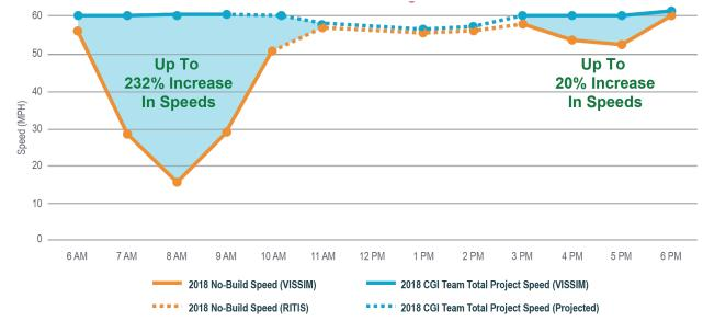
Figure 3.8: Outer Loop Average Speed—US 1 to Cromwell Bridge Road (2018)
