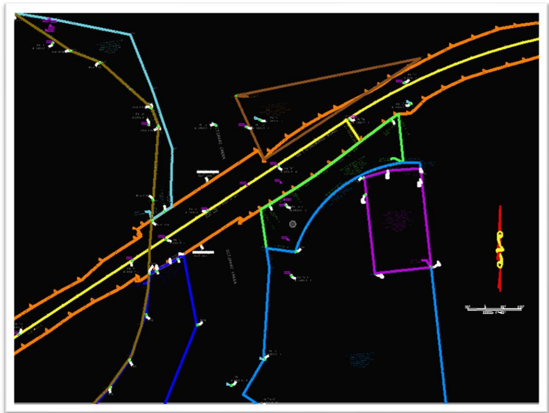
Exhibit 25 - Mosaic example showing the base line (yellow), right of way (orange), parcels (multiple distinct colors), and north arrow in a way so that both the field crew and surveyor can easily identify them
