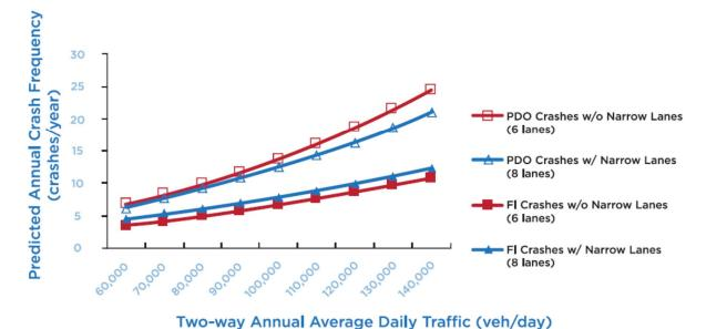
**Figure 19. Graph.** Predicted Crash Frequency With and Without Narrow Lanes and Narrow Shoulders (Conversion from 6-lane Freeway to 8-lane Freeway).
