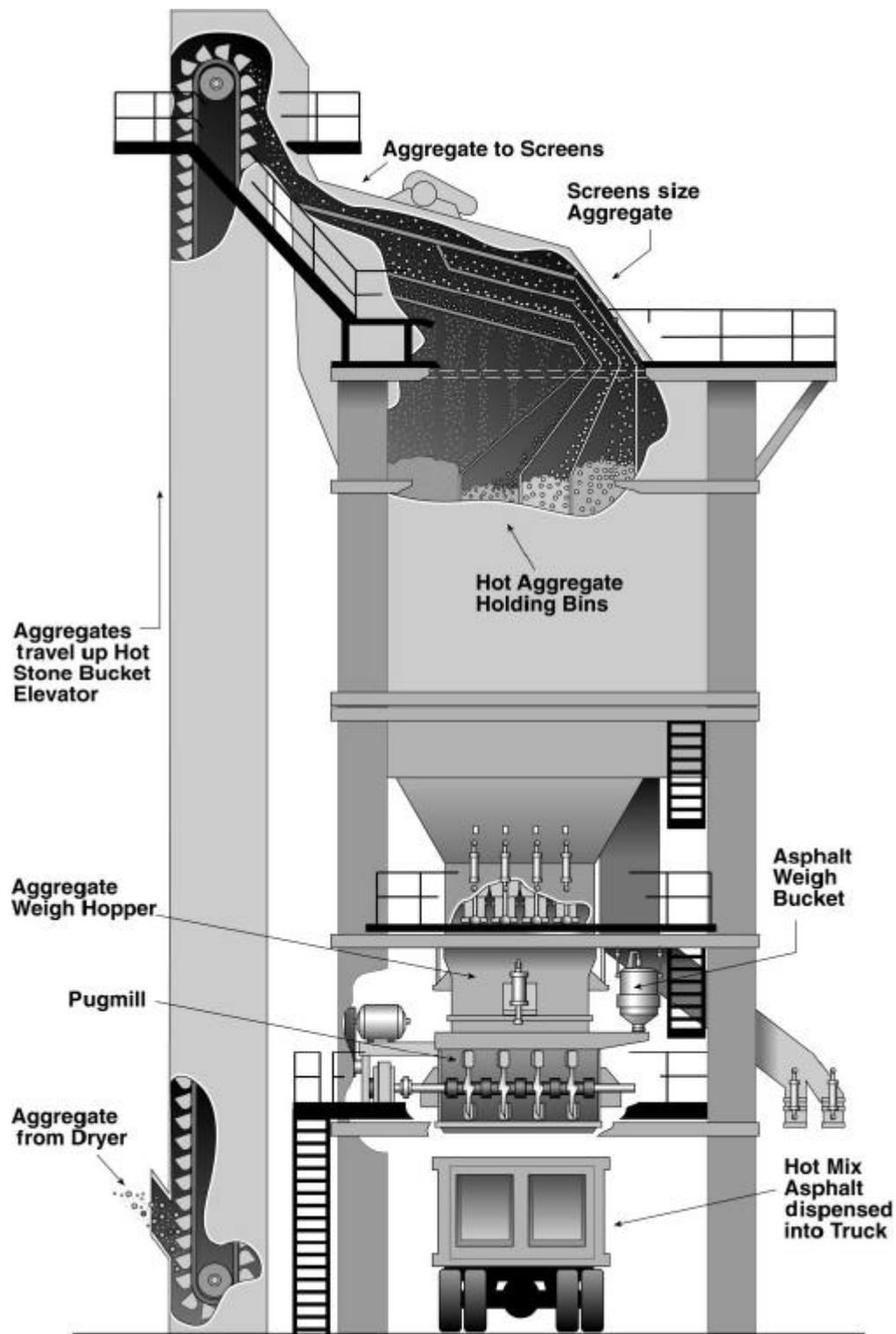
Figure 2.3 Flow of material in batch tower.
