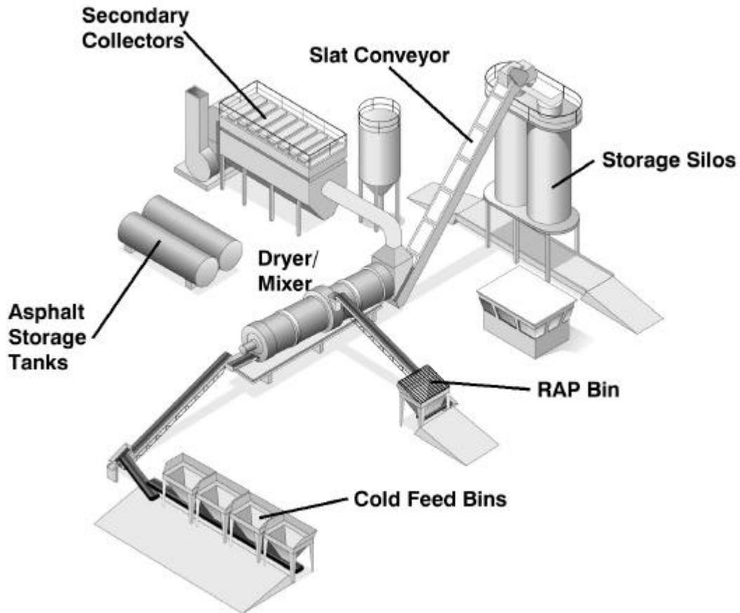
Figure 2.6 Typical "drum-mix" (continuous-flow) facility.
