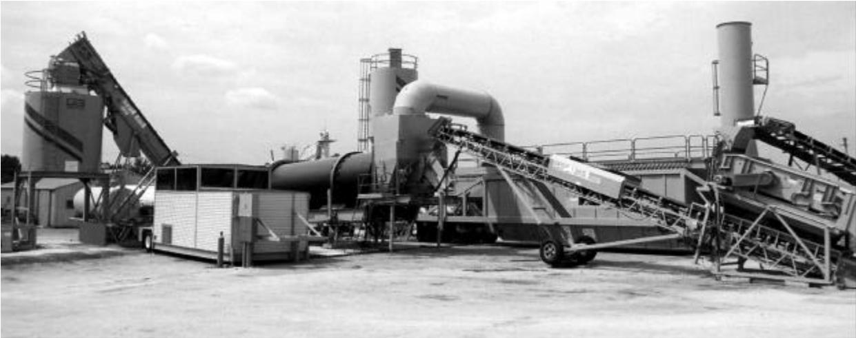
Figure 2.10 Modern counter-flow drum-mix facility.
