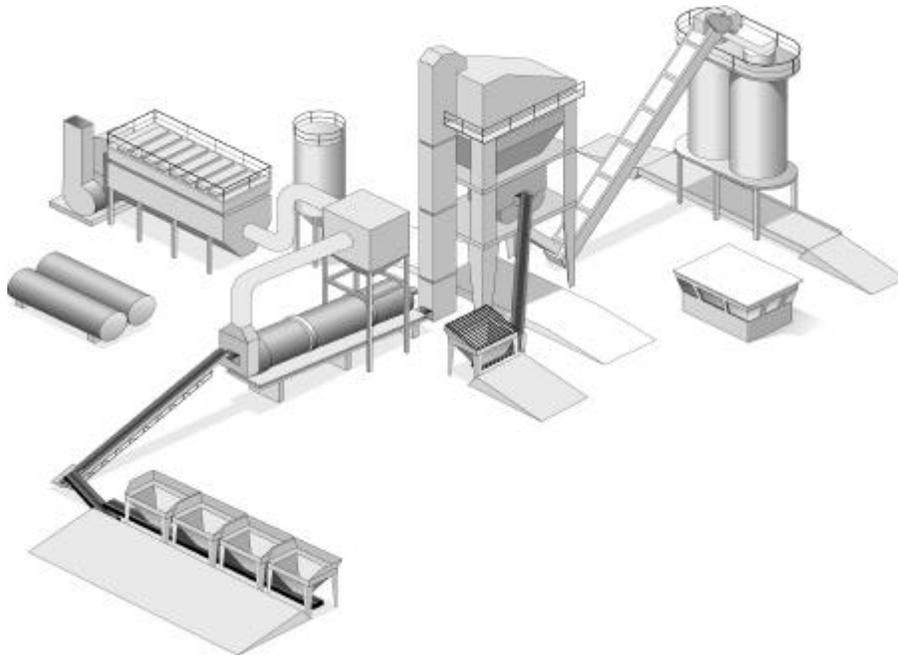
Figure 2.1 Typical asphalt batching style plant.
