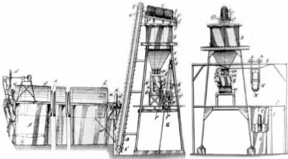
Figure 2.2 Warren Brothers patent drawing for batch plant.
