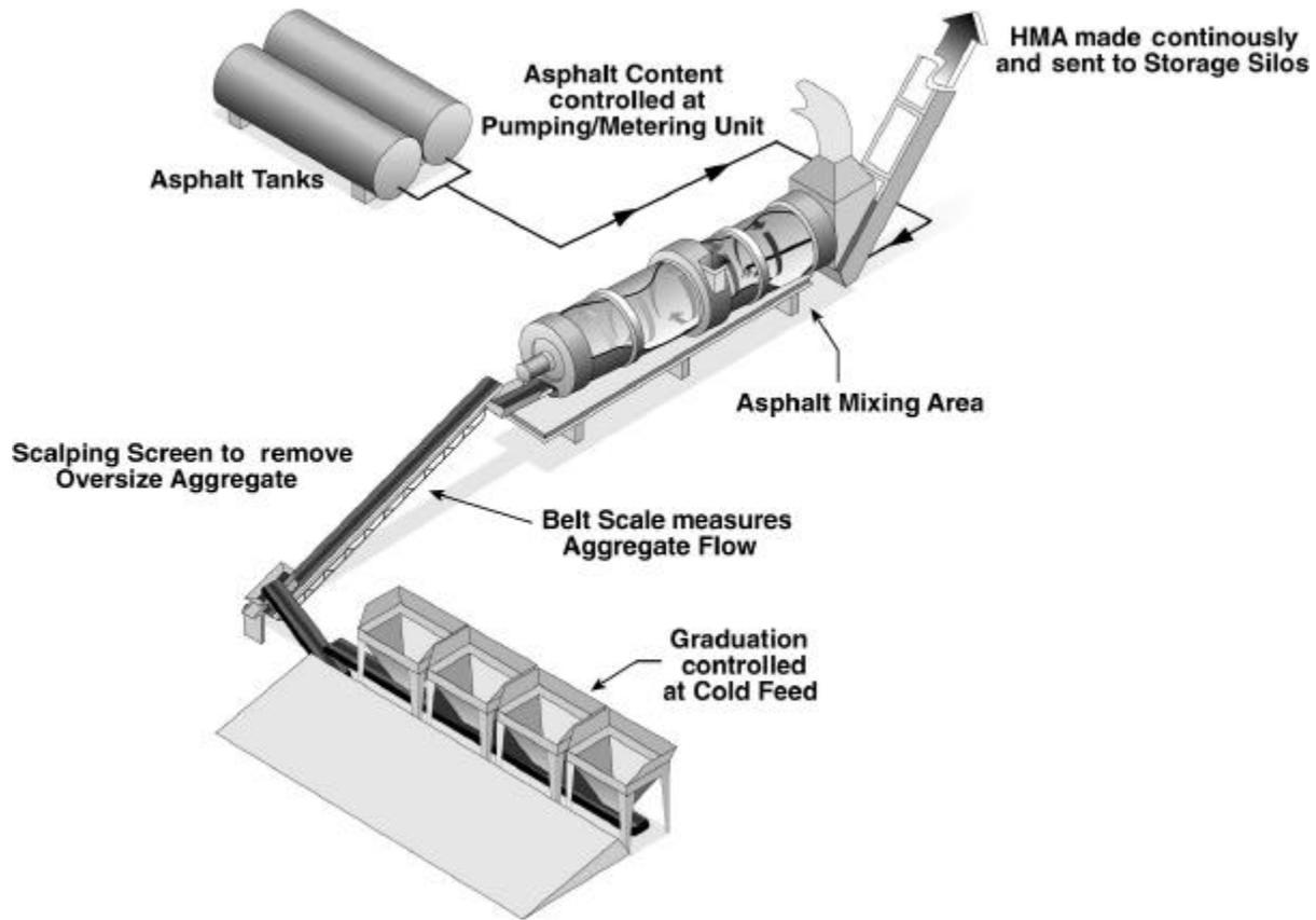
Figure 2.7 Flow of material through a "drum-mix" (continuous flow style facility).
