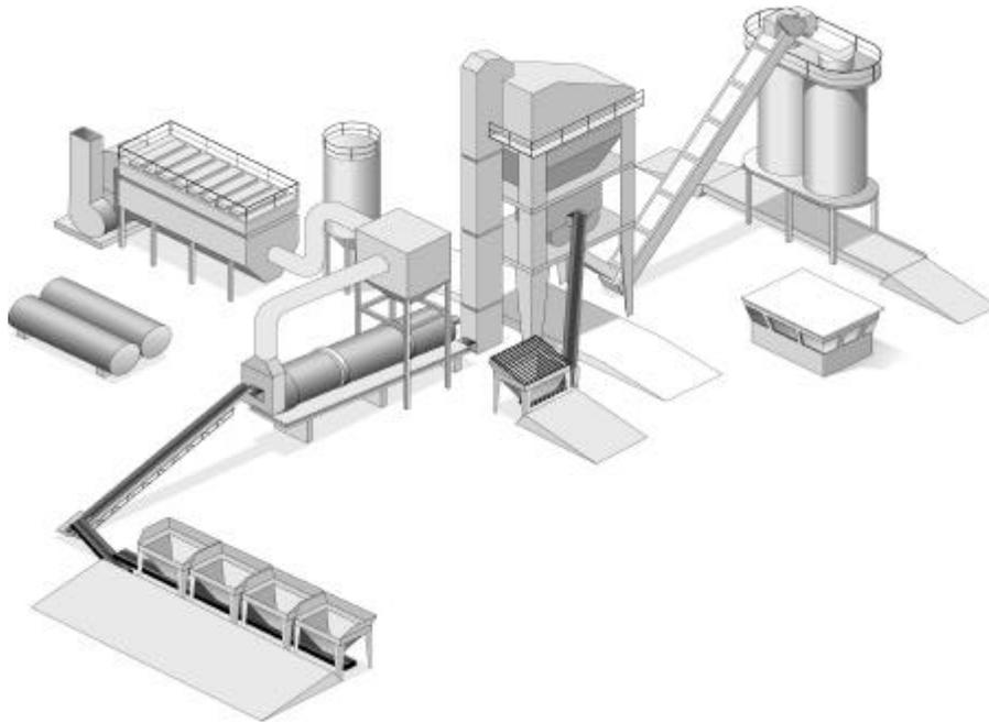
Figure 2.1 Typical asphalt batching style plant.
