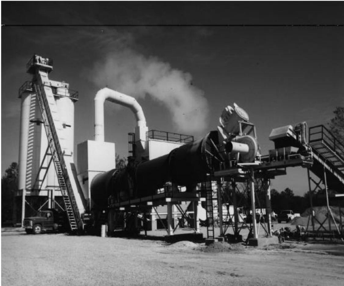
Figure 2.8 Modern parallel-flow drum-mix facility.
