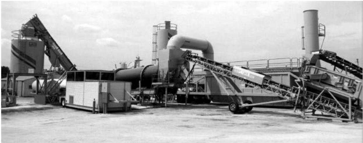
Figure 2.10 Modern counter-flow drum-mix facility.
