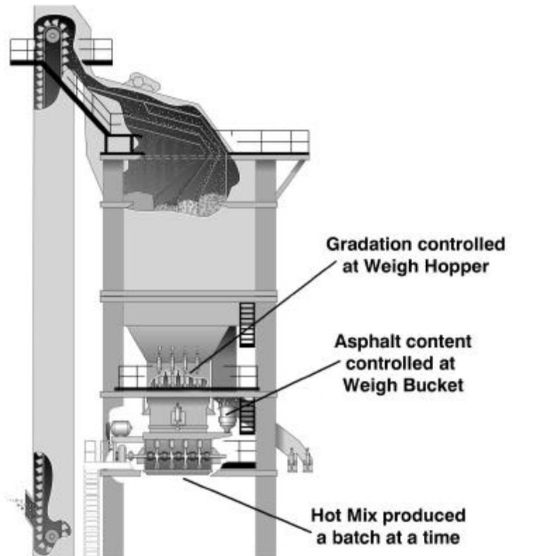
Figure 2.4 Gradation and asphalt control in batch plant.
