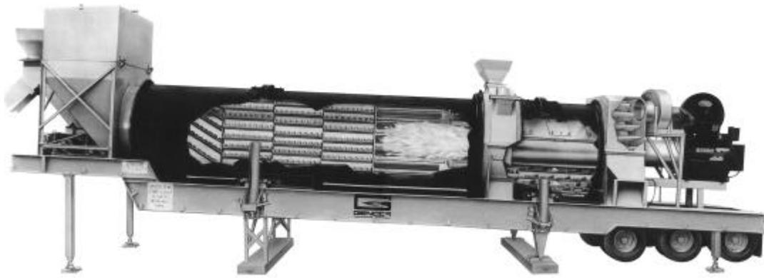
Figure 5.6 Counter-flow drum-mixer.
