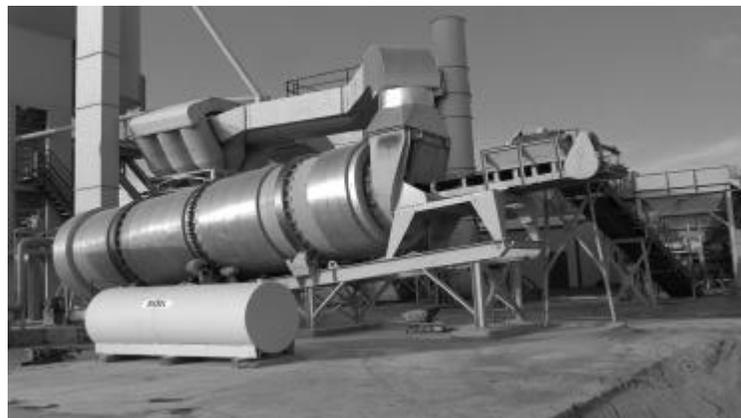
Figure 5.14 Counter-flow dryer with insulation.
