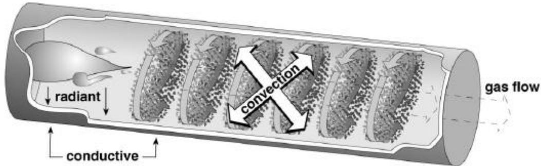
Figure 5.13 Three types of heat transfer in an aggregate dryer.
