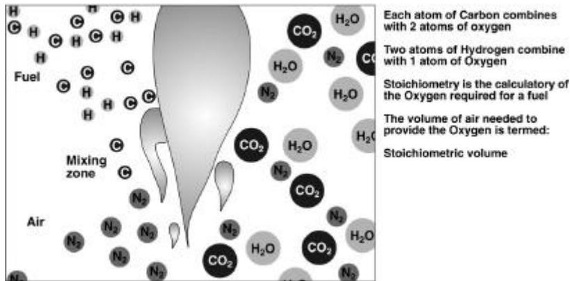
Figure 5.19 Combustion chemistry.
