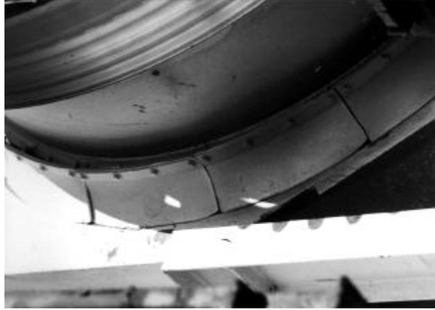
Figure 5.51 Tramp air being drawn in around entry end of counter-flow dryer.
