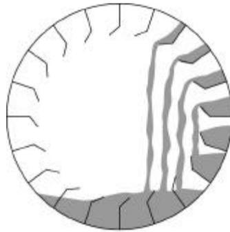
Figure 5.38 Material pitches short due to slow rotational speed.
