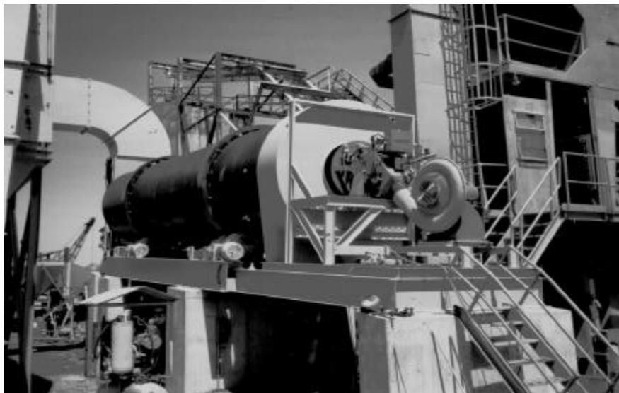
Figure 5.26 Older dryer with new combustion chamberless burner.
