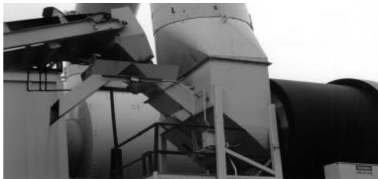
Figure 5.44 Fixed chute entry to dryer with vibrator on chute.
