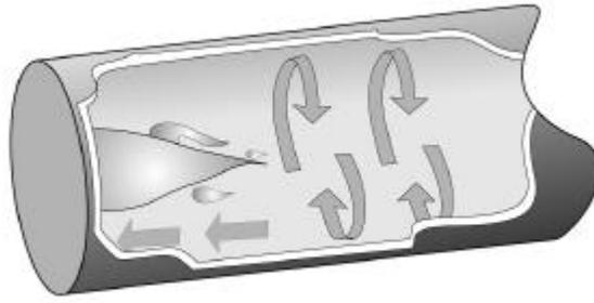
Figure 5.36 Gravity aids movement of aggregate through dryer.
