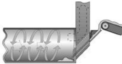
Figure 5.43 Typical fixed chute entry.
