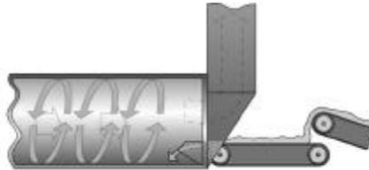
Figure 5.47 Typical slinger feed entry.
