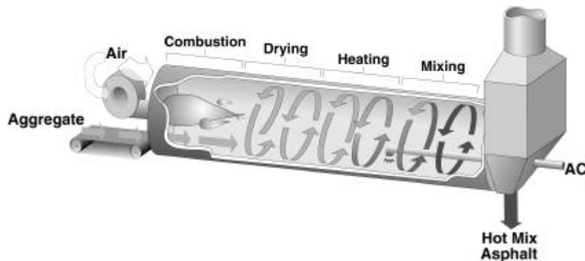
Figure 5.32 Combustion, drying, heating and mixing zones in a parallel-flow drum-mixer.
