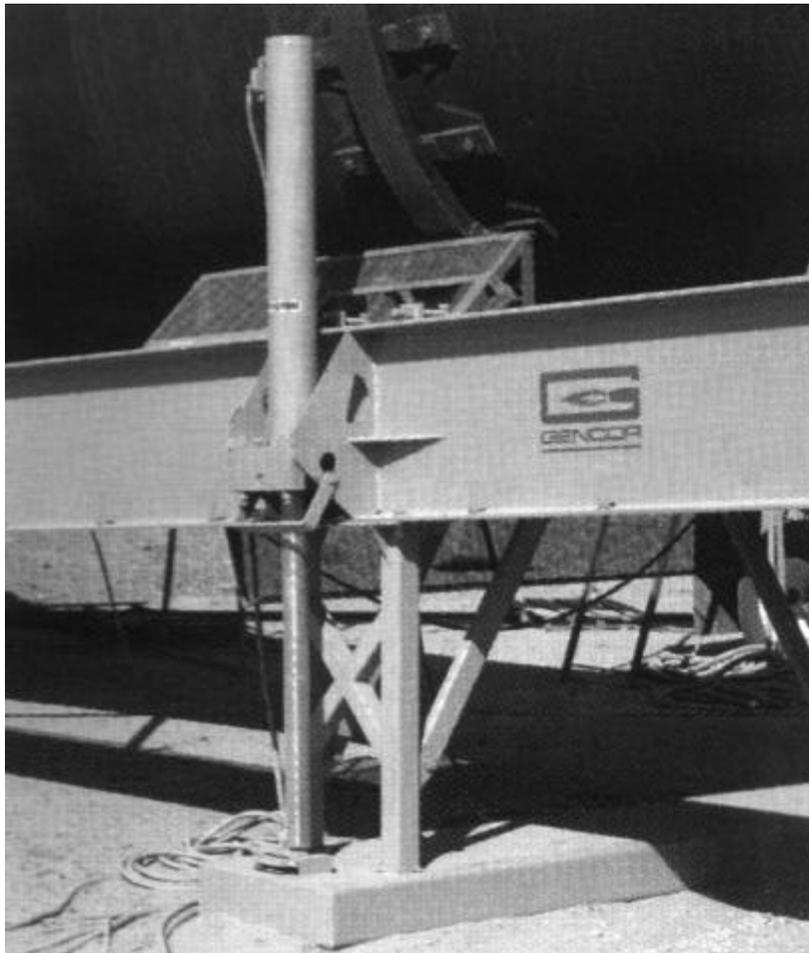
Figure 5.37 Hydraulic slope adjustment support on a portable plant.
