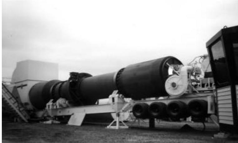
Figure 5.4 Parallel-flow drum-mixer.
