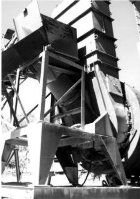
Figure 5.46 Rotating chute entry to dryer.
