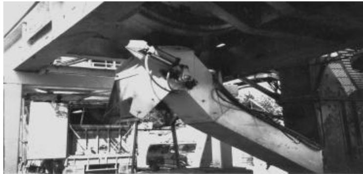
Figure 5.57 Two-way discharge chute.
