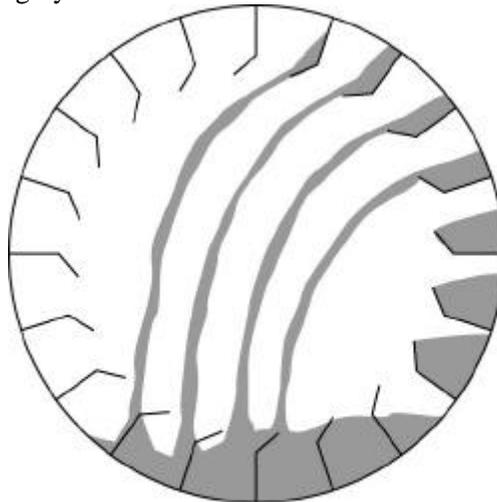
Figure 5.29 Overveiling – material pitches long.
