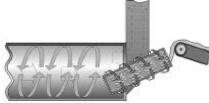
Figure 5.45 Typical rotating chute entry to dryer.
