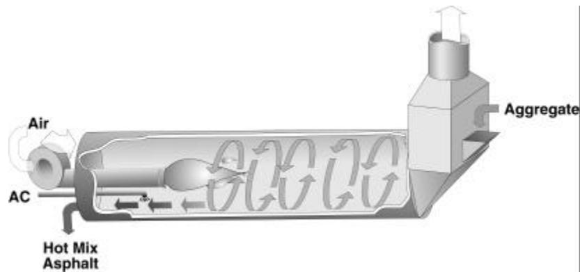
Figure 5.5 Typical counter-flow drum-mixer.
