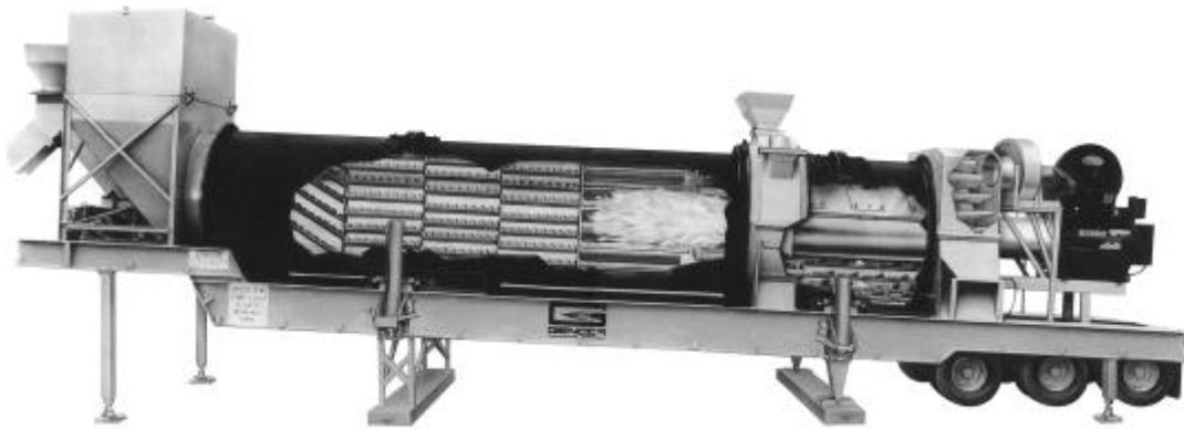
Figure 5.6 Counter-flow drum-mixer.
