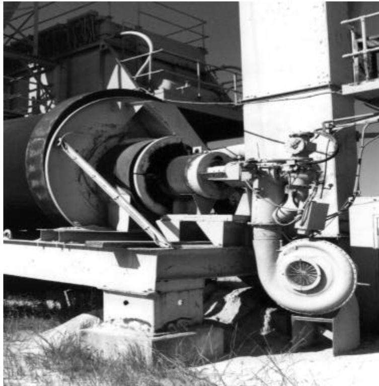
Figure 5.25 Older burner with combustion chamber.
