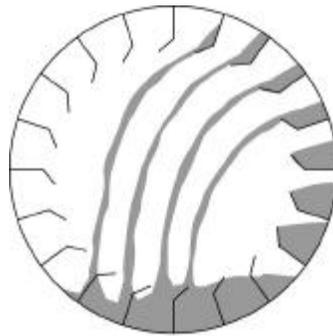
Figure 5.39 Material pitches long due to rotational speed.
