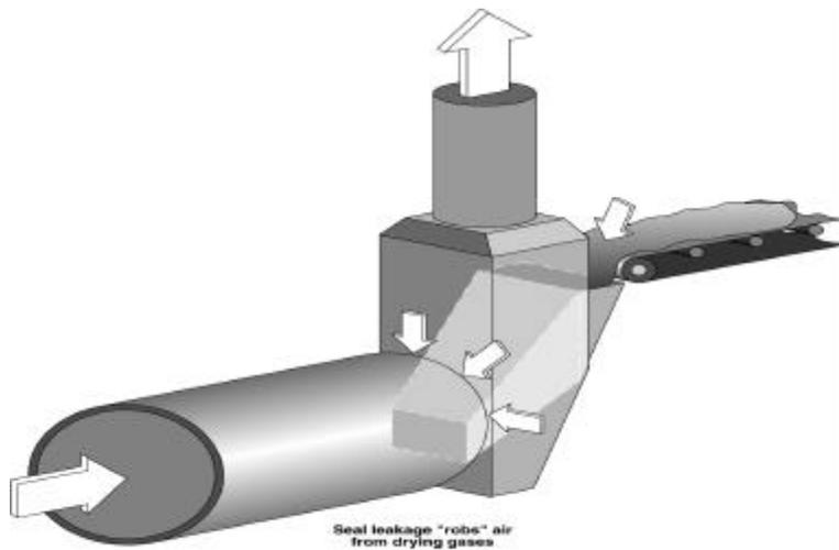
Figure 5.49 Belting type dryer seal.
