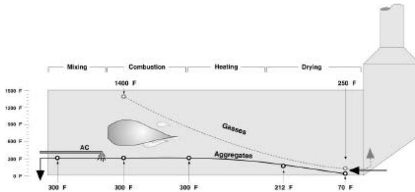
Figure 5.35 Temperature profile of counter-flow drum mixer drying virgin aggregates.
