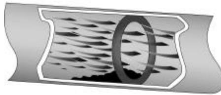
Figure 5.42 Dams increase detention time by holding material in the dryer.
