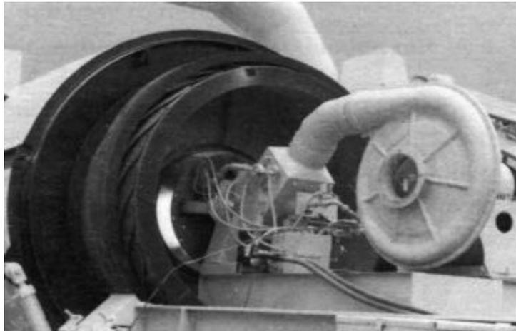
Figure 5.21 Induced draft burner.
