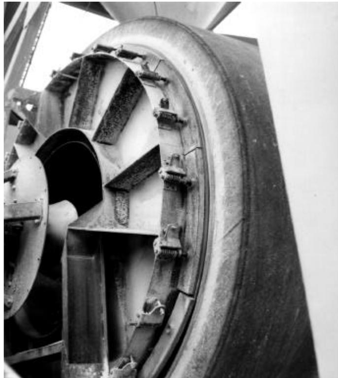
Figure 5.50 Mechanical type dryer seal.
