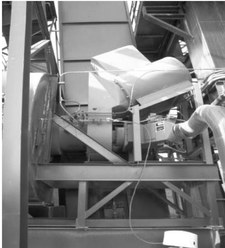
Figure 5.23 Total air burner.
