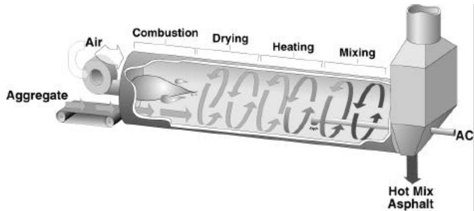
Figure 5.8 Parallel-flow drum-mixer zones.
