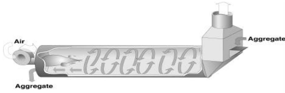
Figure 5.1 Typical counter-flow dryer.
