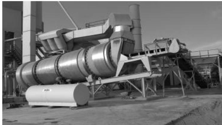
Figure 5.14 Counter-flow dryer with insulation.
