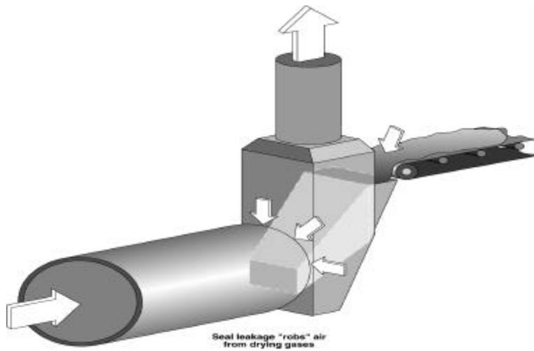
Figure 5.49 Belting type dryer seal.
