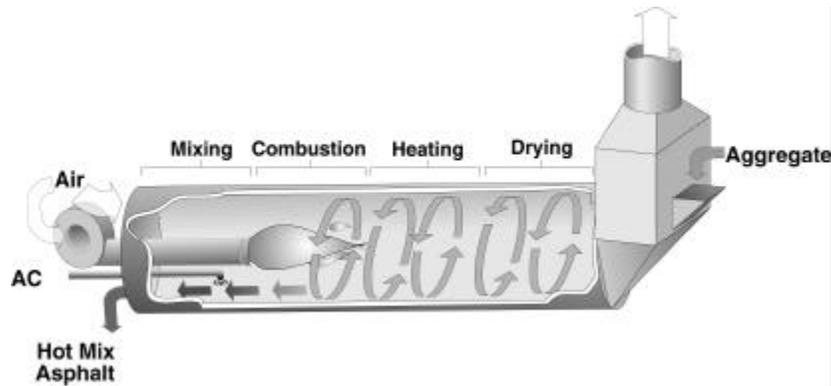
Figure 5.9 Counter-flow drum-mixer zones.
