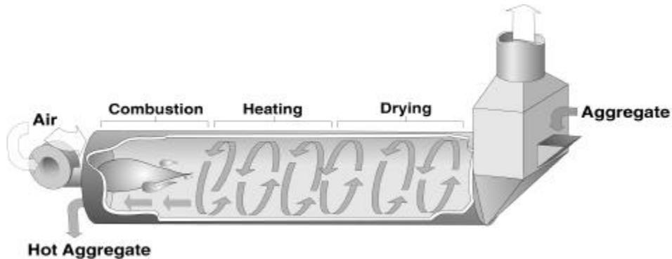
Figure 5.31 Combustion, drying and heating zones in a counter-flow dryer.
