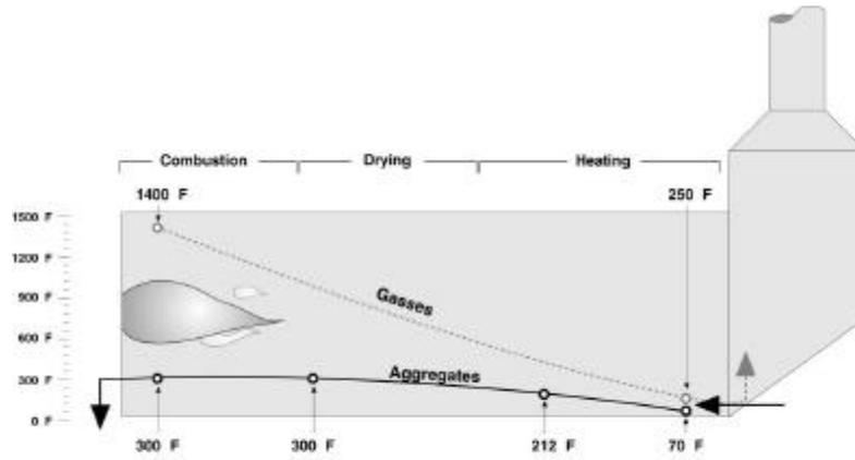
Figure 5.34 Temperature profile of counter-flow dryer drying virgin aggregates.
