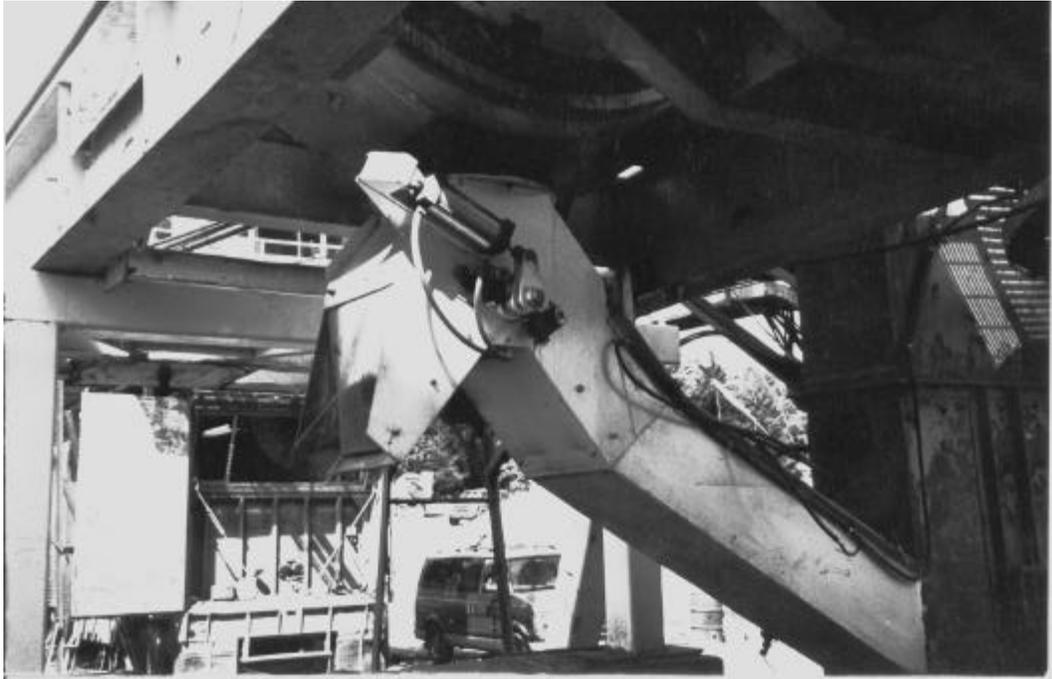
Figure 5.52 Gravity drop chute from dryer.
