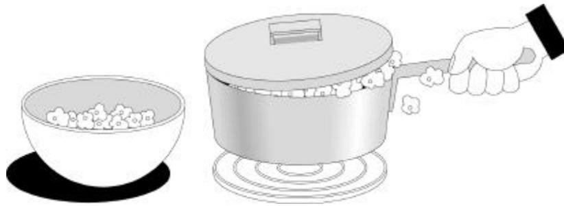
Figure 5.10 Example of conductive heat transfer.
