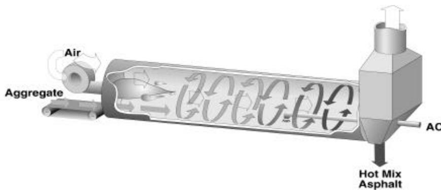
Figure 5.3 Typical parallel-flow drum-mixer.
