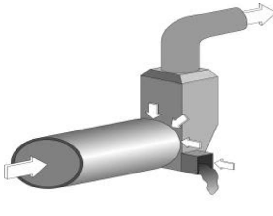
Figure 5.56 Tramp air being drawn in around parallel-flow dryer discharge area.
