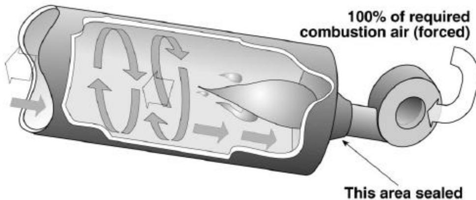
Figure 5.22 Total air burner.
