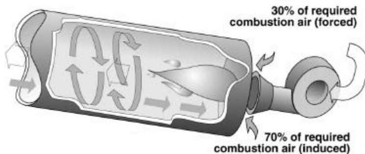
Figure 5.20 Induced draft burner.
