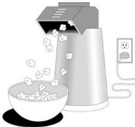
Figure 5.11 Example of convective heat transfer.
