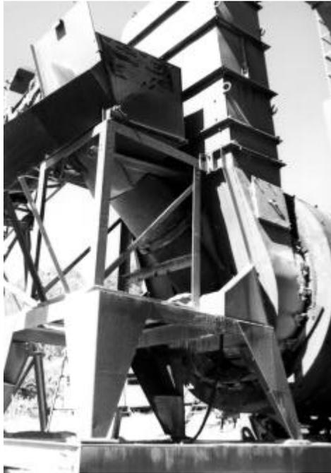
Figure 5.46 Rotating chute entry to dryer.
