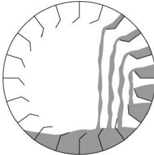
Figure 5.28 Insufficient veiling - material falls too soon.
