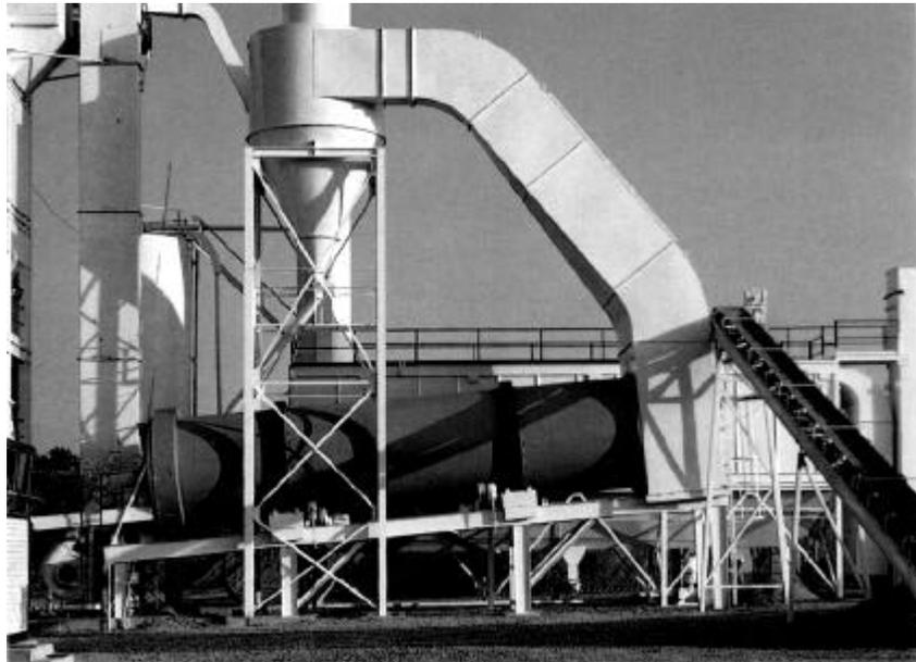
Figure 5.2 Counter-flow dryer on batch plant.
