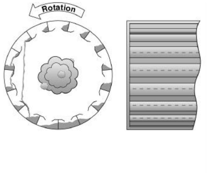
Figure 5.16 Over flame combustion flight.
