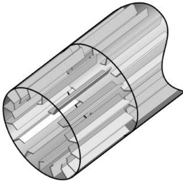
Figure 5.30 Flights in a dryer are "staggered" row to row, to improve veiling.
