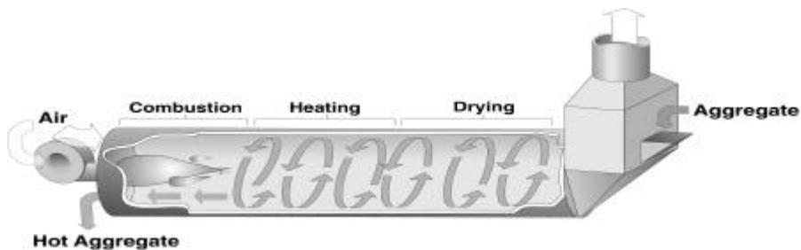
Figure 5.7 Counter-flow batch plant dryer zones.
