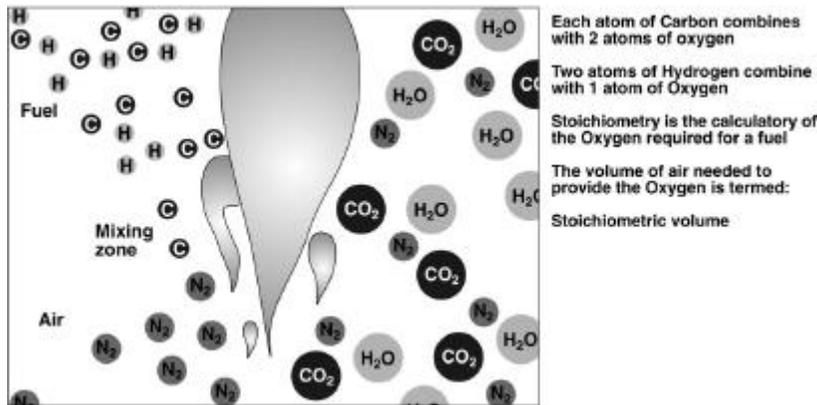
Figure 5.19 Combustion chemistry.
