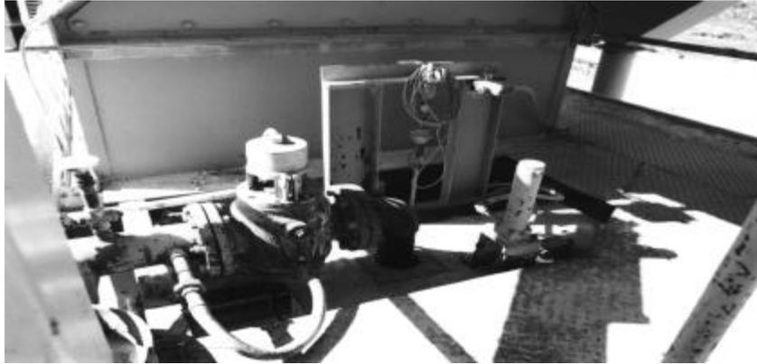
Figure 4.22 Asphalt fill valve on batch tower.
