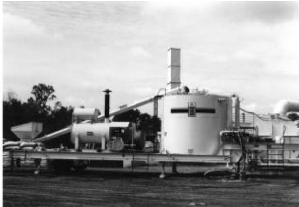
Figure 4.15 Crumb rubber modified asphalt processing system and tanks.
