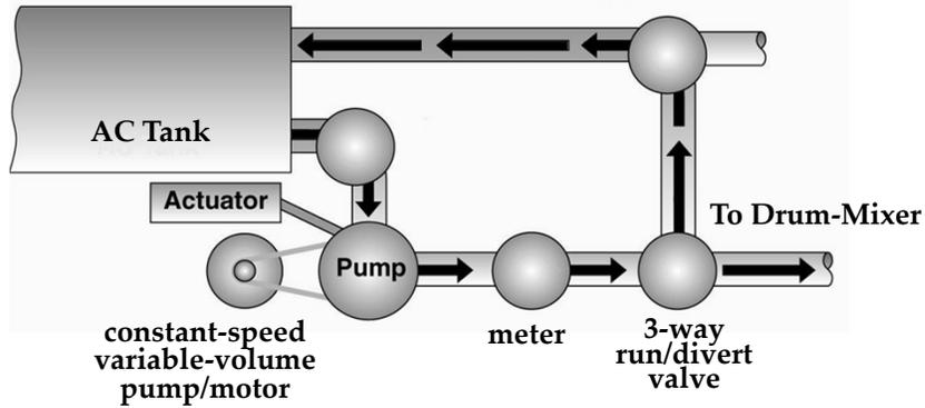
**Asphalt Metering System for drum-mixer plants
