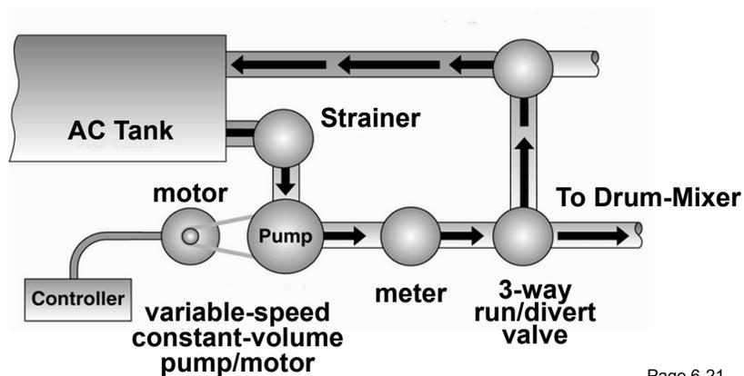
**Asphalt Metering System for drum-mixer plants
