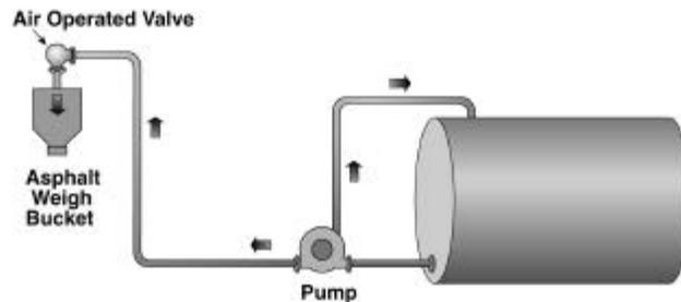
Figure 4.24 Asphalt fill valve on batch tower.
