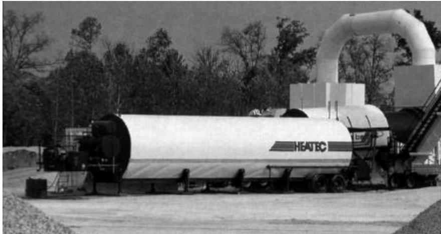
Figure 4.3 Portable asphalt tank.
