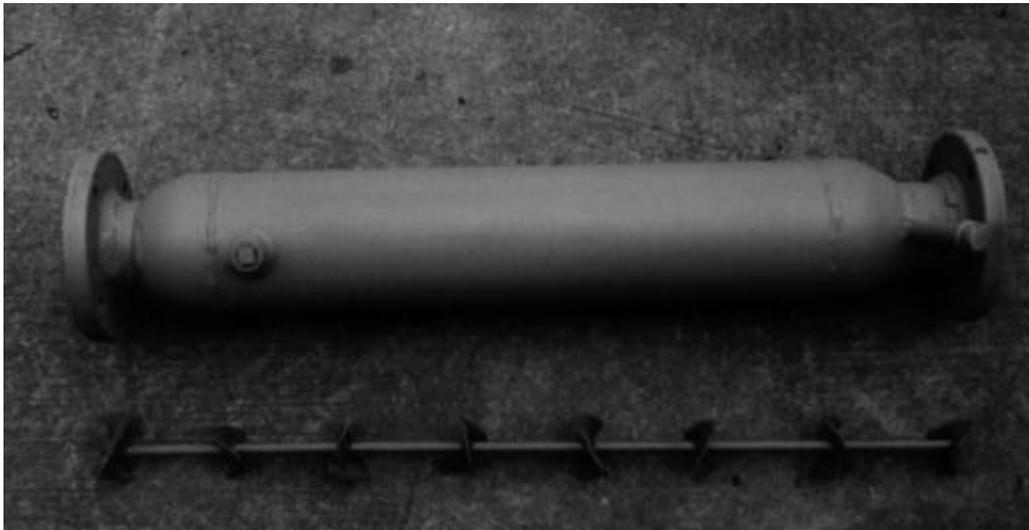
Figure 4.32 Liquid additive static in-line blender.
