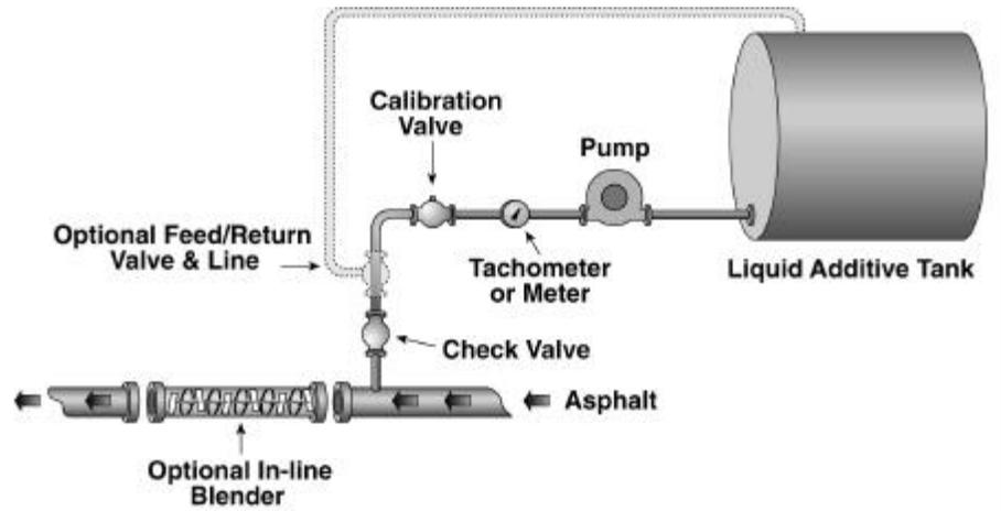
Figure 4.28 Typical asphalt additive tank system.
