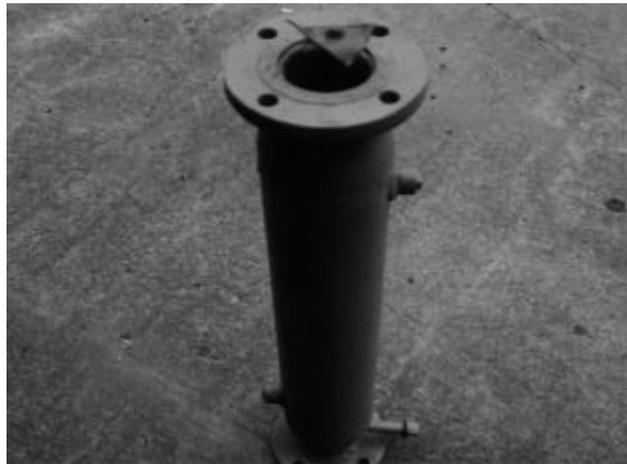
Figure 4.33 Liquid additive static in-line blender.
