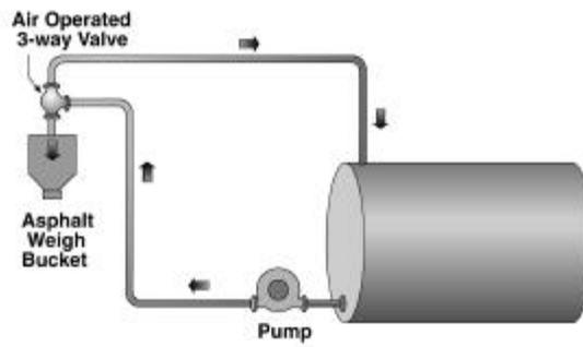
Figure 4.23 Two line asphalt system for batch tower.
