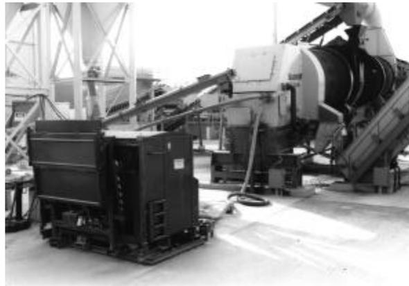
Figure 4.16 Fiber adding system with tank.
