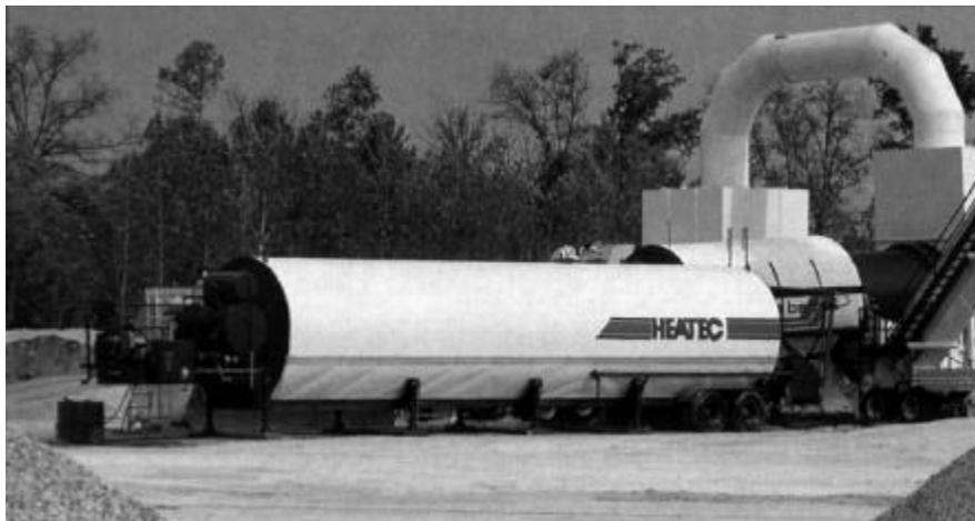
Figure 4.3 Portable asphalt tank.
