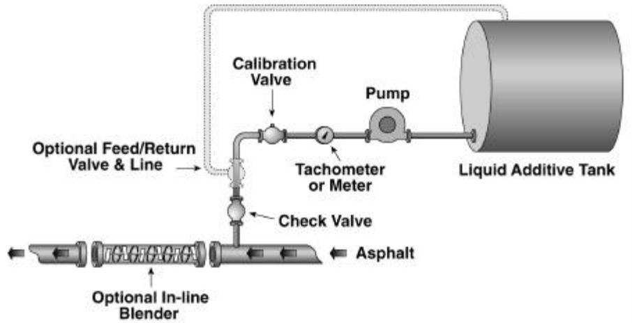
Figure 4.28 Typical asphalt additive tank system.
