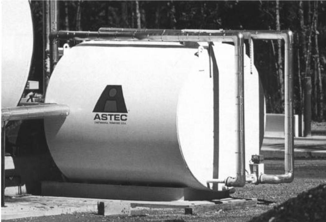
Figure 4.30 Liquid asphalt binder additive tank system.
