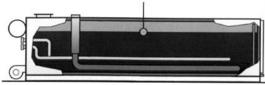
Figure 4.11 Typical direct fired asphalt tank.
