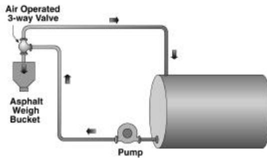
Figure 4.23 Two line asphalt system for batch tower.
