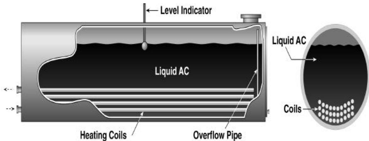
Figure 4.1 Typical horizontal asphalt tank.
