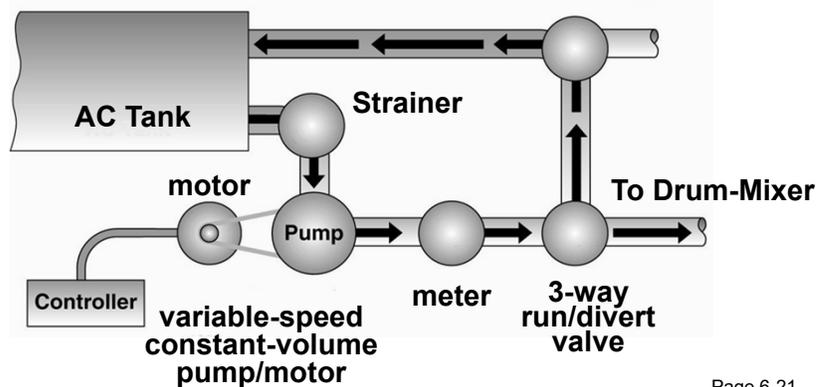
**Asphalt Metering System for drum-mixer plants
