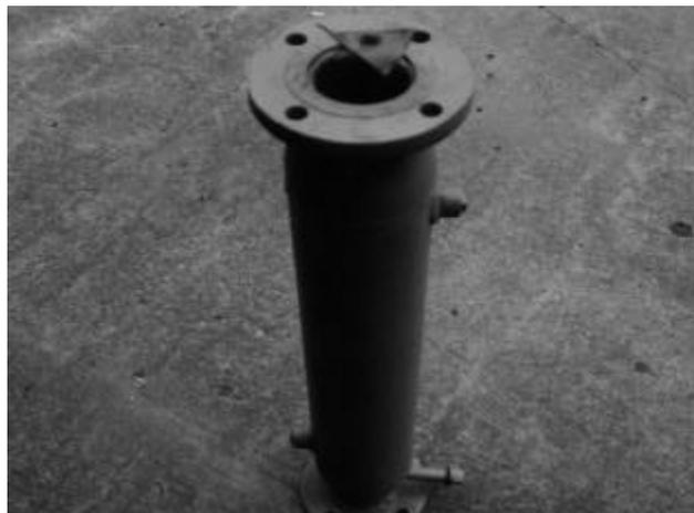
Figure 4.33 Liquid additive static in-line blender.
