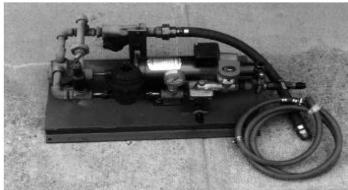
Figure 4.29 Typical liquid additive pumping skid including pump/motor and tachometer.
