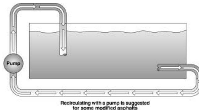
Figure 4.14 Recirculating with a pump is suggested for some modified asphalts.
