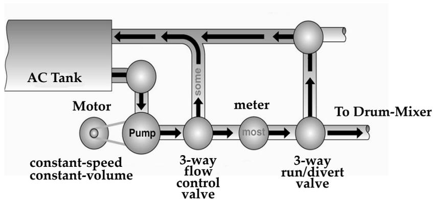
Asphalt Metering System for drum-mixer plants with constant speed constant volume pump and flow control valve
