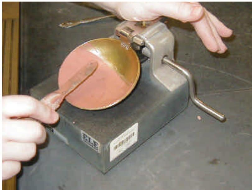
Figure 6 - Spreading Specimen in Liquid Limit Cup
