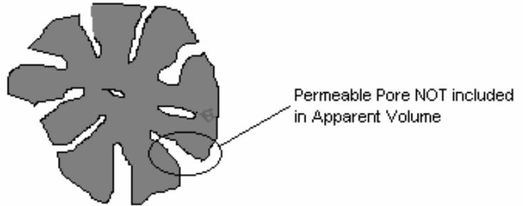
Figure 13 - Diagram of Apparent Specific Gravity
