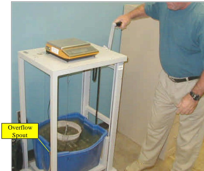
Figure 2 - Coarse Aggregate Gravity Apparatus.
