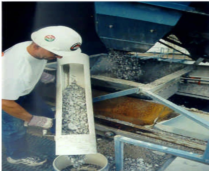
Figure 1 - Streamflow Sampling
