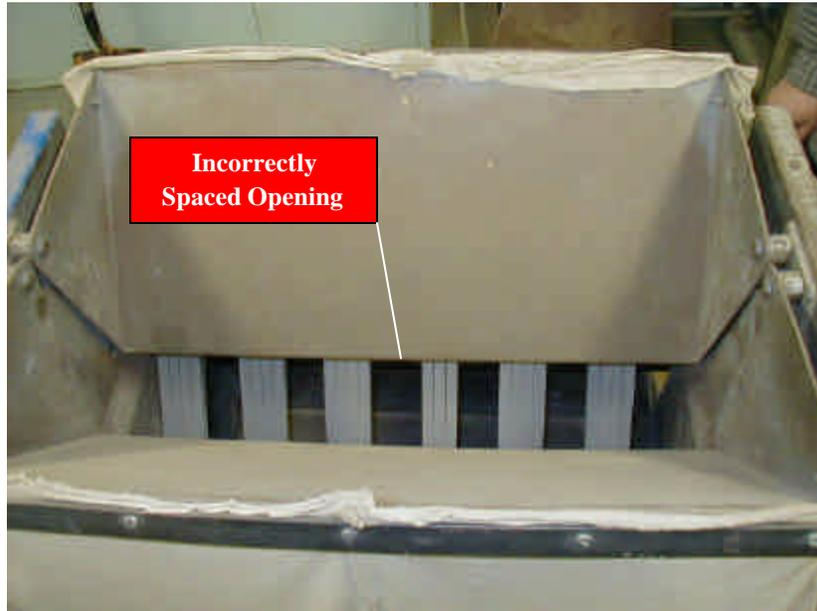
Figure 8 – Incorrect Openings
