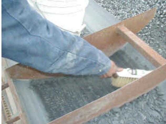
Figure 3 - Cleaning fines from belt.
