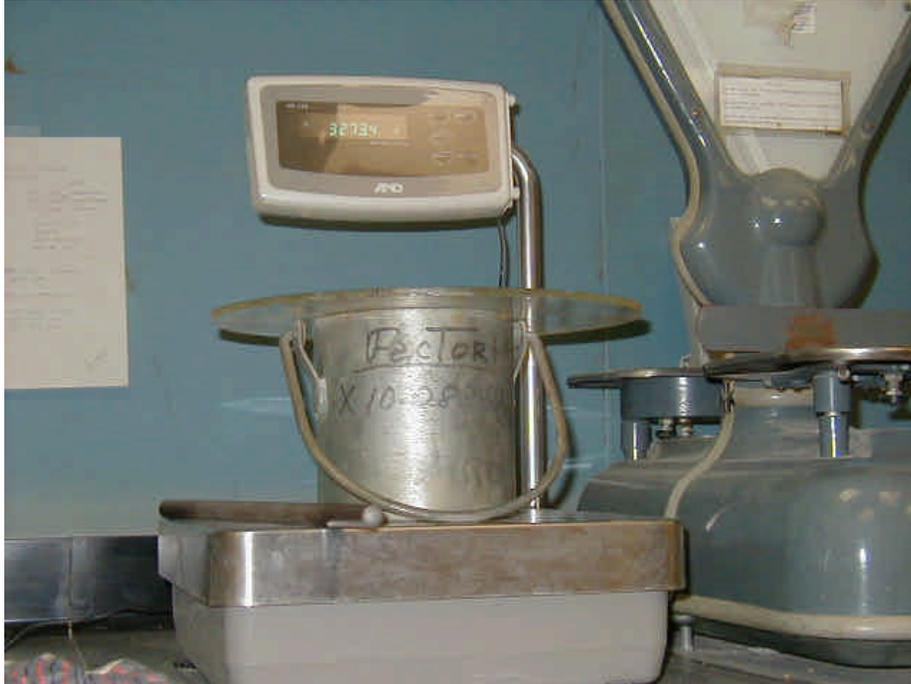
Figure 2 - 1/10 cubic foot measure.
