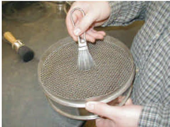
Figure 3 - Use Wire Brush on Coarse Sieves
