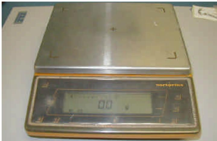
Figure 1 - Balance: conforming to class G5 (AASHTO M 231).
