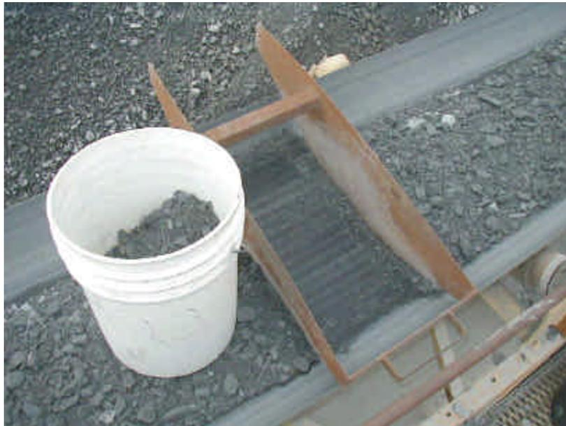
Figure 2 - Belt Cut Using Template
