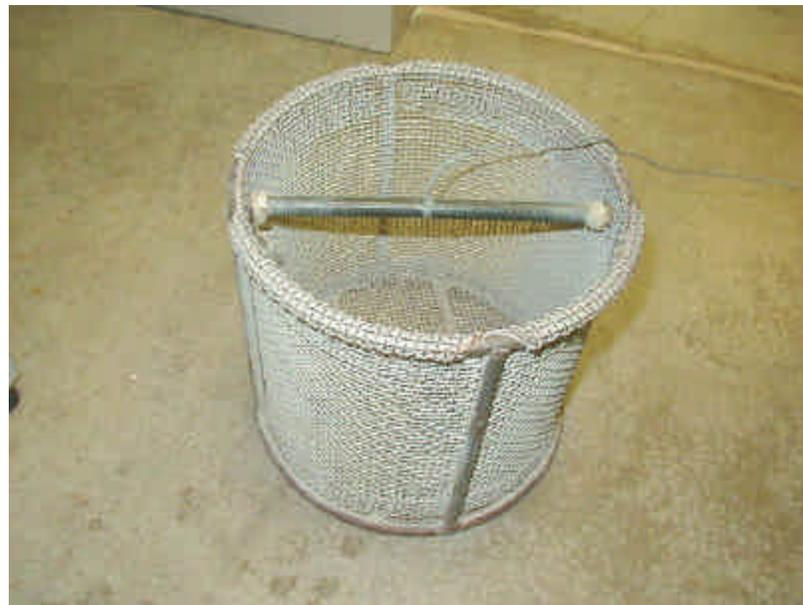
Figure 3 - Sample container: wire basket of 3.35 mm (No. 6) or less mesh wire cloth, with a capacity to contain aggregate with a nominal maximum size of 37.5 mm (1½ in.) or smaller.
