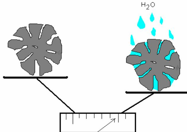
Figure 14. Increase in mass due to absorption of water
