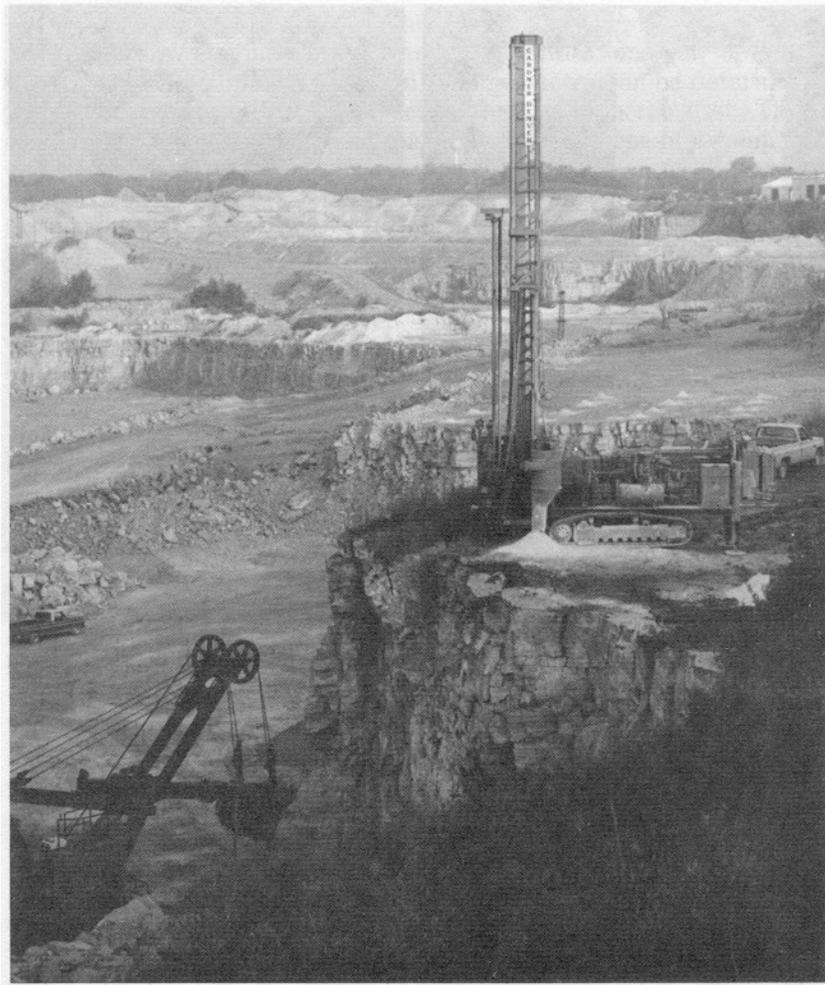
**Fig 4.2 Down The Hole Hammer Drill.**
