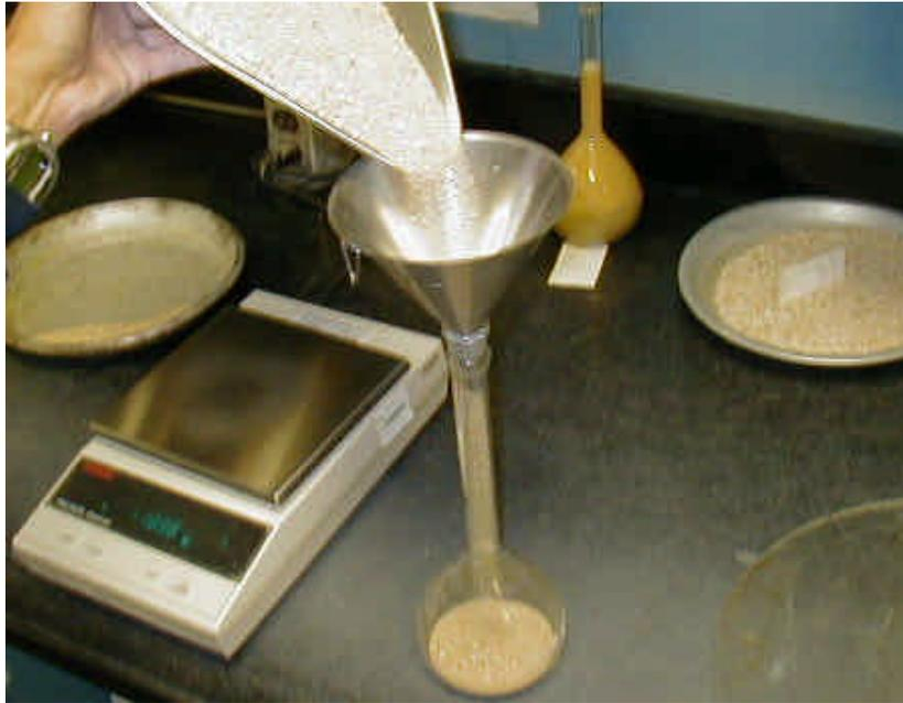
Figure 5 - Pouring sand into the pycnometer once SSD is achieved
