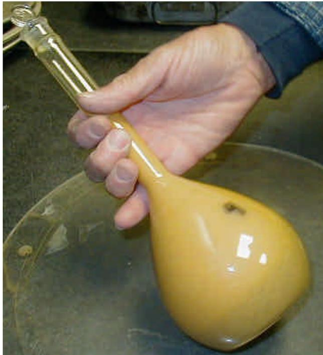
Figure 6 - Rolling of pycnometer
