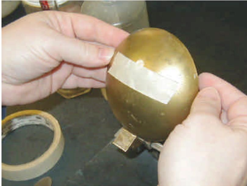
Figure 2 - Placing Masking Tape on Cup Bottom
