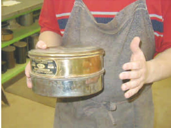
Figure 6 - Checking thoroughness of sieving
