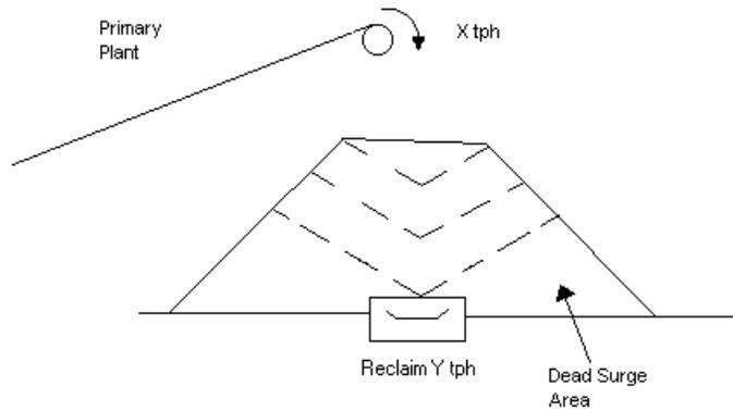
Figure 5-8 Inverted Cone
