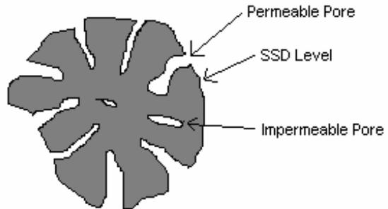
Figure 11 - Diagram of Bulk Specific Gravity
