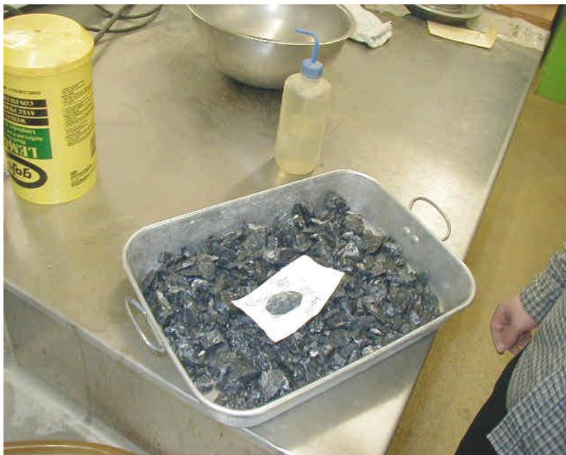
Figure 7 - Washed sample ready for drying.
