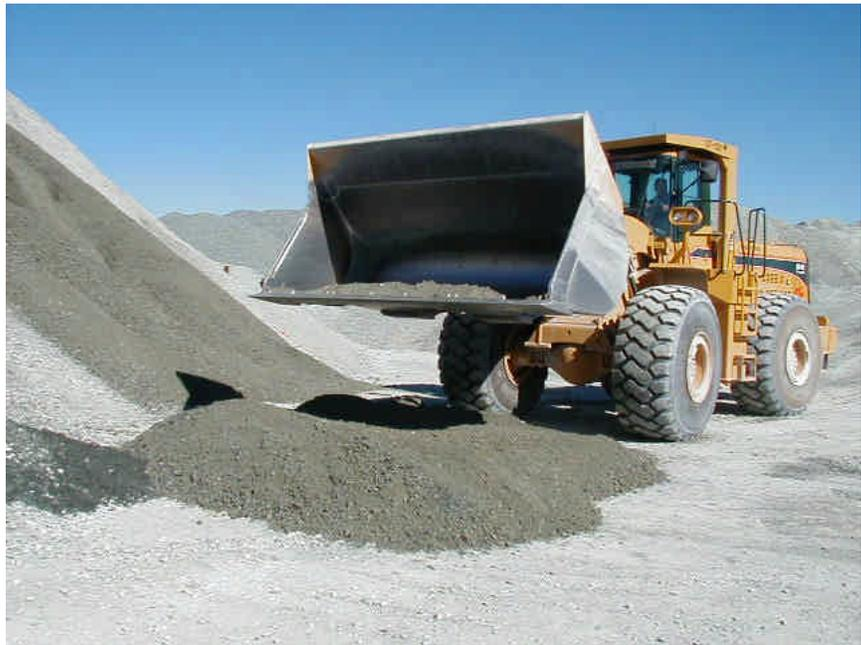
**Fig. 4.5 Front end loader.**
