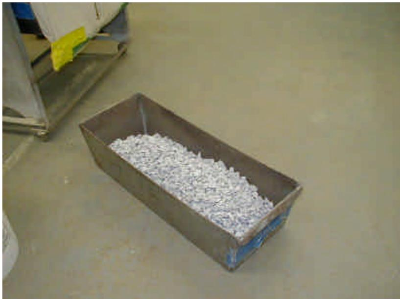
Figure 7 - Proper sized pan to fit splitter
