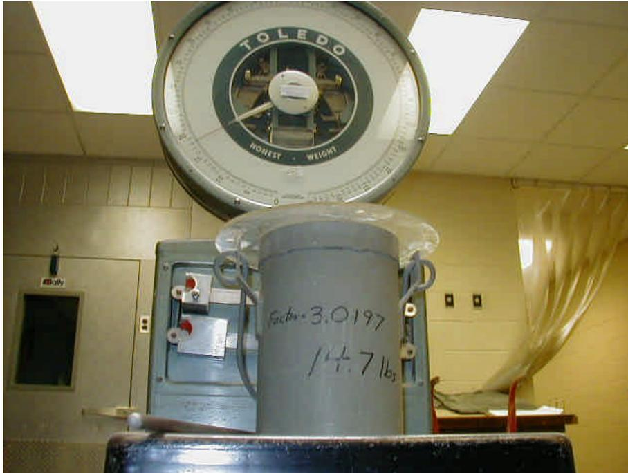
Figure 1 - 1/3 cubic foot measure.
