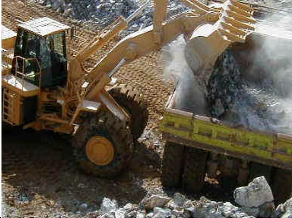
**Fig 4.3 Front end loader loading off road vehicle from muck pile.**
