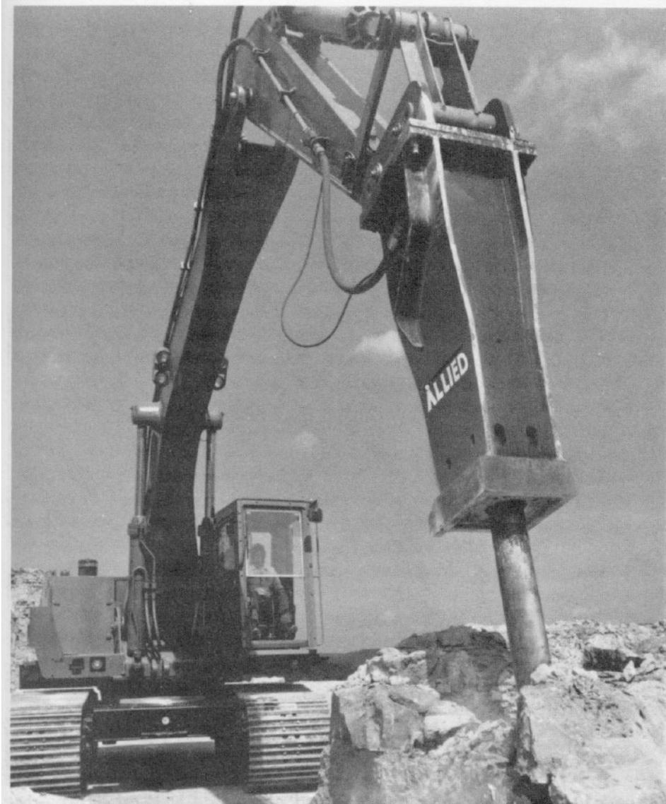
**Fig 4.8 Backhoe mounted hydraulic impact hammer.**
