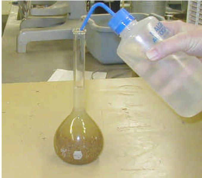
Figure 7 - Filling pycnometer
