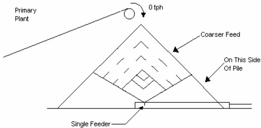
Figure 5-7 Note Alignment of Primary Conveyor and Tunnel
