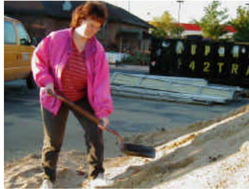
Figure 2 - Stockpile sampling with a square-nosed shovel
