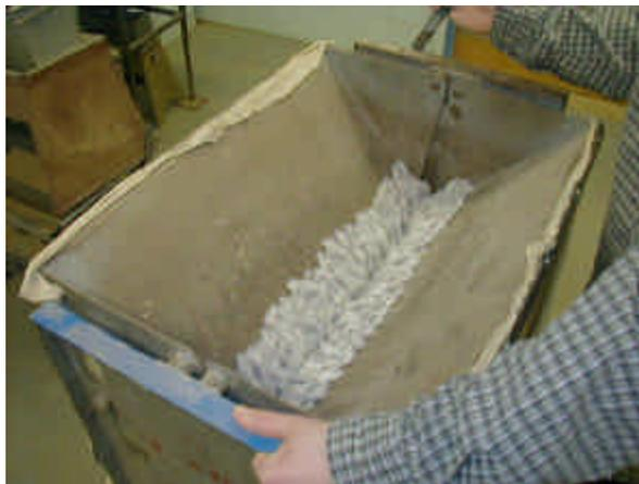
Figure 6b - Mechanical splitter method.
