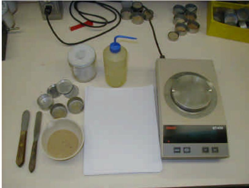
Figure 1 - Equipment for Plastic Limit
