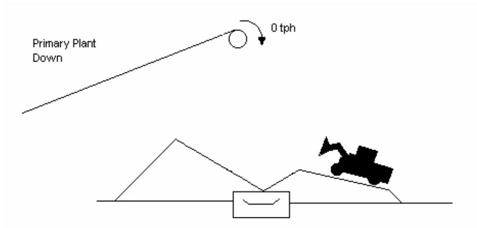
Figure 5-4 Reclaiming Plant Feed From Dead Surge Pile Area
