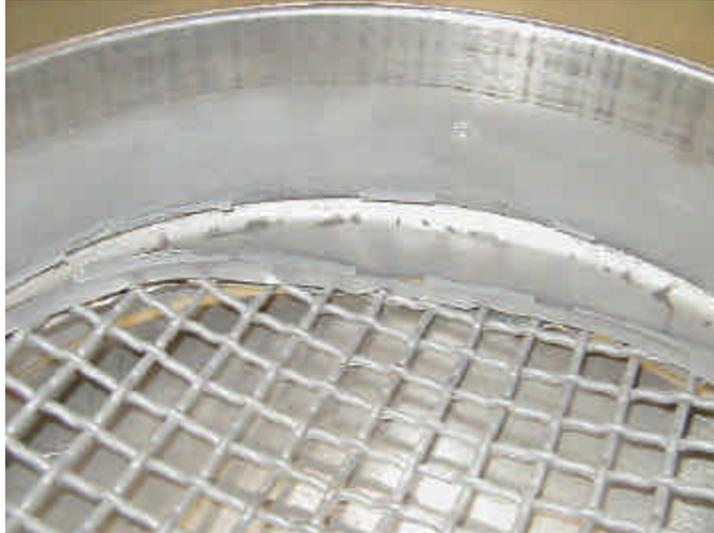
Figure 5 - Cracked Outer Seam
