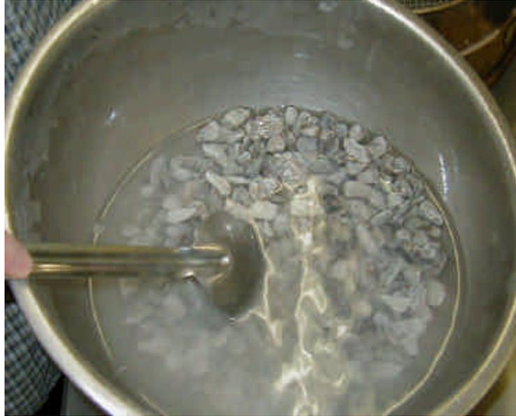
Figure 2 - Wash sample in a large container. Sample should be stirred or agitated in order to suspend the fines in the water.
