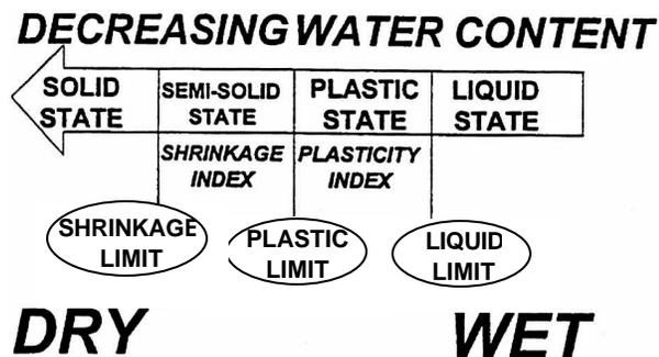
After exceeding the optimum moisture necessary to achieve compaction, material becomes less stable as moisture increases (moving from left to right on the diagram). A material whose moisture content is greater than the Liquid Limit is soft and unstable.
