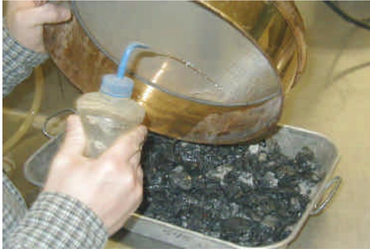
Figure 6 - A water bottle may be used to rinse the material from the 75 mm (No. 200) sieve to the drying pan.
