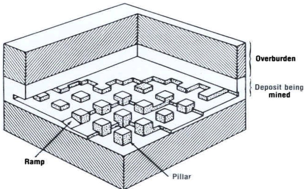
Fig 4.10 Room and pillar mining sequence.
