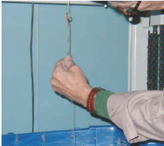
Figure 5 - Suspension apparatus: wire used shall be of smallest practical diameter.
