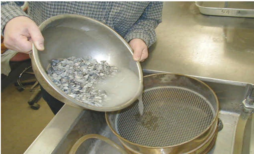
Figure 3 - Fines suspended in the water are washed over a 2.36 mm (No. 8) or 1.18 mm (No. 16) and a 75  $\mu\text{m}$  (No. 200) sieve.
