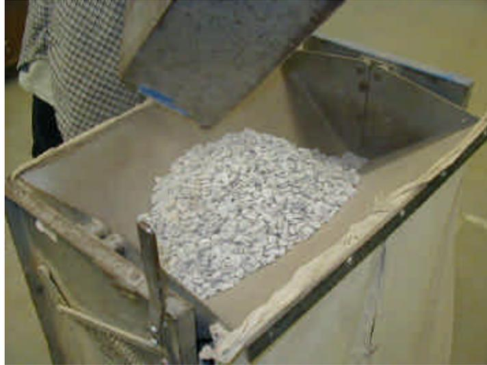
Figure 6 - Sample not spread uniformly in splitter
