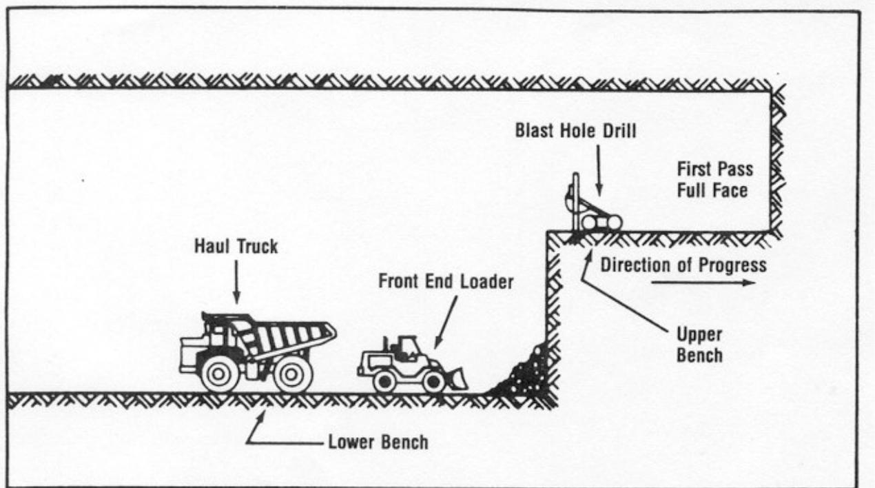
Fig 4.12 Underground bench mining ( cross section )
