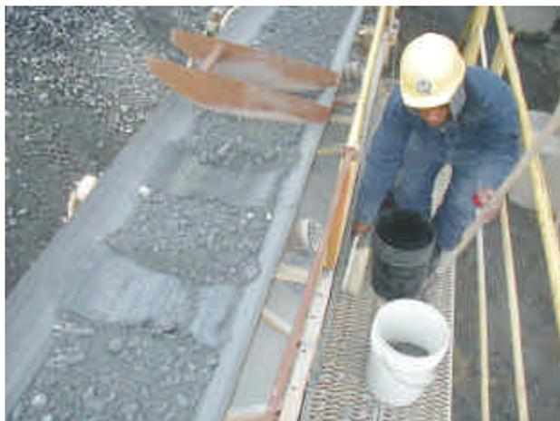
Figure 4 - Three belt cuts to make one sample.
