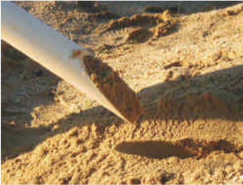
Figure 1 - Stockpile sampling with a sampling tube
