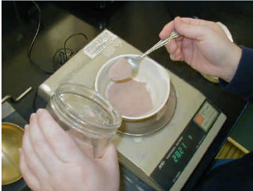
Figure 4 - Weighing Test Specimen
