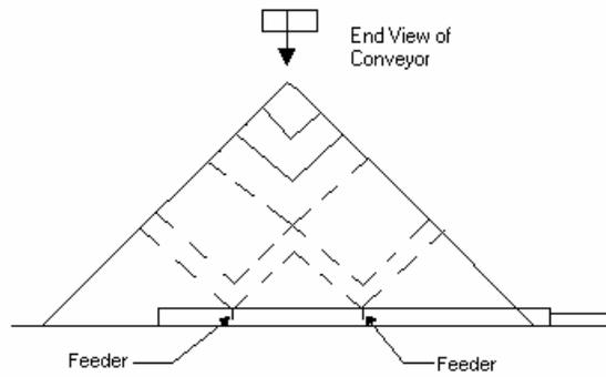
Figure 5-6 Multi Feeders Reclaiming From Surge Pile
