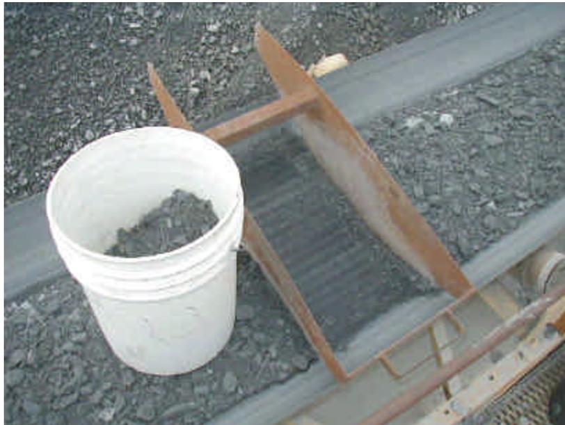
Figure 2 - Belt Cut Using Template
