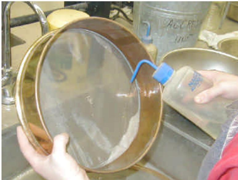
Figure 5 - Material retained on the 75  $\mu$ m (No. 200) sieve after washing
