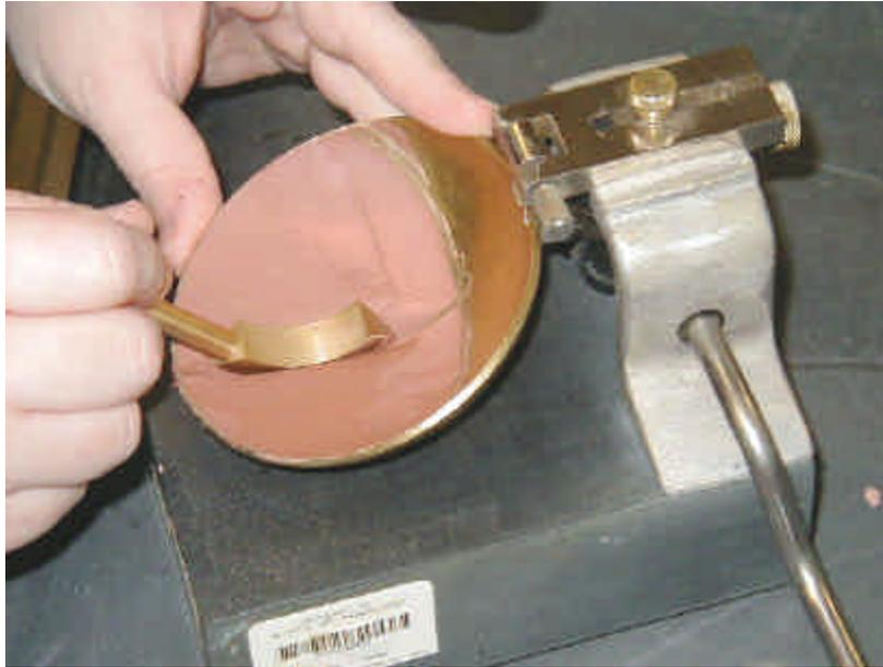
Figure 7 - Grooving the Soil Specimen
