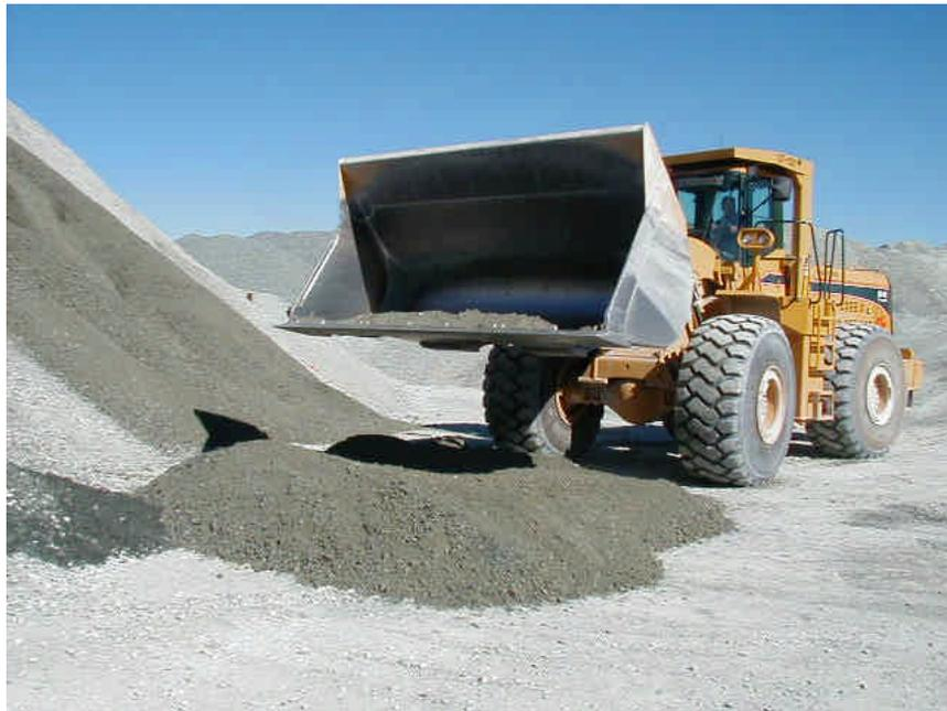
**Fig. 4.5 Front end loader.**
