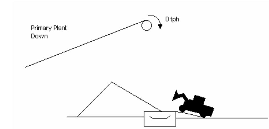
Figure 5-5 Reclaiming Plant Feed From Coarsest Dead Surge Pile Area
