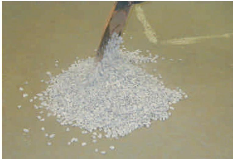
Figure 9 - Improper mixing of sample for quartering
