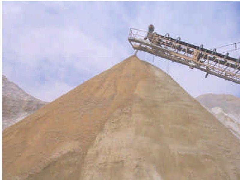
Figure 1 - Flowing Aggregate Stream (Bins or Belt Discharge)
