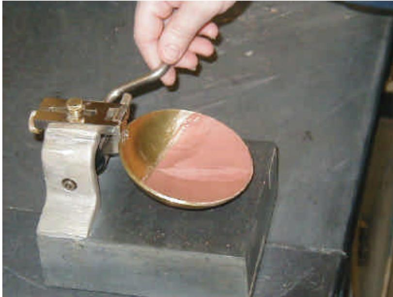
Figure 8 - Applying Blows by Turning the Handle
