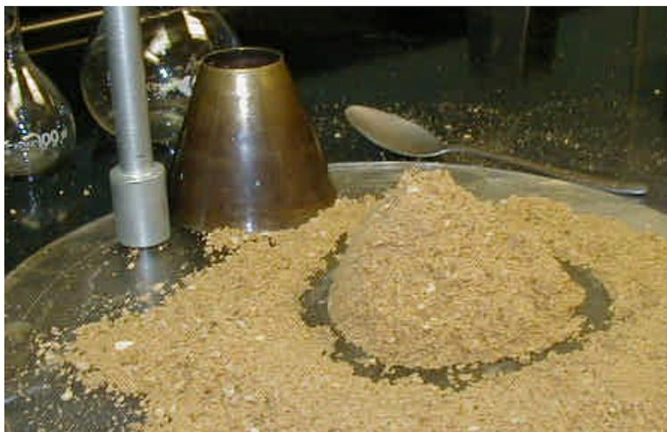
Figure 4 - Sand at SSD condition will slump once the cone is removed
