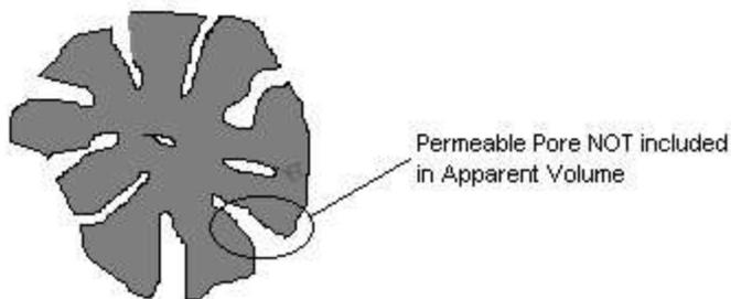
Figure 13 - Diagram of Apparent Specific Gravity Apparent Volume = volume of aggregate particle not including permeable voids.
