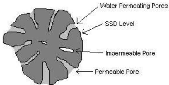
Figure 12 - Diagram of Bulk SSD. Specific Gravity SSD mass is the Saturated Surface Dry Condition and includes the mass of the water in the permeable pore space.
