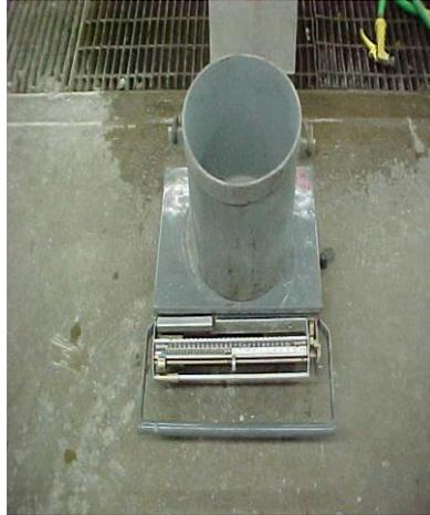
Place concrete in the measure in 3 equal layers of approximately equal volume / consolidating each layer
