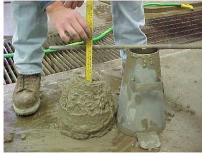
Measure to the nearest 1/4 inch the slump from the top of mold to the displaced original center of the top surface of the specimen. Perform the test within 2-1/2 minutes.
