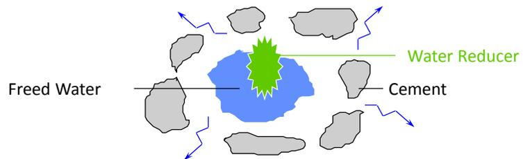
Water reducers separate flocs into individual grains. Trapped water is released and the grains slip by each other like ball bearings- improving the workability of the concrete
