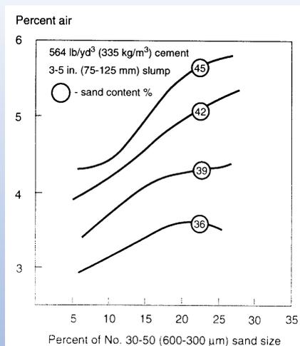
Fig. 4-1. Effect of increasing percentage of No. 30-50 (600-300 μm) material on air content. Craven, 1948. (#SK20603)
