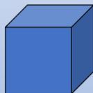
1 cubic foot block of water weighs 62.4 lb/ft<sup>3</sup>
