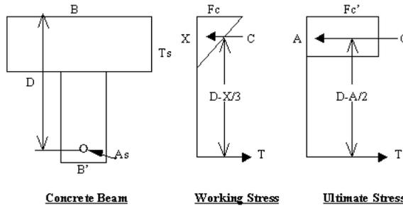
$f'_c$  = strength required to withstand live and dead loads + safety factor
