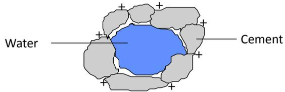
Charged Cement Particles Cling Together And Form Flocs Which Trap Water
