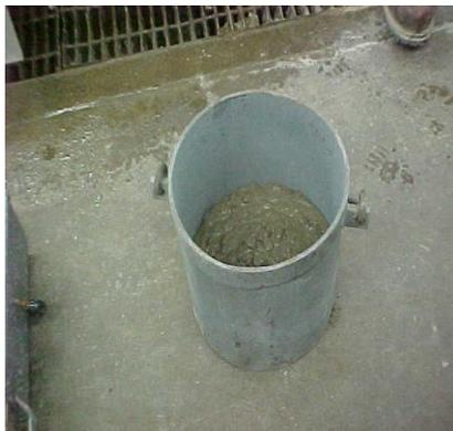
Strike off concrete level with the surface and clean off all excess concrete.
