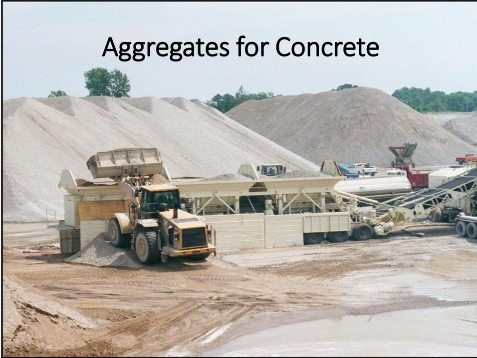
**Aggregates generally occupy 60 - 75% of the volume in a concrete mix ( 70 - 85% by weight )**
