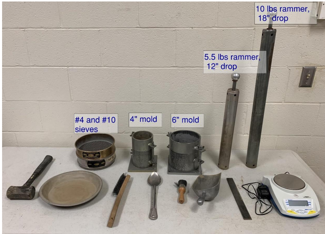
Figure 2.1 ASHTO T-99 and T-180 equipment
