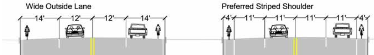
Figure 2.2 - Example of roadway retrofit to provide additional shoulder space for bicycles (3' operating space, 1' gutter)
