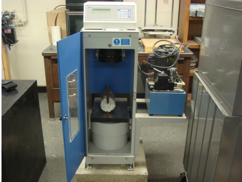
Figure 4.4: Split Tensile Strength Test with Bearing Strips Prior to Loading
